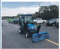
25 HP w/heated cab and front mounted snow blower!
