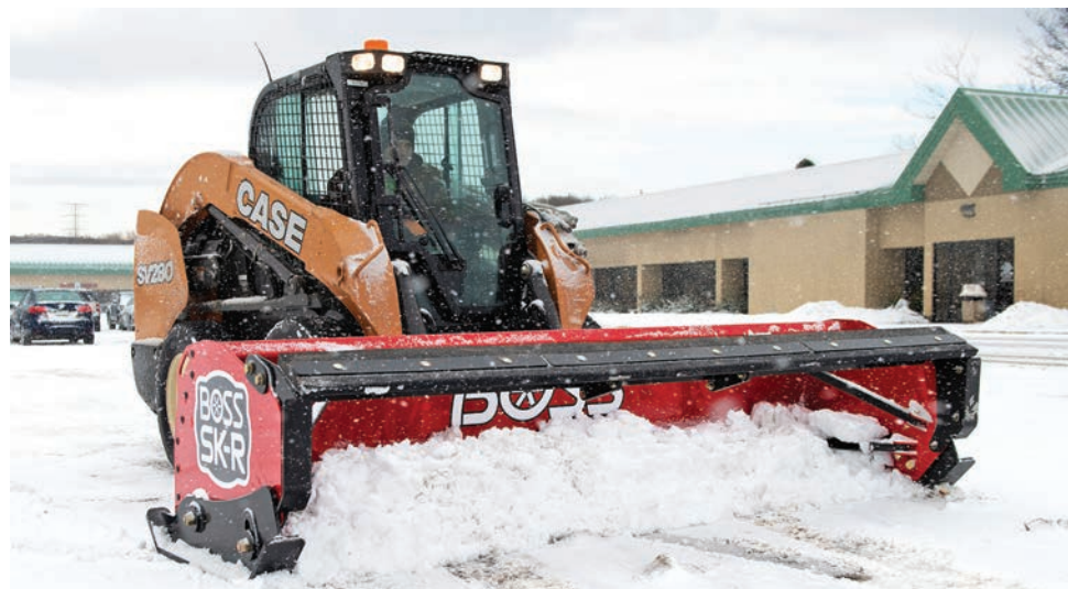
The BOSS XT is now available in 8'2" and 9'2" stainless steel models. Its flared blade wings and enhanced curl design allow users to throw snow higher and farther over existing banks than conventional plows.
