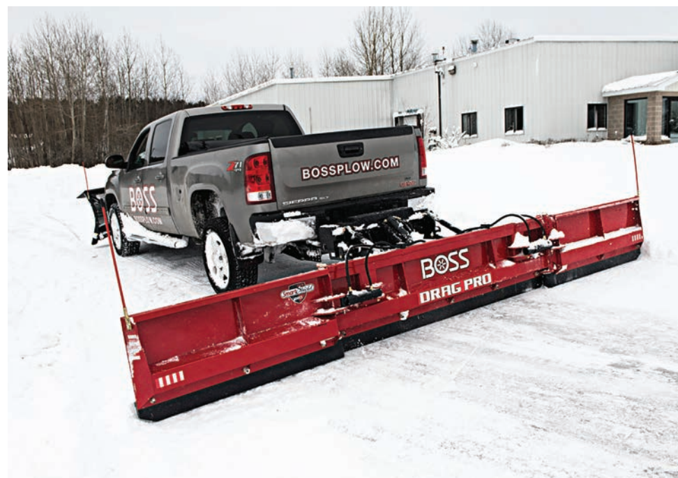
Photos courtesy of BOSS The folding wing models are easily controlled via remote in the truck's cab.
