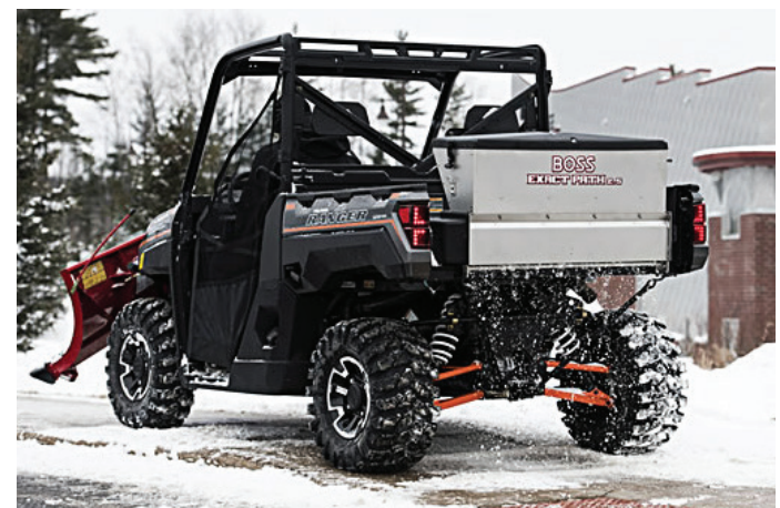
A stainless steel hopper and frame with a polyethylene cover keep materials dry and free flowing.
