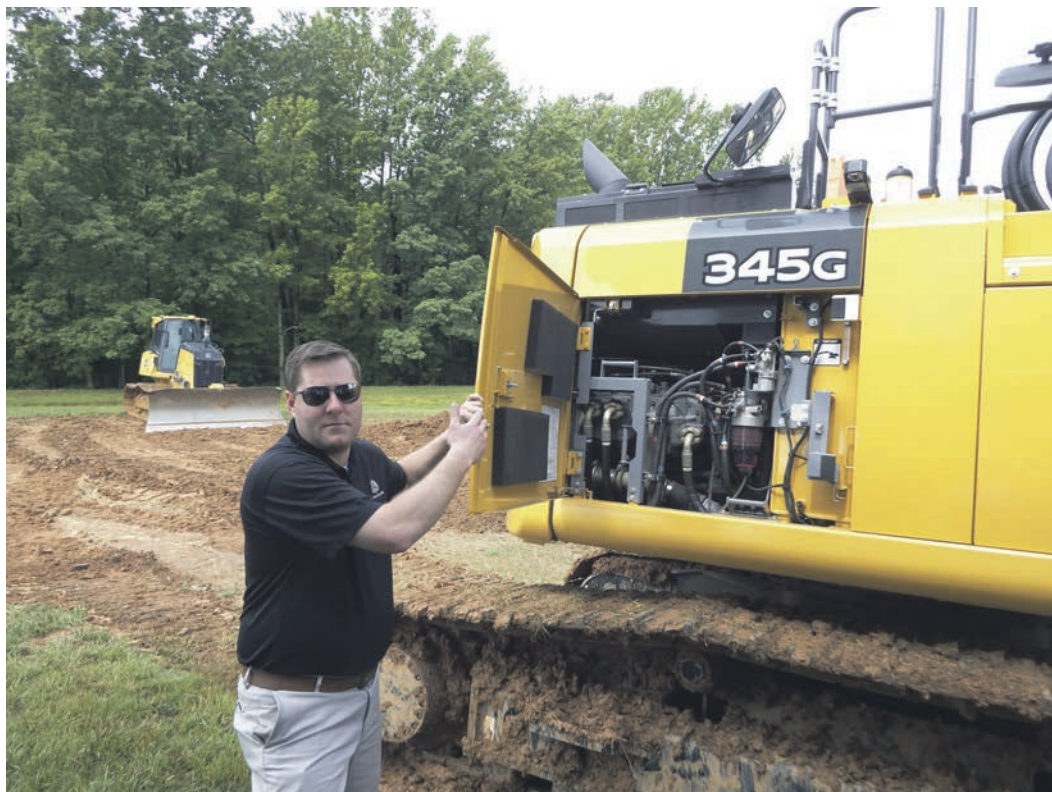
The 345C features three hydraulic pumps that provide optimum hydraulic pressure to various functions of the excavator when the demand is needed. Alex Anhalt, product consultant for excavators, explains how the systems work.
