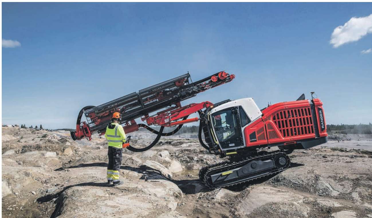
Ranger DXi rigs are extremely mobile, thanks to a low center of gravity and high tramping power.
