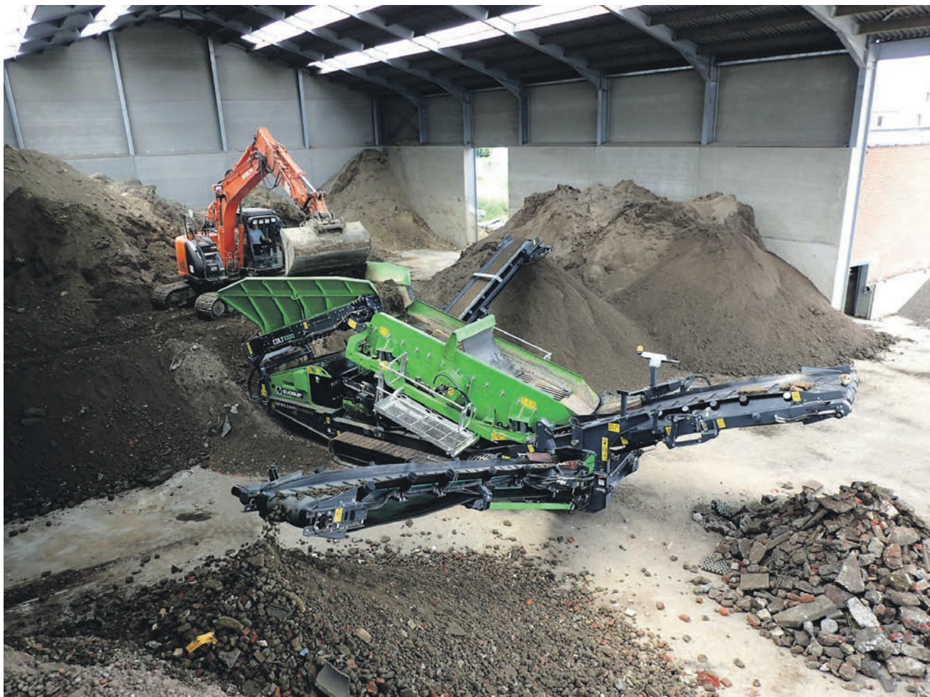
Standard configuration discharges the fines product to the right side of the plant, with the mid-grade on the left.
