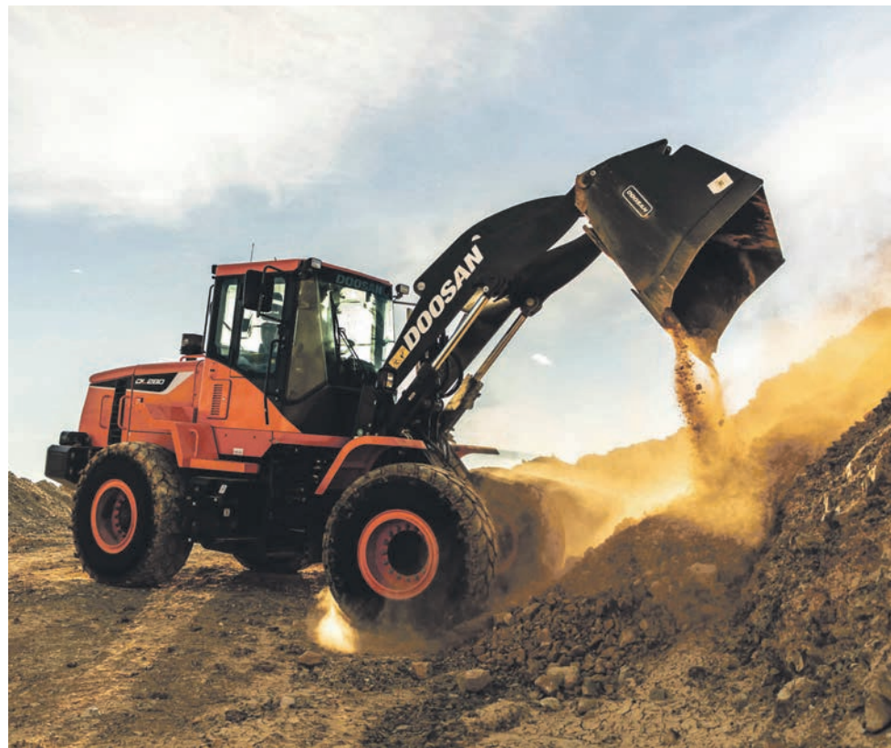
Operators requiring additional dumping capabilities into trucks and hoppers will benefit from the high-lift Z-bar configuration available on the DL280-5.
