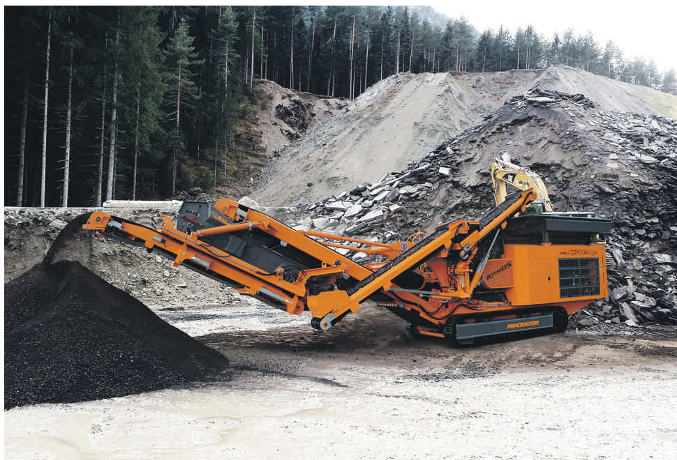
Rockster R1100DS Impact Crusher: Recycling of RAP for reuse as adjunct for new asphalt.
