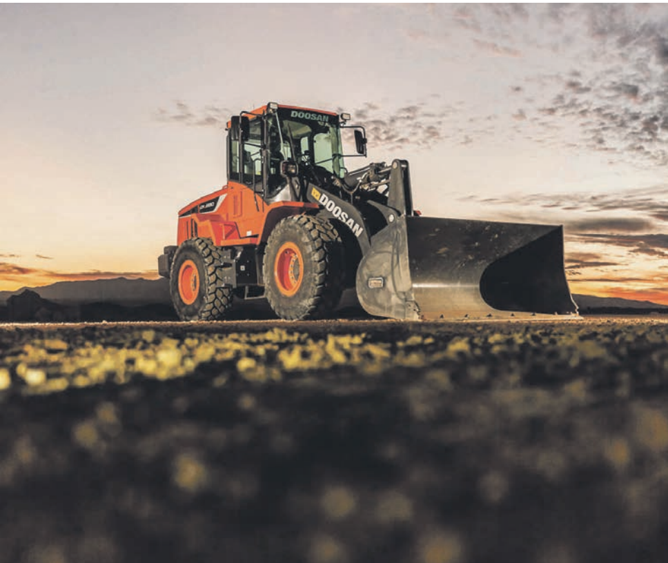
The DL280-5 has an optional quick coupler to easily change attachments, including buckets (general purpose, light material or multi-purpose) and pallet forks.
