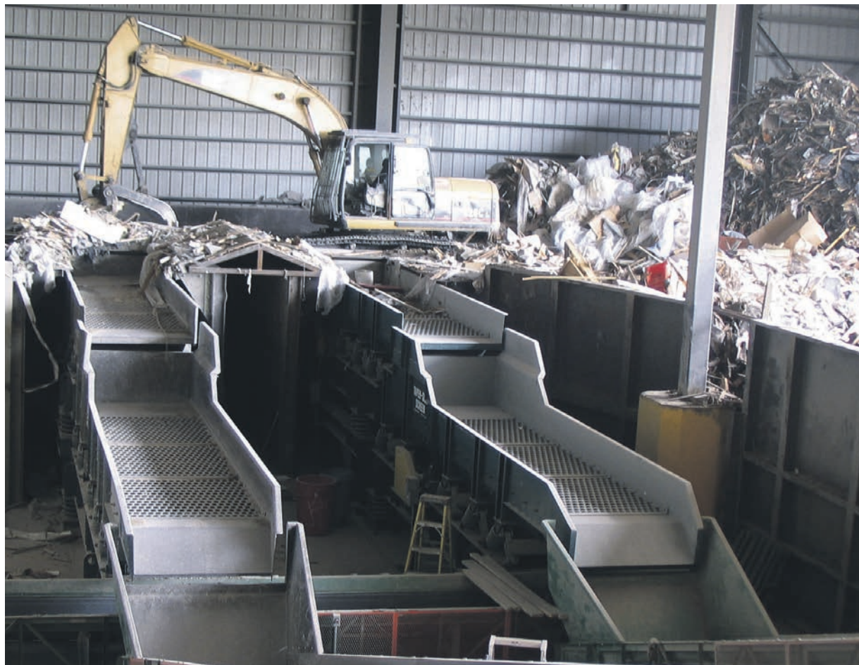
An excavator feeds the C&D material onto the Action TAPER SLOT screen to remove material and particles that are smaller than three inches.
