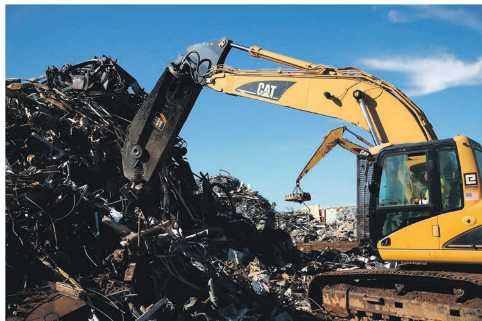
Tapered spacer plates reduce the drag of material being cut, a design feature that both reduces the amount of energy required from the shear and speeds cutting.
