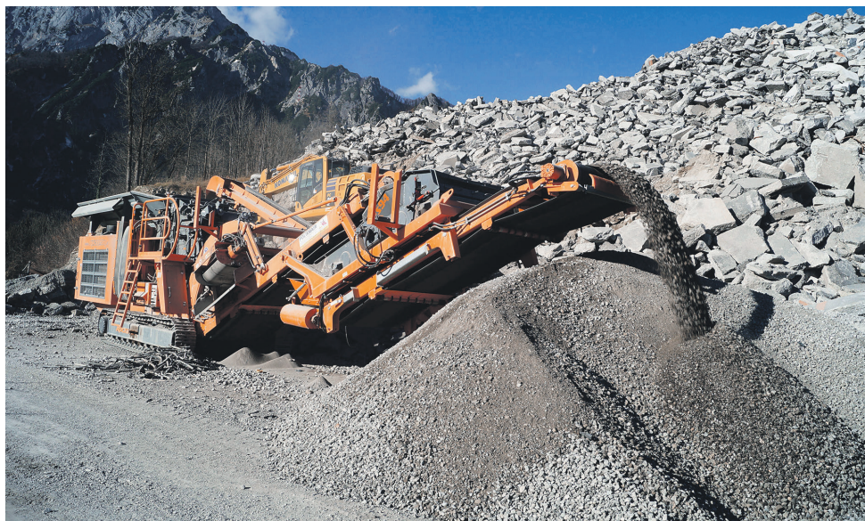
Rockster Impact Crusher R1100D: Recycling of 100,000 tons of highway concrete which is reused for stabilization and fillings in road construction.
