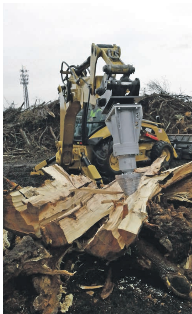
The Black Splitter Model SB Hydraulic Cone Splitter helped The Shelter Island Recycling Center on Long Island, N.Y. to preserve its new horizontal grinder by downsizing vegetative waste before processing.
