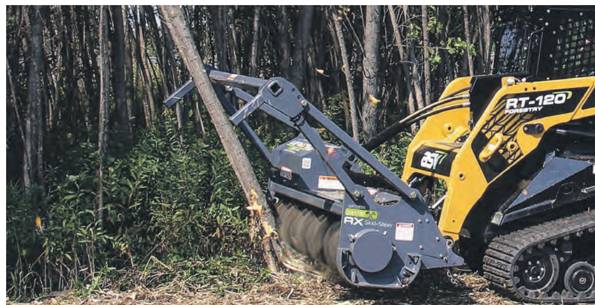
Featuring a new rotor, tooth design and exclusive two-stage cutting chamber, the heavy-duty Battle Ax is designed for highly efficient vegetation management.
