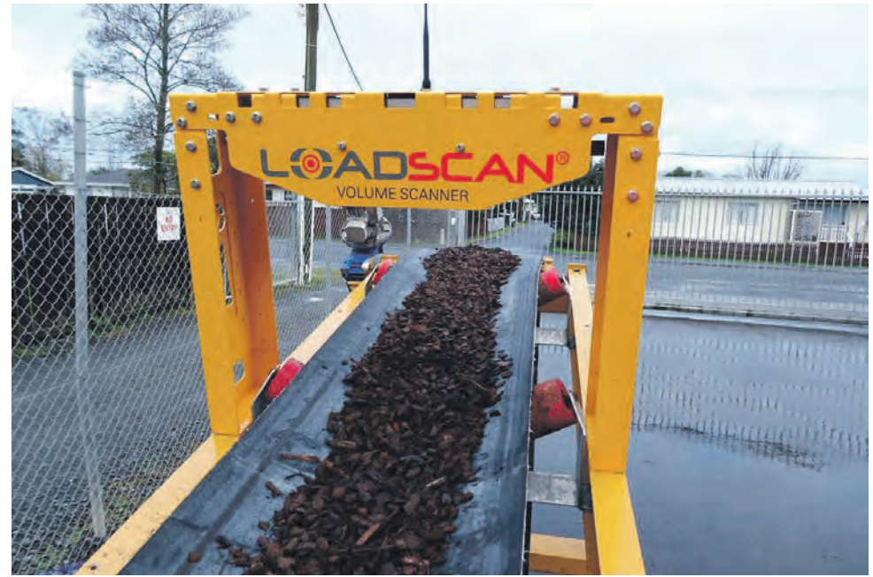
With this system you'll measure actual volume, not a converted weight estimate while also recording a 3D color profile of every load.
