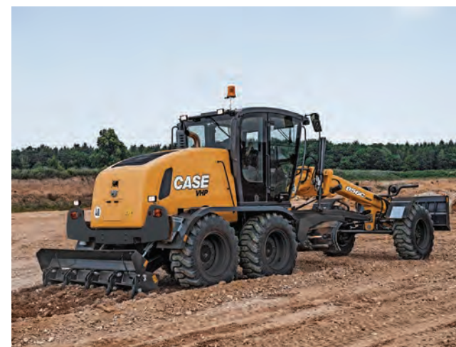
All maintenance checkpoints are located at ground or fender level — making service and daily maintenance as straightforward as possible.
