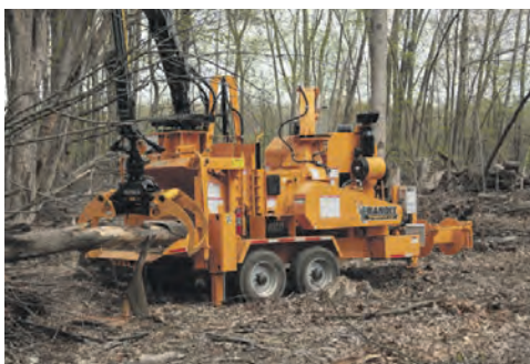
Using intuitive controls, the operator can guide the material quickly into the chipper to be processed in a fraction of the time it would take operators to winch.
