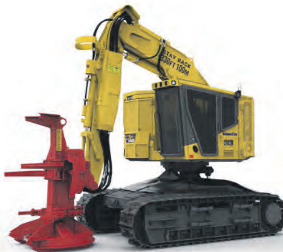
The state-of-the-art, fully certified Komatsu forestry cab has been relocated to the left of the boom for industry commonality.
