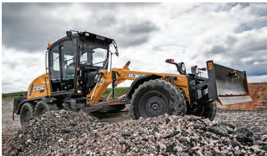
A low-profile rear-mounted cab with wide tinted floor-to-ceiling windows and external mirrors offers superior visibility of the moldboard and surrounding area.
