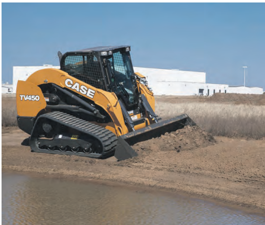
The newest and largest CASE CTL ever built features an industry leading 9,188 pounds of breakout force.
