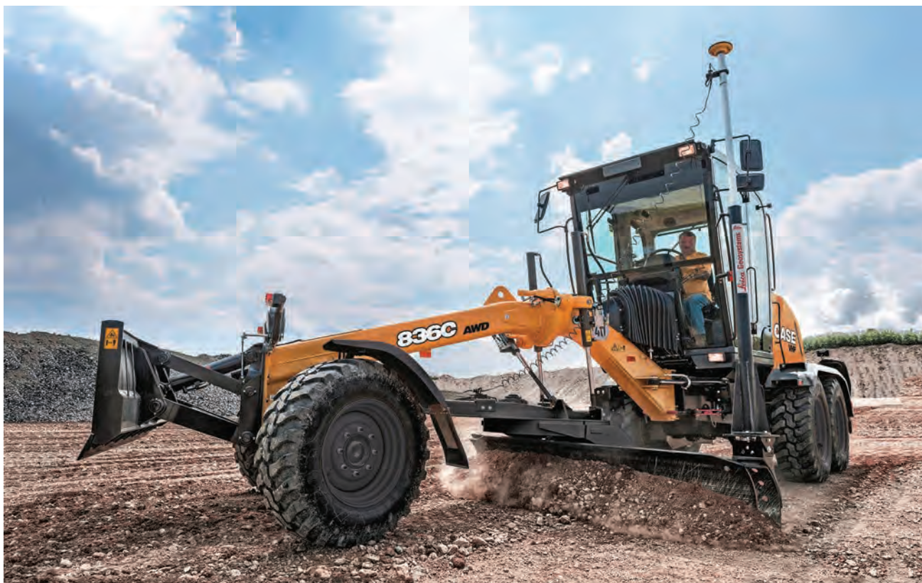
CASE C Series motor graders feature a high-carbon steel moldboard and a new moldboard mount and slide system.
