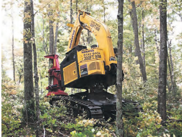
Boom, arm and rear hydraulic tubes and hoses have robust forestry-specific guarding that improve protection and shed debris.
