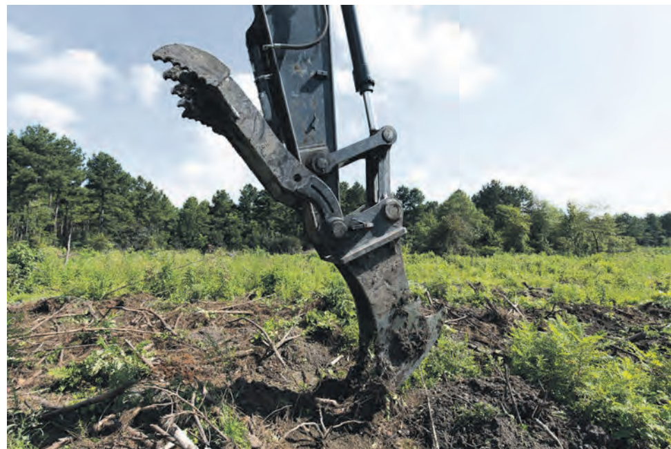
The Stumper also features claws on the back of each shank to push stumps away from the excavator.
