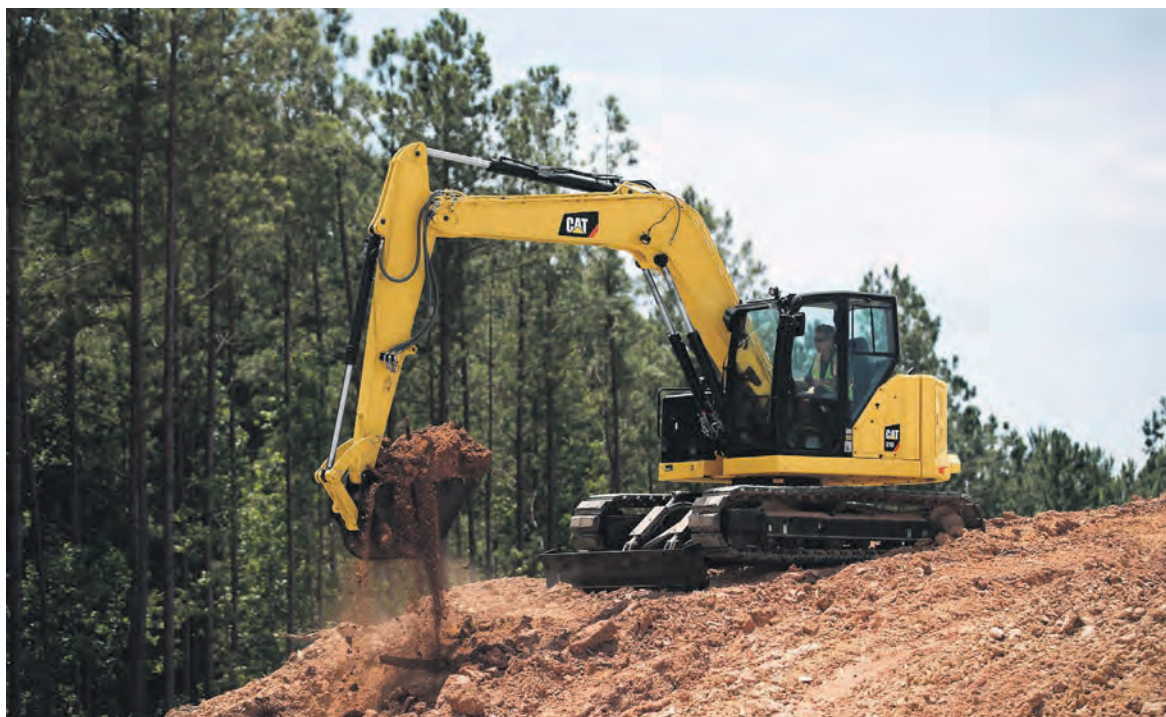
For added versatility, the standard auxiliary hydraulic system (complete with quick-disconnect lines) provides one-way, two-way and continuous flow.
