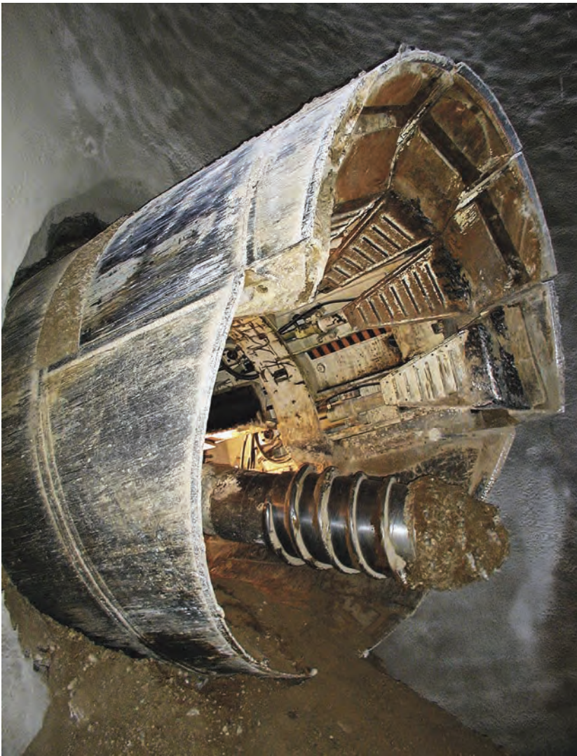
Herrenknecht AG's partial-face excavation machines are able to excavate any soil encountered through the use of two different cutting tools.
