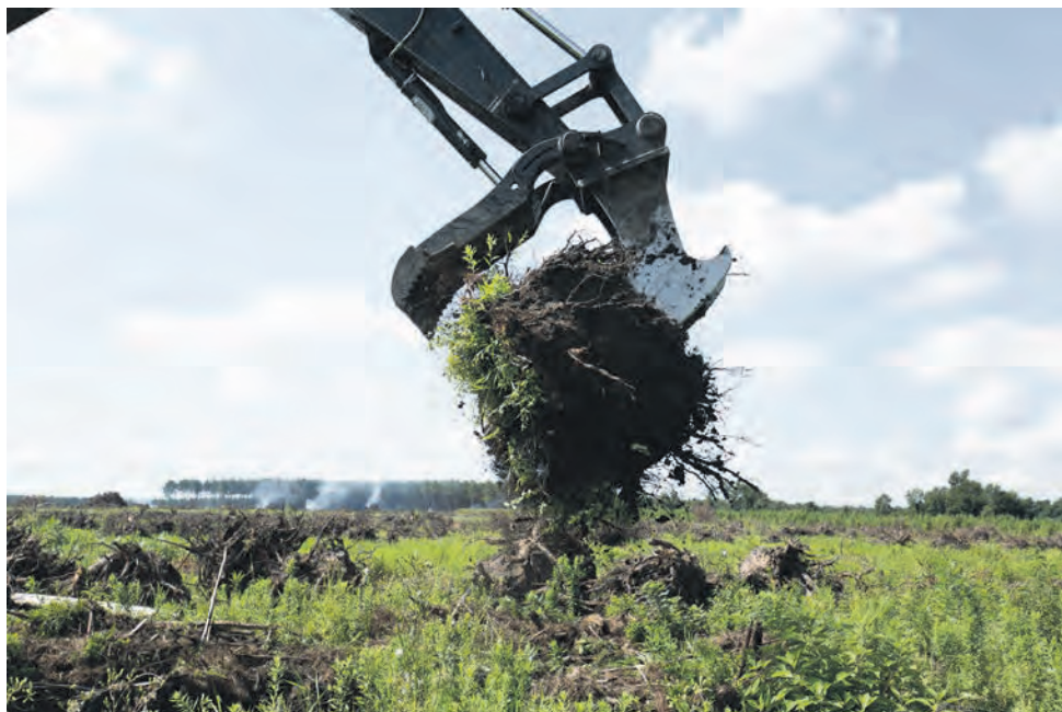
The attachment's two shanks easily cut through roots so operators can remove stumps without displacing a large amount of soil.
