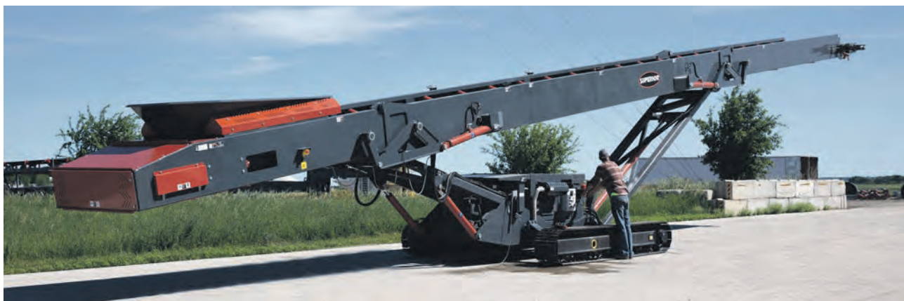
The hopper’s drive and backstop are hydraulically controlled in addition to the discharge conveyor’s fold and raise features. Photos courtesy of Superior
