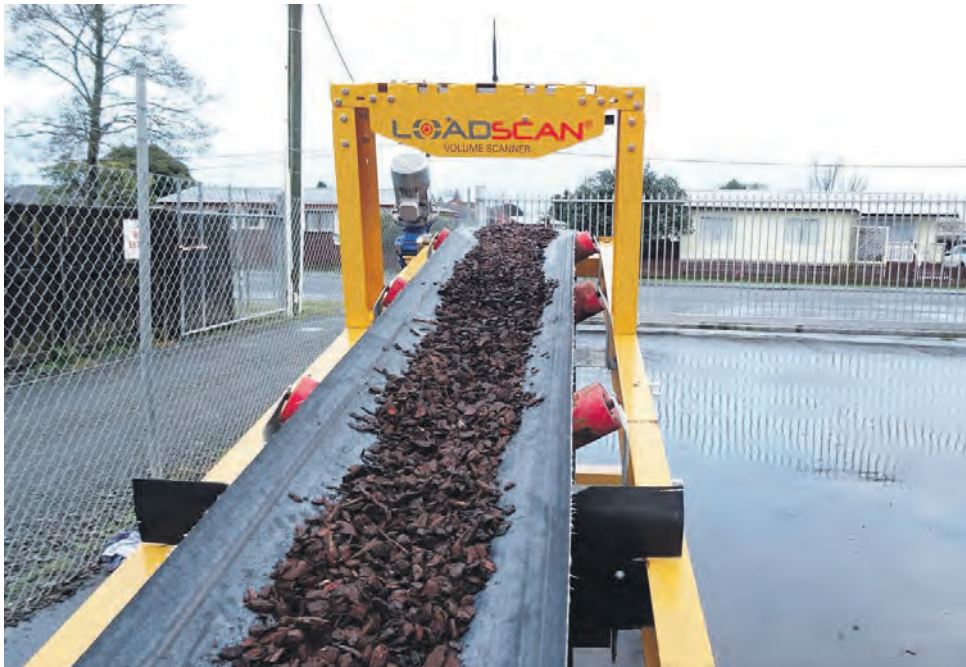
The CVS is an above-belt lidar laser measurement system making it perfect for production management.
