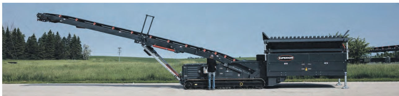
The tracked stacker will be one of the heaviest models available in its class at 34,000 pounds.
