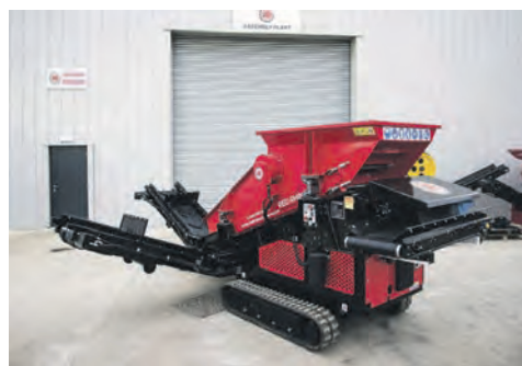
Red Rhino's latest development is a highly compact 3-way split screener.
