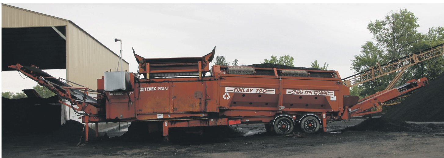
The Terex Finlay 790 Single Skin Trommel with ¼-inch trommel screen used to further size already-ground asphalt shingles (RAS) for use in new asphalt mix at Senn Blacktop.
