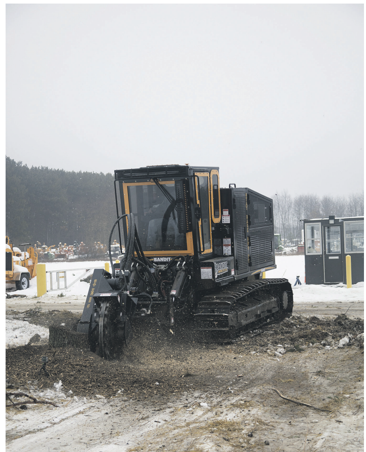
When Bandit Industries needs to remove trees to make room for the expansion, they've got plenty of equipment on hand to deal with the stumps like this BTC-300 track carrier with its detachable stump grinder head. This machine made quick work of the dozen stumps standing in the way of the building construction.
