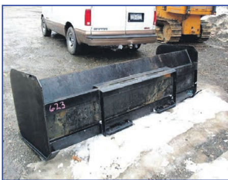
Wildkat SAB 96 8' Snowpusher for Skidsteer, Adjustable Steel Cutting Edge, Universal Skid Steer Coupler, New ..... $1,950
