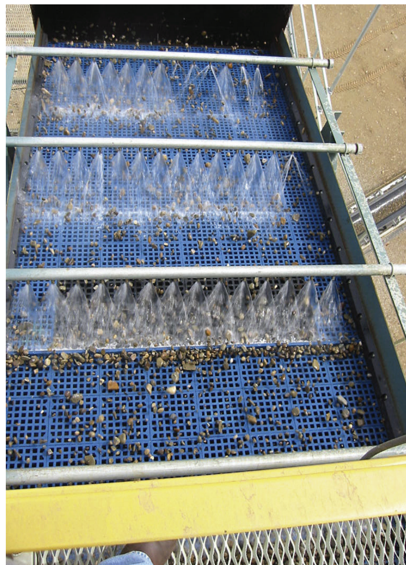
Good overlapping spray with adequate PSI and surface dams can help increase quality, efficiency, and capacity.
