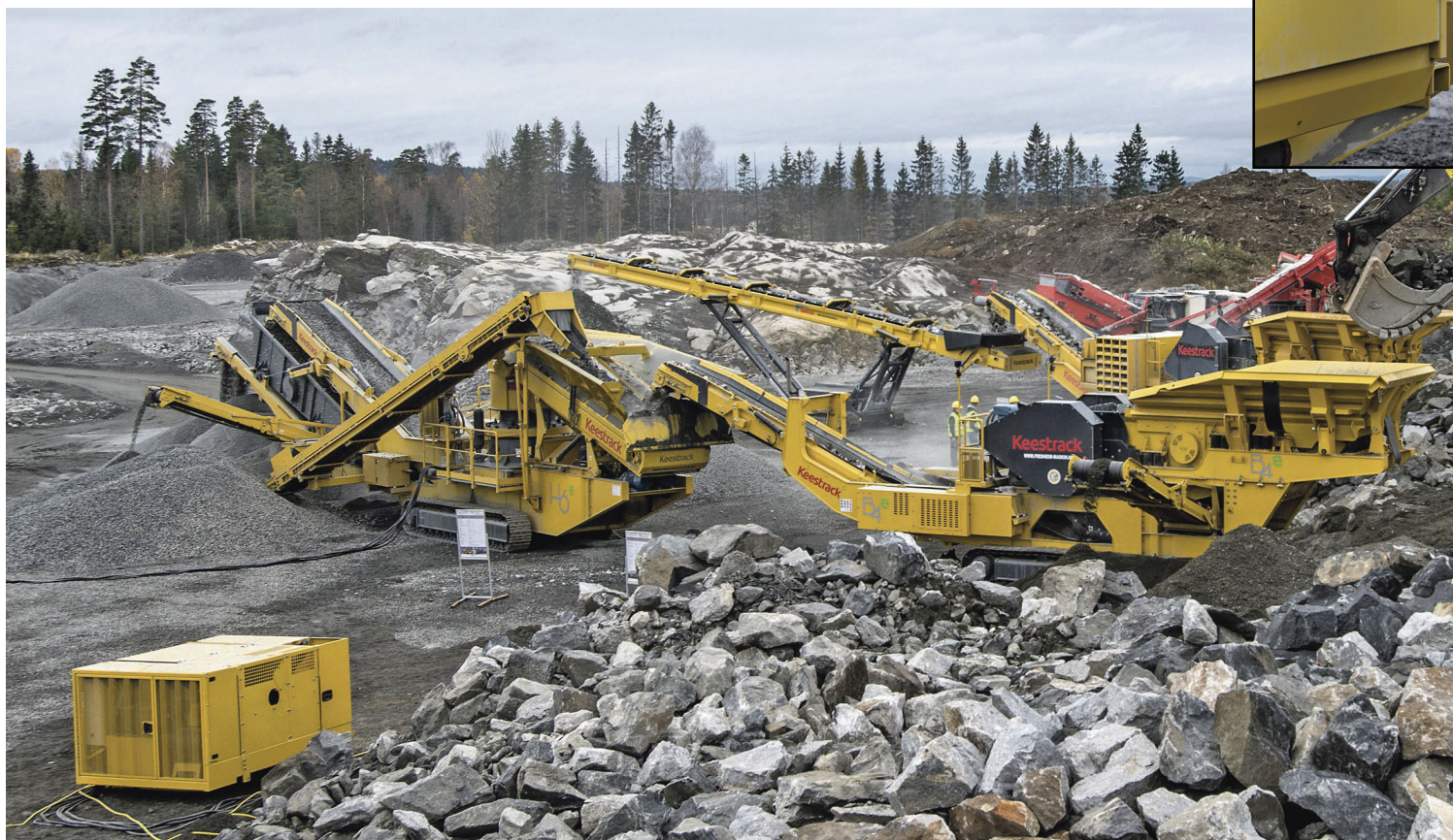
The detachable motor/generator module of the Keestrack H6e crusher (in the background) guarantees a lower load on the drive through dust and vibrations. This solution is now also available as an option for the Keestrack B4e large jaw crusher (right).
