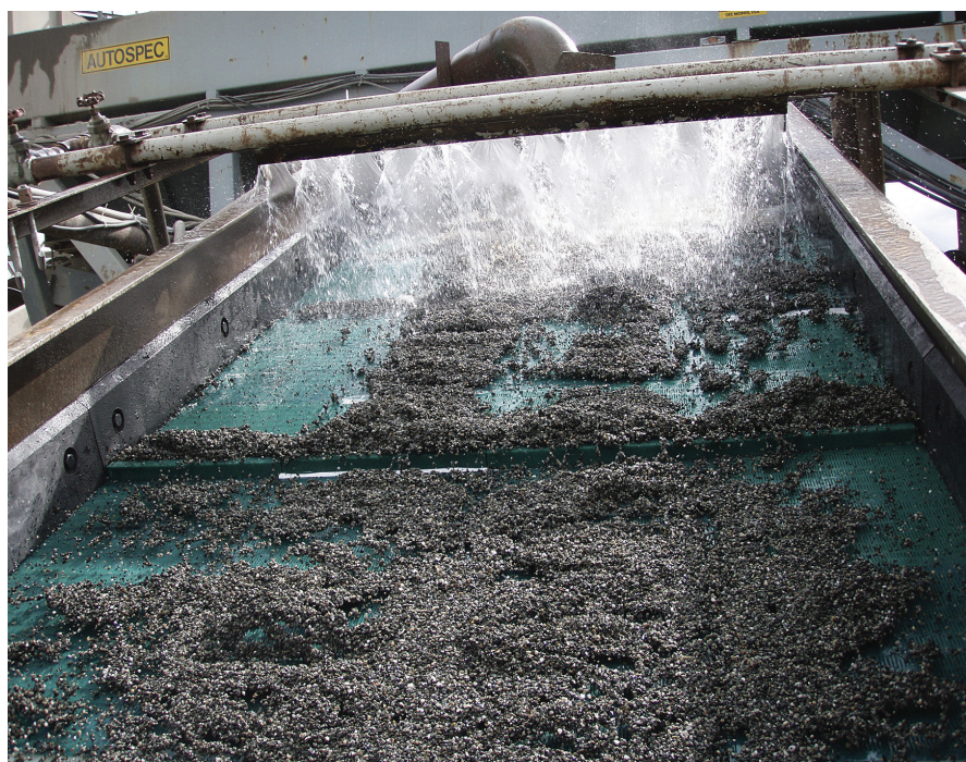
Panels with dams built into the surface are a great way to add retention time if the "water dam" from your spray bars isn't enough. The increased travel rate of inclined screens would make this a good application to incorporate dam panels.
