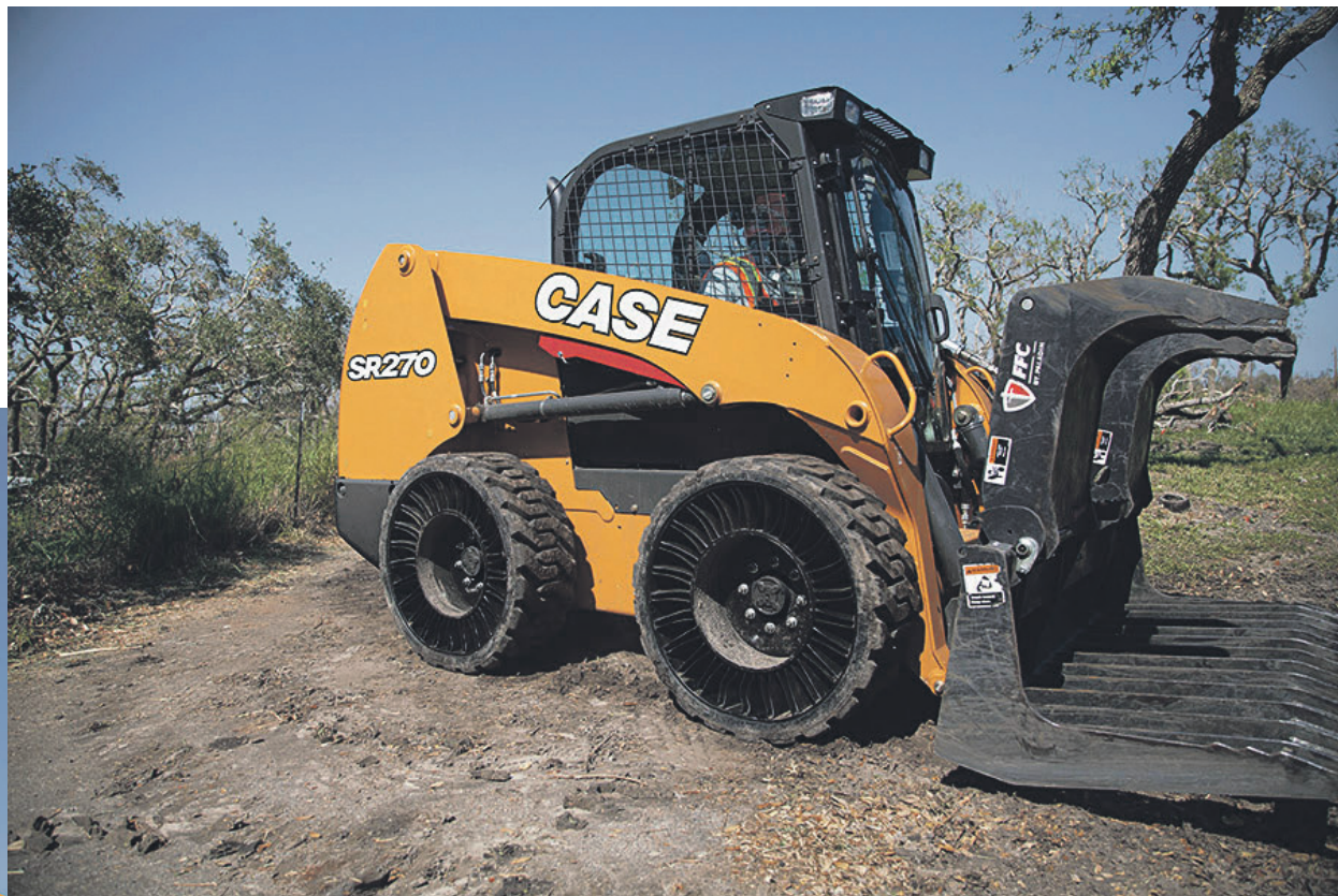
The Michelin X Tweel SSL provides outstanding stability and enables a skid steer loader to work rapidly with more comfort for the operator, reducing driver fatigue while improving productivity.
