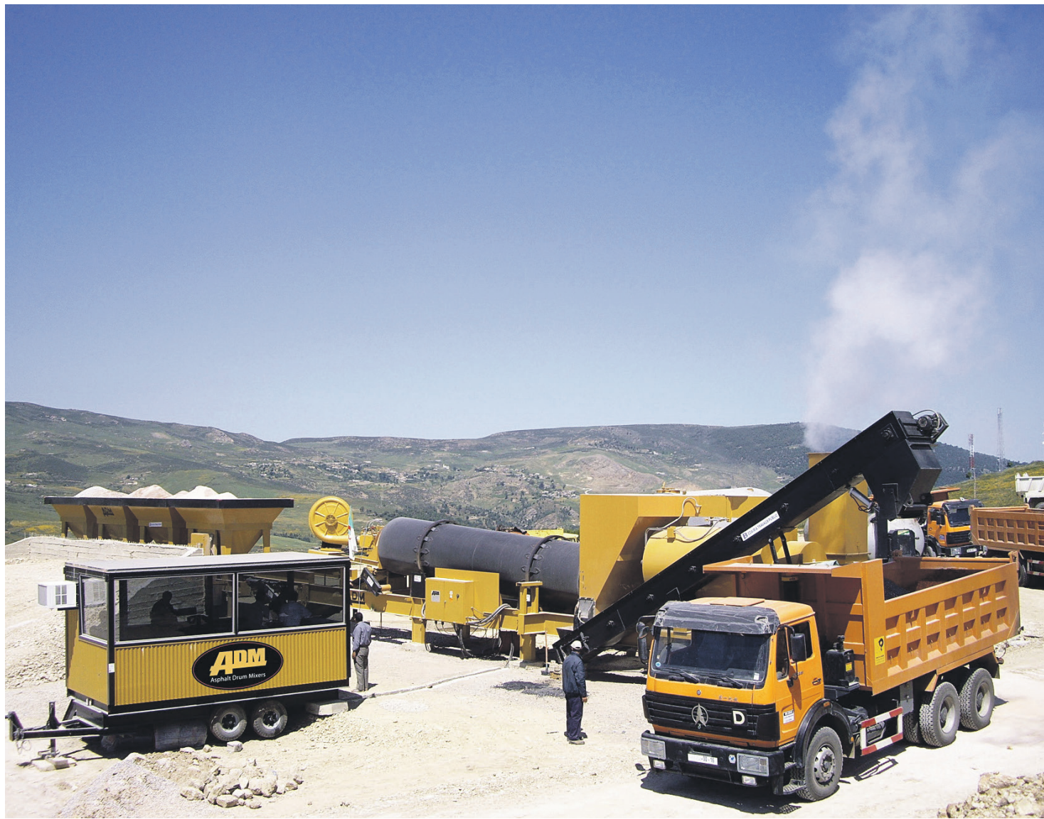
The SPL series includes all necessary components for drum-mixing asphalt production yet fits on a single trailer frame.
