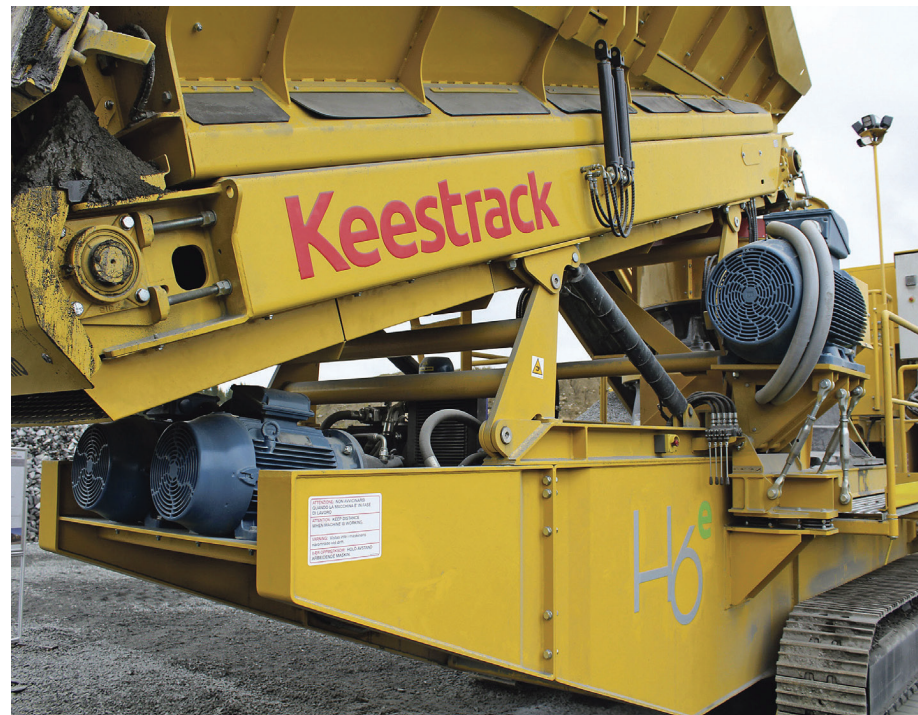
The 220 kW electric motor of the crusher drive (right) and the two 30 kW generators of the load-sensing operating hydraulics, which are mounted in a protected manner beneath the feeder, enable all-electric operations.
