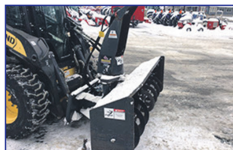
Erskine ES2000 Snowblower Skid Steer Mount Blower, Standard Flow, 7' Working Width, Hyd. Spout Rotation, Hyd. Deflector..... $4,000
