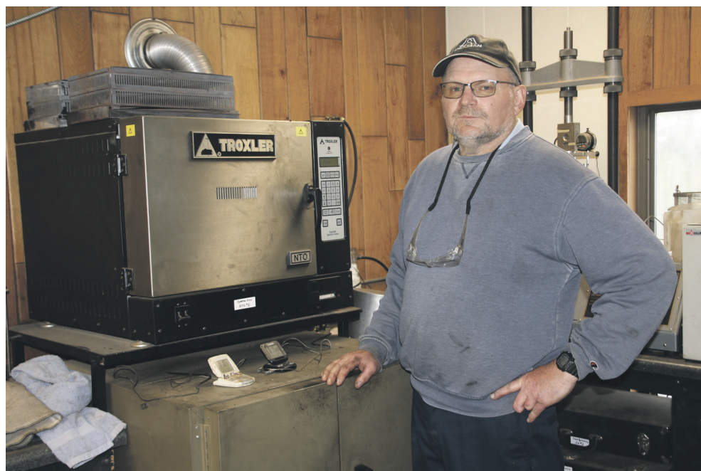
Jeff Novak, Quality Control Manager, with the Troxler Oven NTO in Senn's Company lab, where he develops and tests new HMA mixes to meet WisDOT specs.
