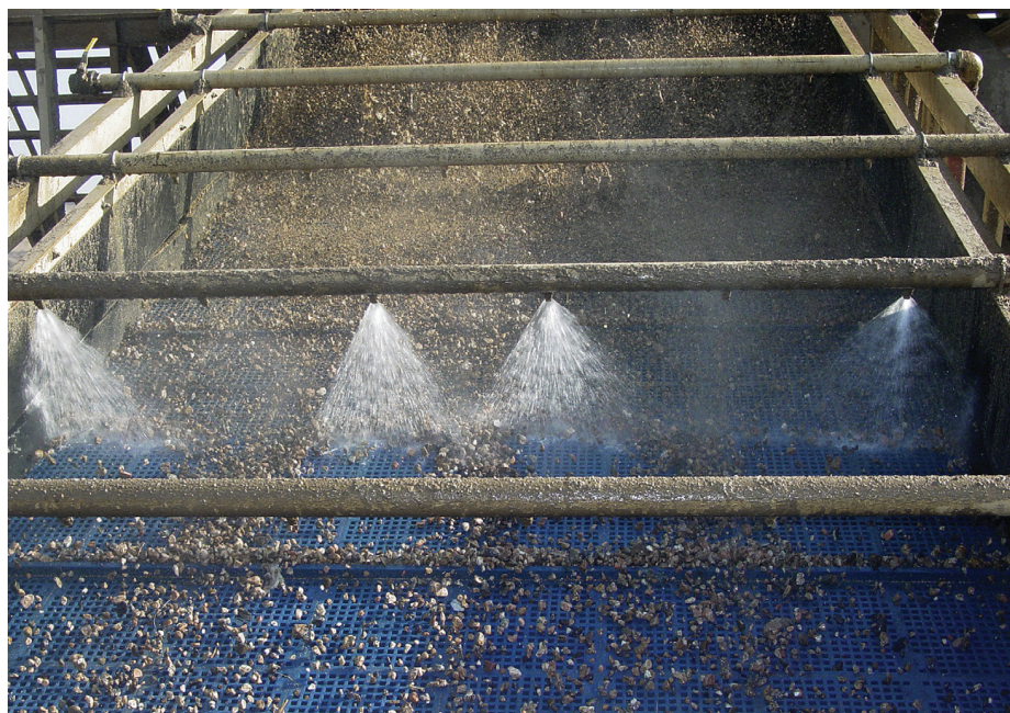
Plugged spray bars/nozzles could be a bottleneck to increased screening capacity and/or improving the quality of your product. Using a non-corrosive spray bar with self-cleaning nozzles can help minimize this issue.
