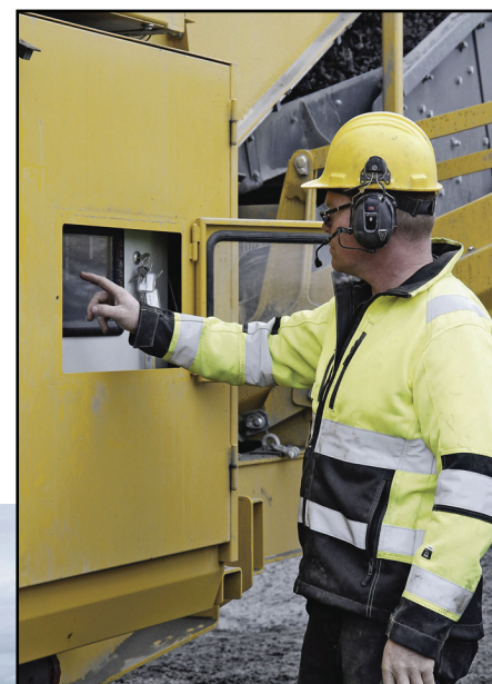
Above: All system functions, including the Hydroset crusher settings, can be operated comfortably and safely via the central Relytec panel of the Keestrack PLC controller.
