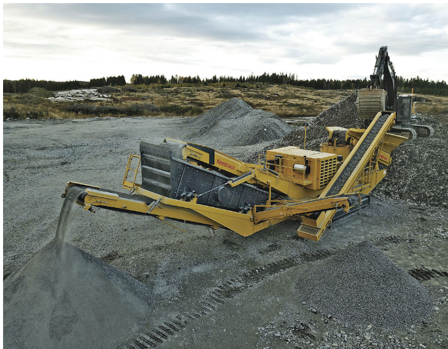
With a max feed size of 215 mm, the Keestrack H6e track-mounted cone crusher can also be deployed as a highly productive stand-alone solution when equipped with the three-deck post-screen module.
