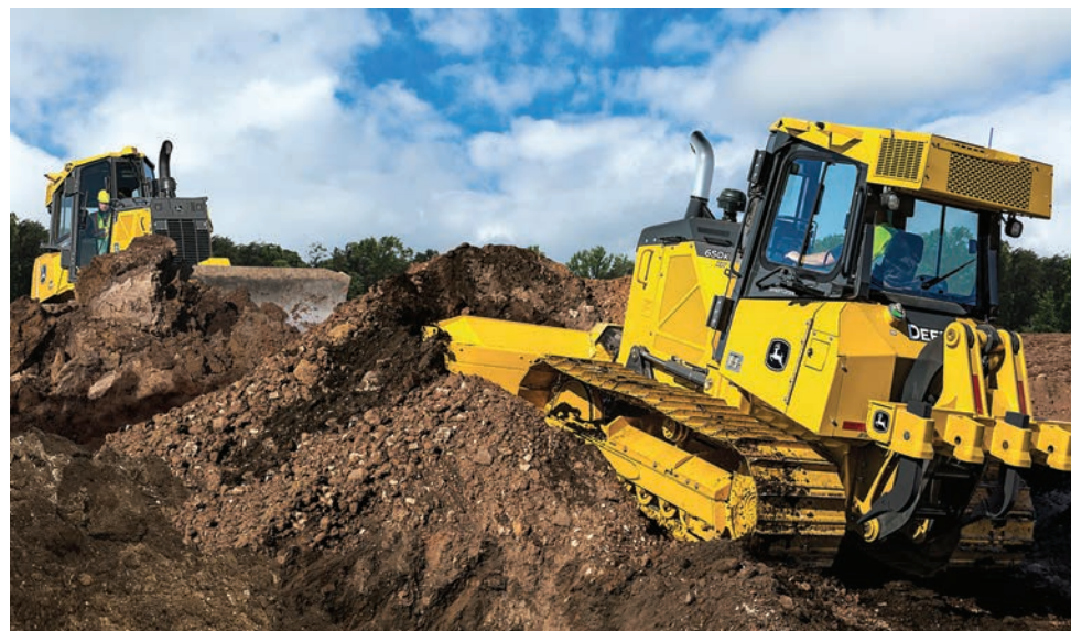
Since SmartGrade is integrated into the machines, it removes the need to install blade-mounted sensors and components daily, reducing setup time and allowing operators to get to work.
