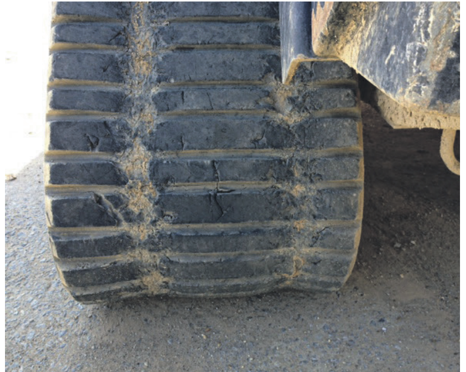
The average rubber track life is about 2,000 hours but can be as high as 5,000 hours with proper maintenance. Neglecting rubber track maintenance, however, can result in a wear life as low as 500 hours. The tread in this track is gone so it is at the end of its serviceable life.
