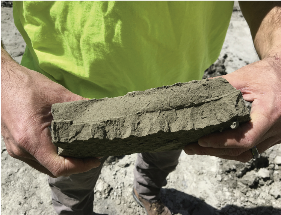
When all of the water has been expelled from the mud, the press opens discharging dry mud cakes.
