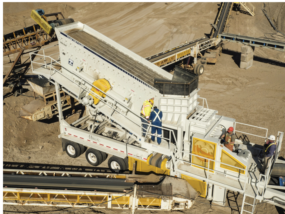
Haver & Boecker’s portable F-class increases operational flexibility by allowing operators to move it quickly between jobsites.
