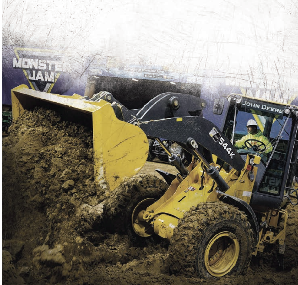
Having the right equipment is critical. The John Deere 544K loader is a prime mover that's used to spot dirt and knock down piles. Photos courtesy of John Deere
