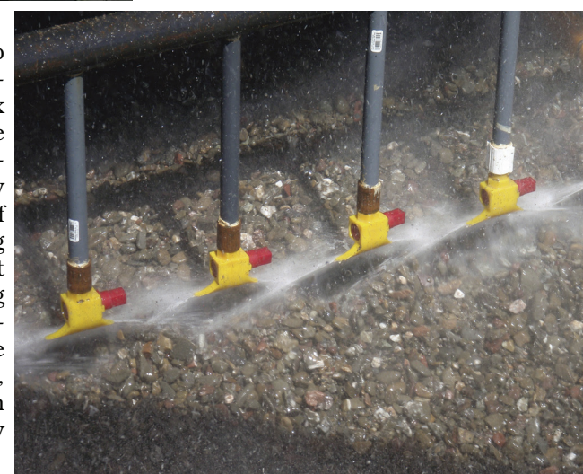
Overlapping spray coverage and self-cleaning nozzles help minimize maintenance requirements.
