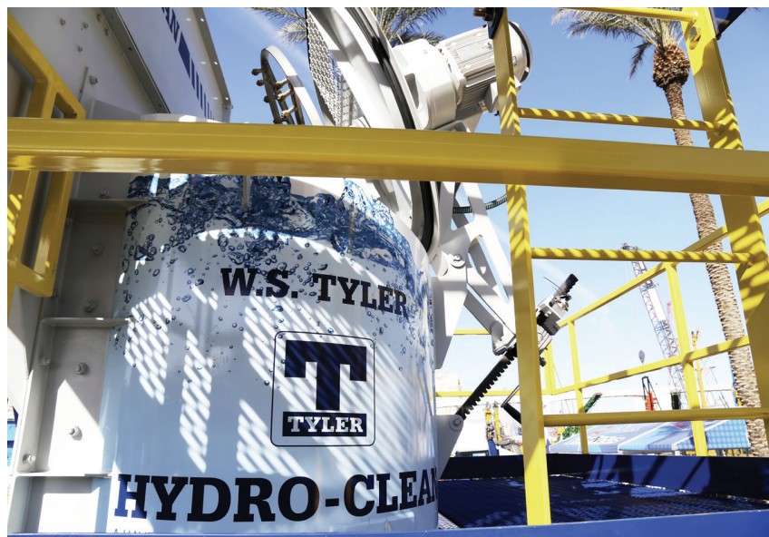
The Hydro-Clean’s high-pressure nozzles effectively clean deleterious material from aggregates, recycled materials and other minerals.
