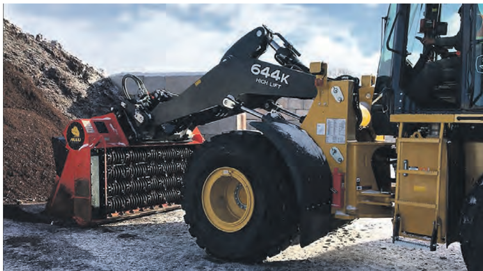
Transformer has also proven to be beneficial in pulverizing frozen piles of mulch that the facility stores outside.
