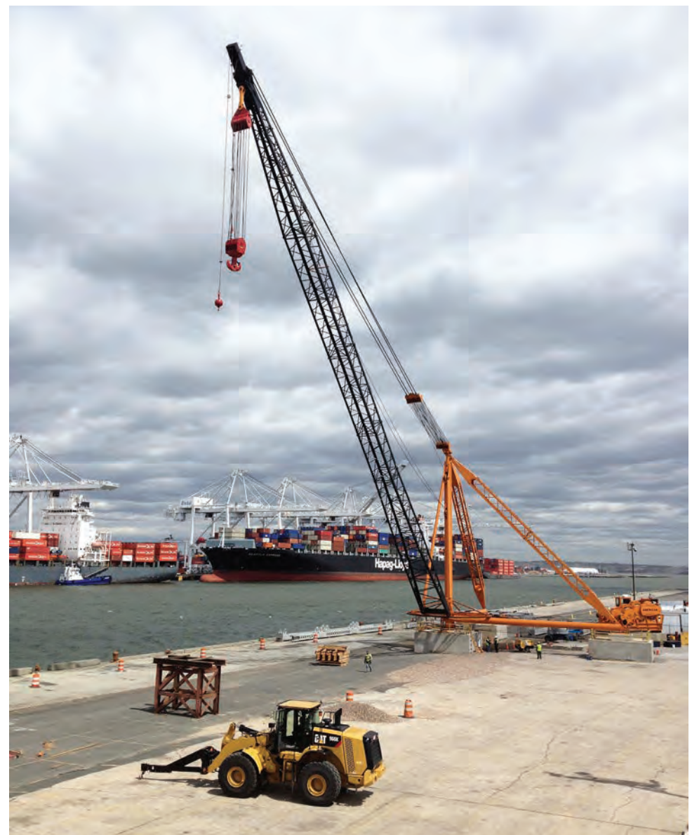
The American Cranes S-60 stiffleg derrick is an ideal choice for dockside operations thanks to its high lifting capacity and stability.
