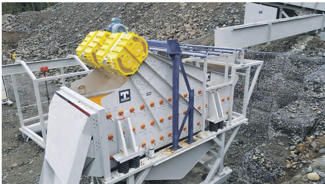
Haver & Boecker offers new configurations of its Ty-Rail quick-tensioning system. Ty-Rail dramatically cuts the time needed to replace screen media in half. The patented tension rails release as a single piece.
