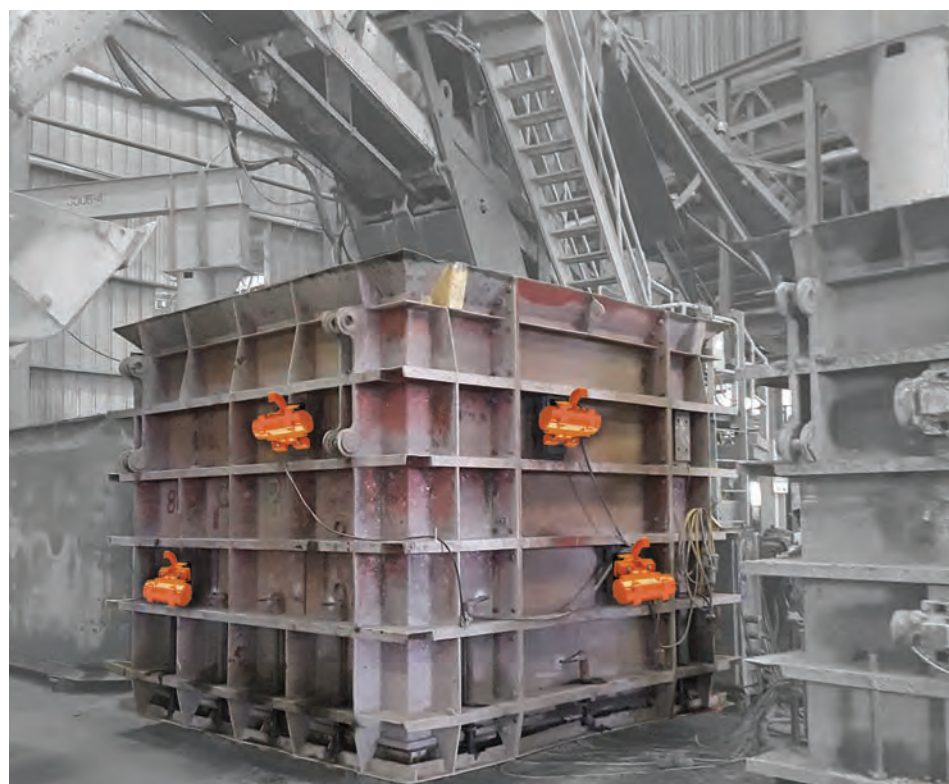
Using standard mounting brackets, operators with several vibrators affixed to a form have found the U1-1600 easily replaces heavier units and offers a longer equipment life with less cumulative weight.
