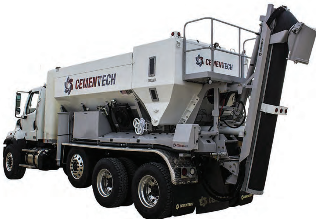
The new Automated Gates technology makes the C60 fully computerized and continues to reduce operator error by syncing the mix design with the appropriate gate setting for material flow.
