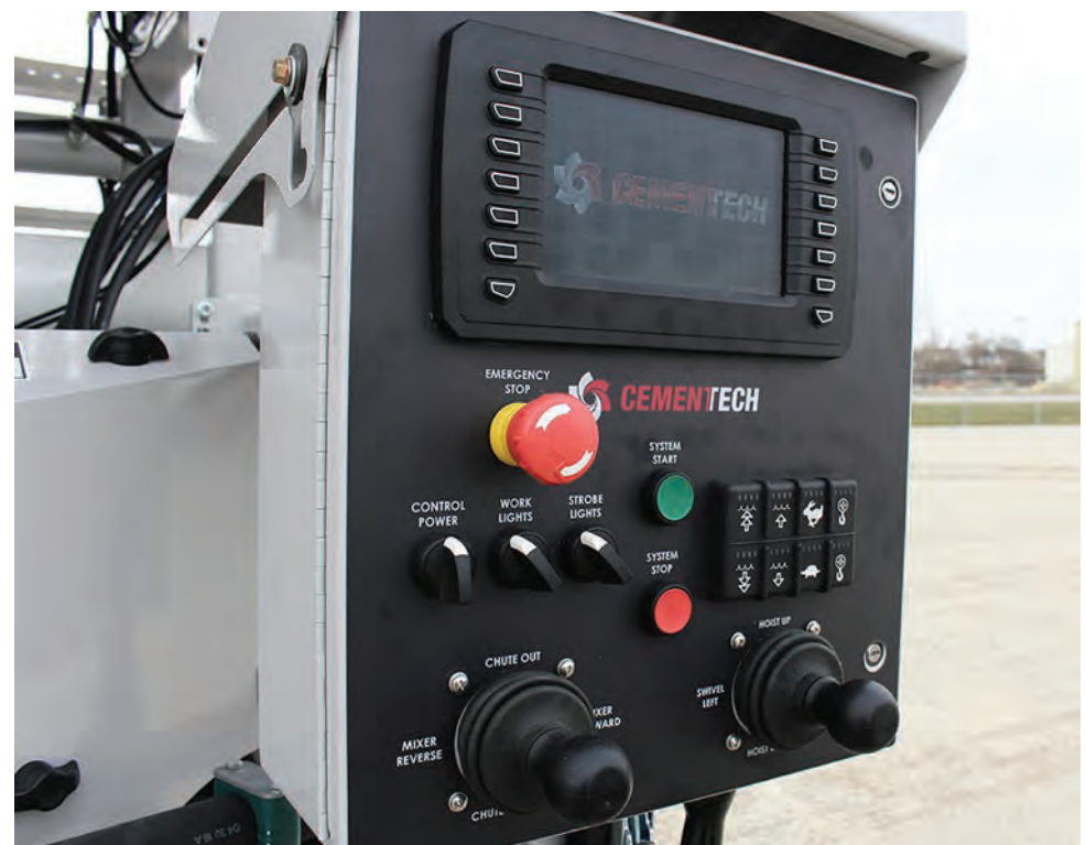
ACCU-POUR is the nerve center for the C Series volumetric concrete mixer with one-button operation using the AP-Touch™ control panel.
