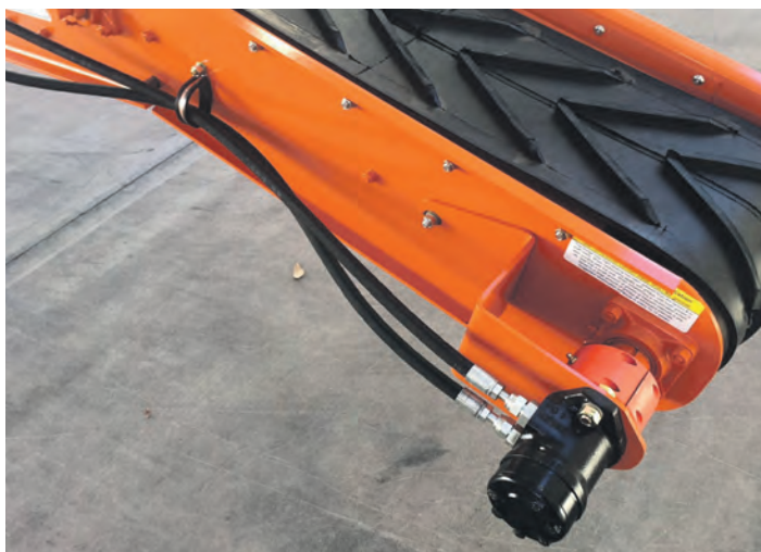
Newly constructed conveyor using a hydraulic motor as a form of a gearing package substitute.
