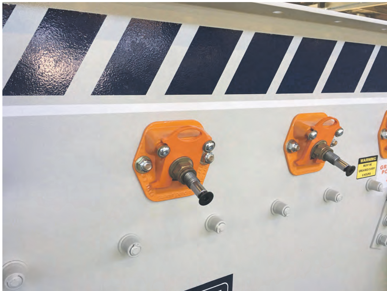
Haver & Boecker developed and now offers three angle-box designs for different vibrating screen setups. This allows producers to benefit from Ty-Rail's time savings during screen media change-outs, even on difficult-to-access areas of a vibrating screen.
