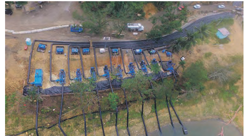
Thompson's aerial view of setup pumping 10 18" dry-prime Thompson Pumps.
