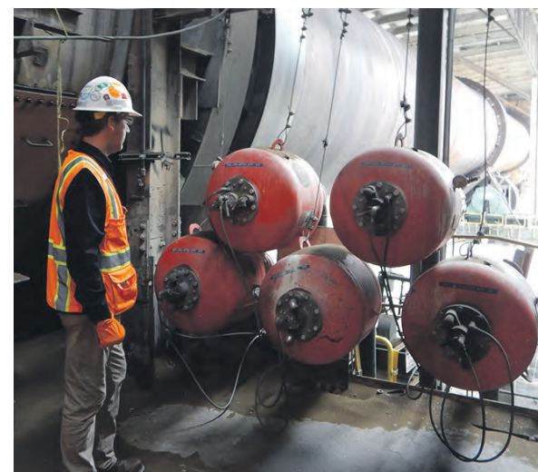
Valves face outward for convenient maintenance, requiring no tank removal to service them.
