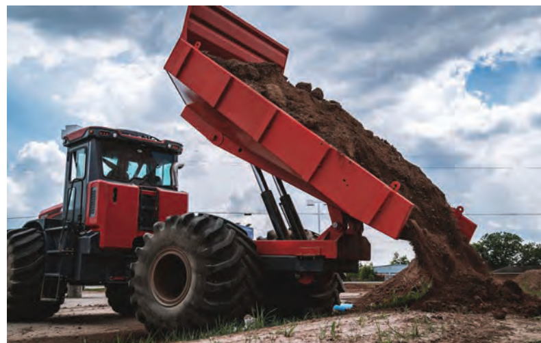
Both models have a 70-degree dump angle at full dump height, with an efficient raise time of 12.5 seconds and lower time of 13.2 seconds.
