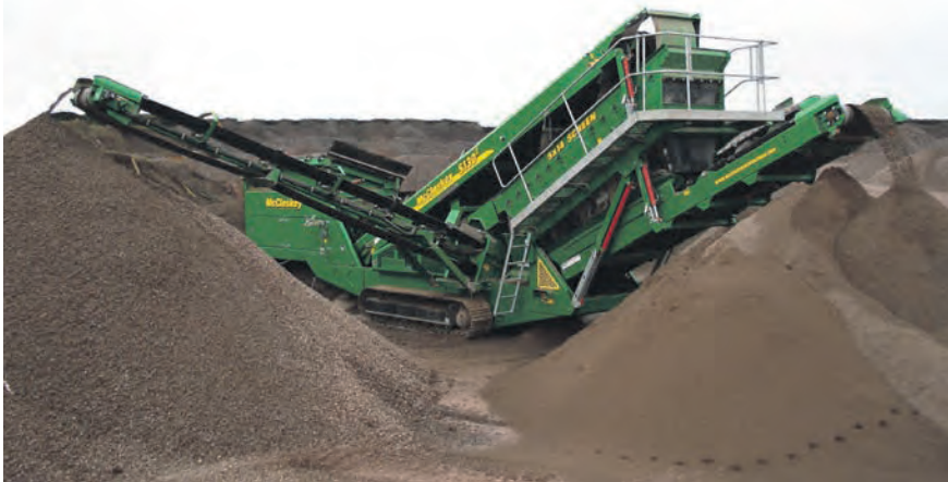
The high-energy 14x5 (4200x1524mm) screenbox of the S130 provides comparable product capacity with other larger class competitor's models.
