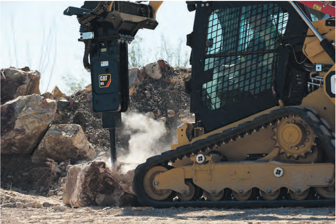
The new hammers are suited for skid steer loaders, multi-terrain loaders, compact track loaders, mini hydraulic excavators (3- to 8-ton operating weights) and backhoe loaders.
