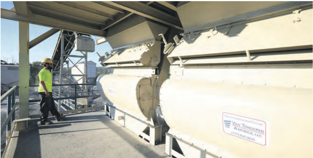
The GIC system is designed with no moving parts for dependable service and nearly zero maintenance in unattended, 24/7 operation.
