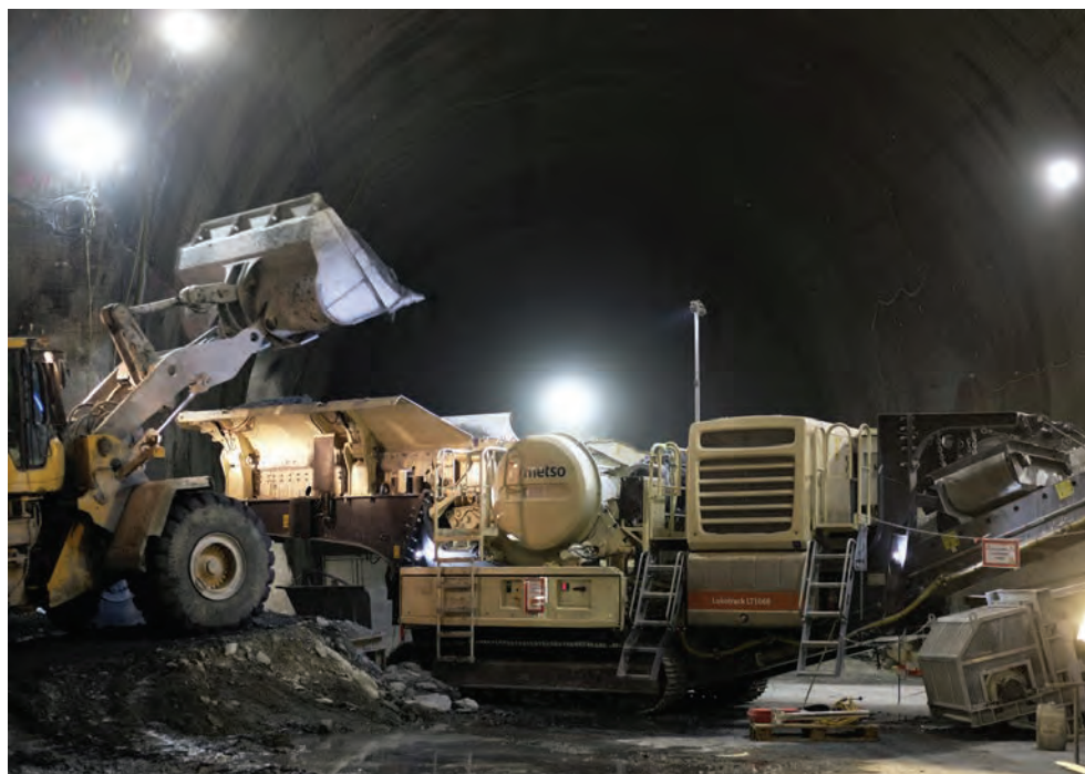
Metso has developed a tracked jaw crusher capable of producing 300tph at the face of a tunnel underground.
