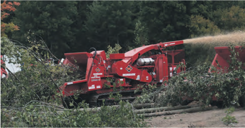
Equipped with the same internal drive perfected on Morbark horizontal grinders, the 40/36 aggressively feeds brushy tops and limbs, quickly and effortlessly filling a chip van to maximum legal load capacity.
