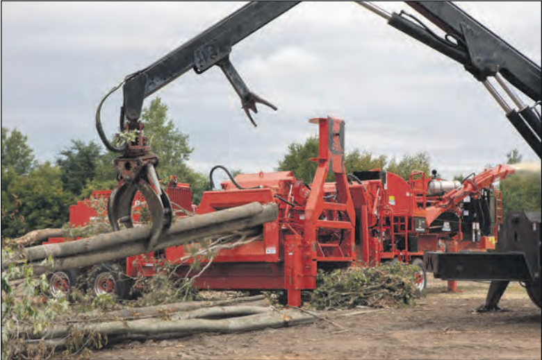
The Model 23 Chiparvester is able to chip large volumes of wood with its 75" (190.5 cm) chipper disc.
