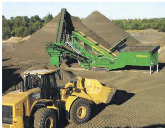
The S130 hopper's 14-foot grid opening allows the use of larger loading shovels.
