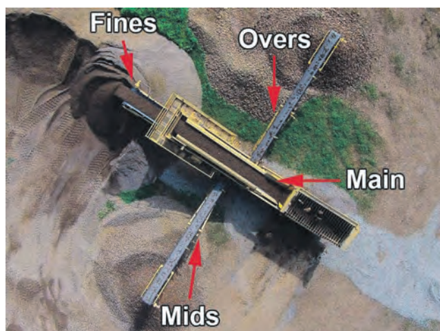
The 514TS3 can deliver four finished products simultaneously.
