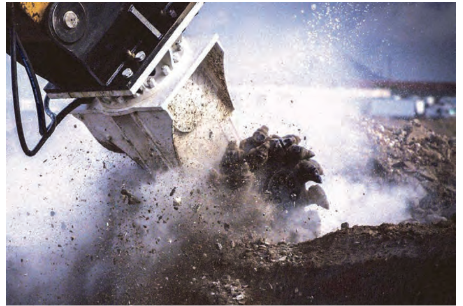
Epiroc's ER 1500 drum cutter is a powerful transverse drum cutter ideal for tunneling, special foundation work, demolition and soil mixing.
