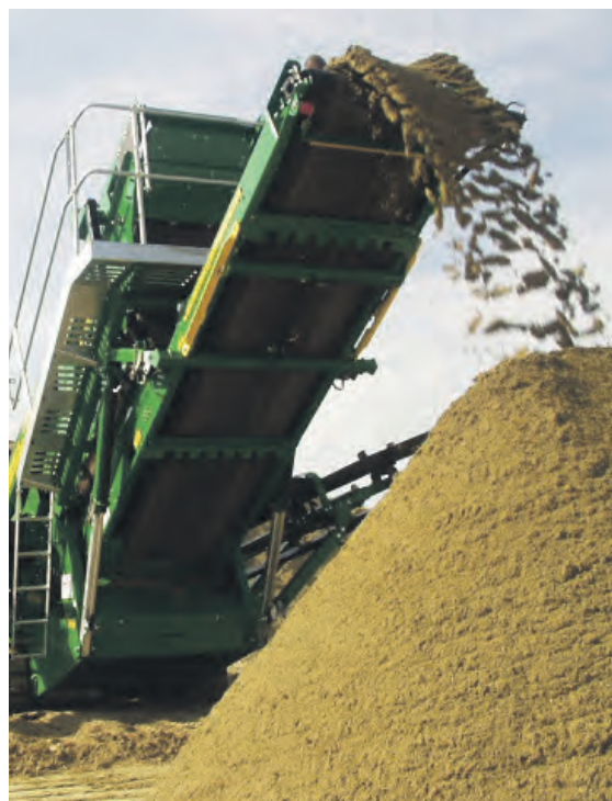
The S80 can employ the steepest screen angle of any three-way-split screening plant currently available, ensuring best-in-class screening ability in materials like sand and peastone.
