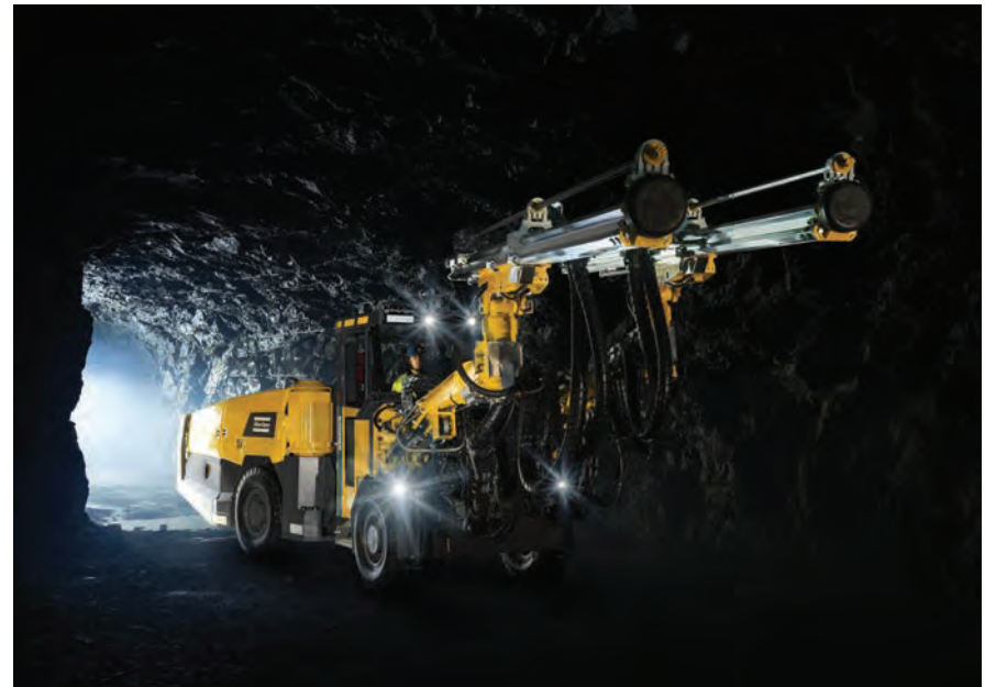
Atlas Copco's (Epiroc) compact tunneling jumbo has been developed specifically for drill and blast in small tunnels.
