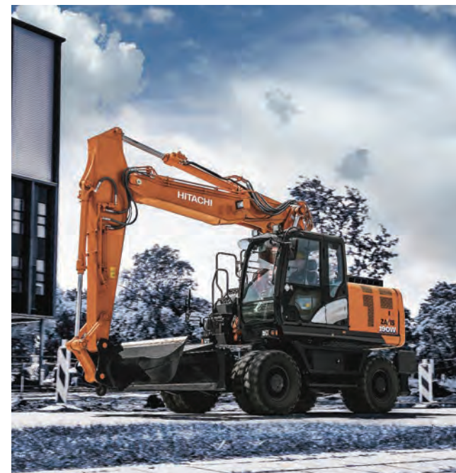
Mobile and maneuverable, Hitachi's wheeled excavator weighs in at 45,300 lbs. and sits on a short wheelbase that makes it easy to work in tight spaces.
