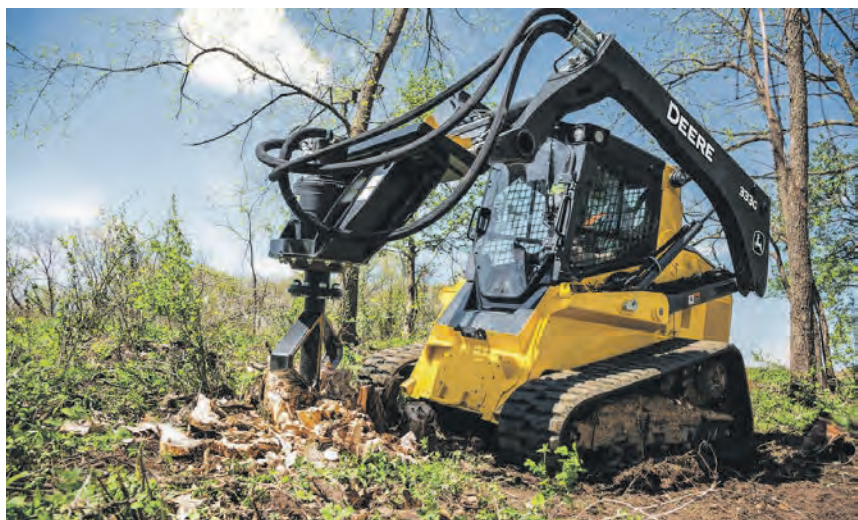
Ideal for landscaping and construction job sites, the new shredder removes stumps from 8 inches to 28 inches in one pass.
