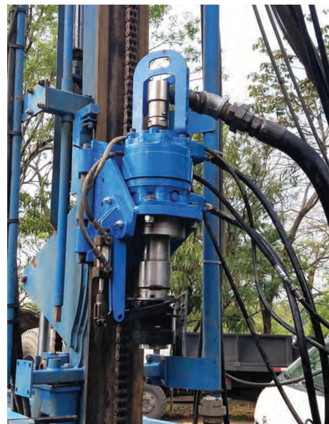
Lone Star offers the LS400T+ with two different Rineer motors, both providing greater torque and easier serviceability compared to the drill's previous hydraulic motor.
