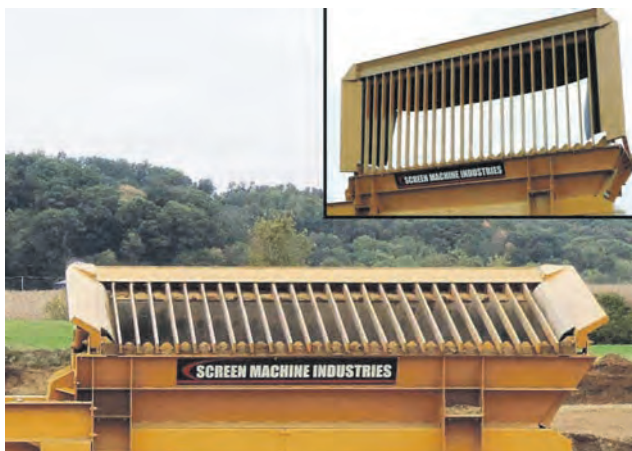
Both models come with standard grizzly and an eight cubic yard hopper.
