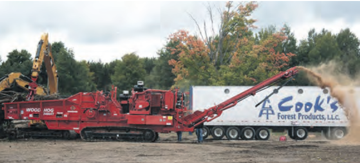
The 6400XT's infeed bed is 24 inches (60.96 cm) longer than previous Morbark grinders in the 1,000-plus horsepower range and has sloped sides.
