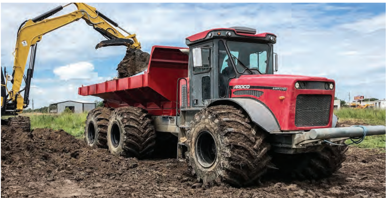
The dump beds are among many interchangeable ARDCO attachments compatible with the back-end platform of the AMT.
