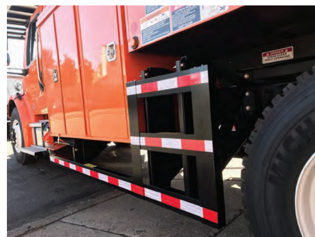
The guards prevent people from being pulled under the vehicle's wheels and run over in the case of a collision.
