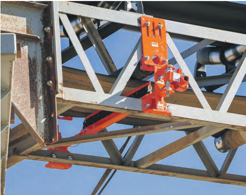
Blade replacement is a simple operation by removing the lock pin and sliding out the cartridge.
