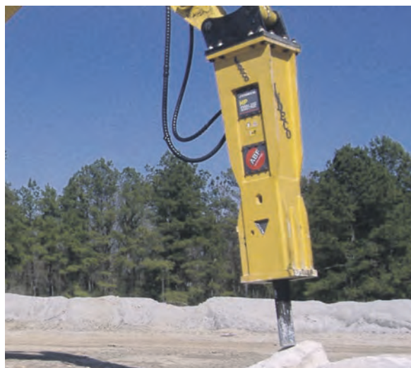
Many modern breakers optimize the hydraulic pressure delivered by the machine, thus improving jobsite productivity and enhancing overall machine performance.
