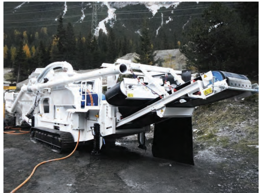
Austrian manufacturer SBM Mineral Processing GmbH has purpose-developed a low height tracked jaw crusher for tunneling.
