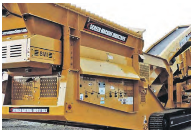
The Spyder 514TS is a patented track-mounted, reverse screening plant designed for primary or secondary screening. Photos courtesy of Screen Machine
