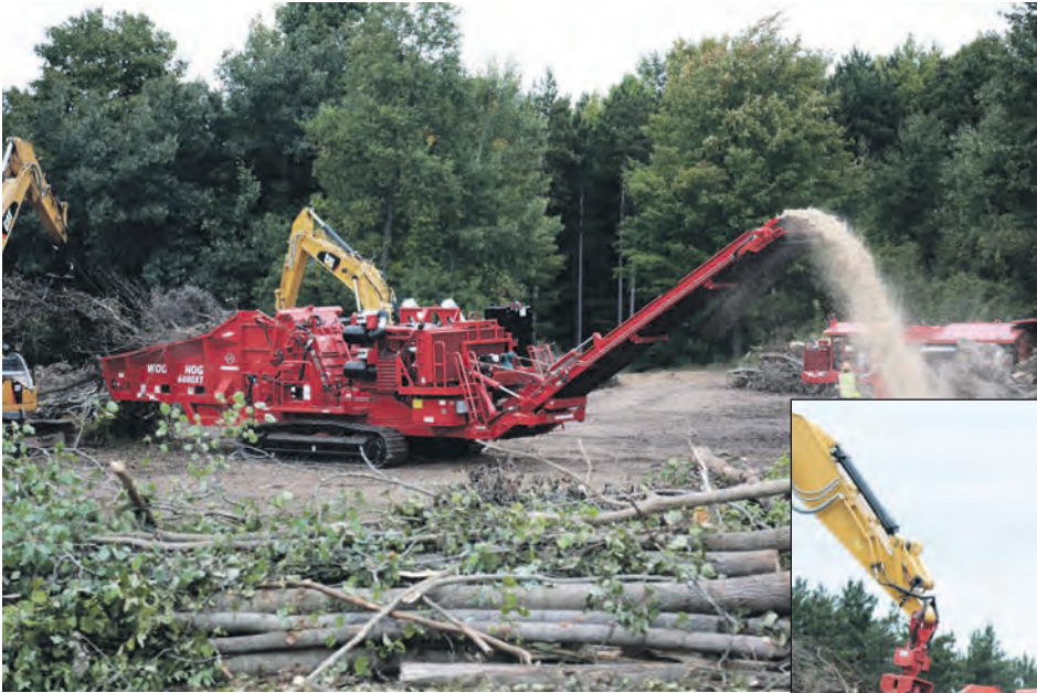
The 6400XT's infeed bed is 24 inches (60.96 cm) longer than previous Morbark grinders in the 1,000-plus horsepower range and has sloped sides.
