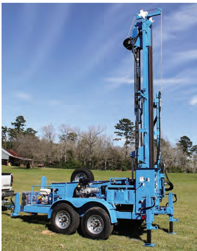
The new high-torque Rineer rotary vane hydraulic motor on Lone Star Drills' LS400T+ reduces rotary service time from days to less than an hour.
