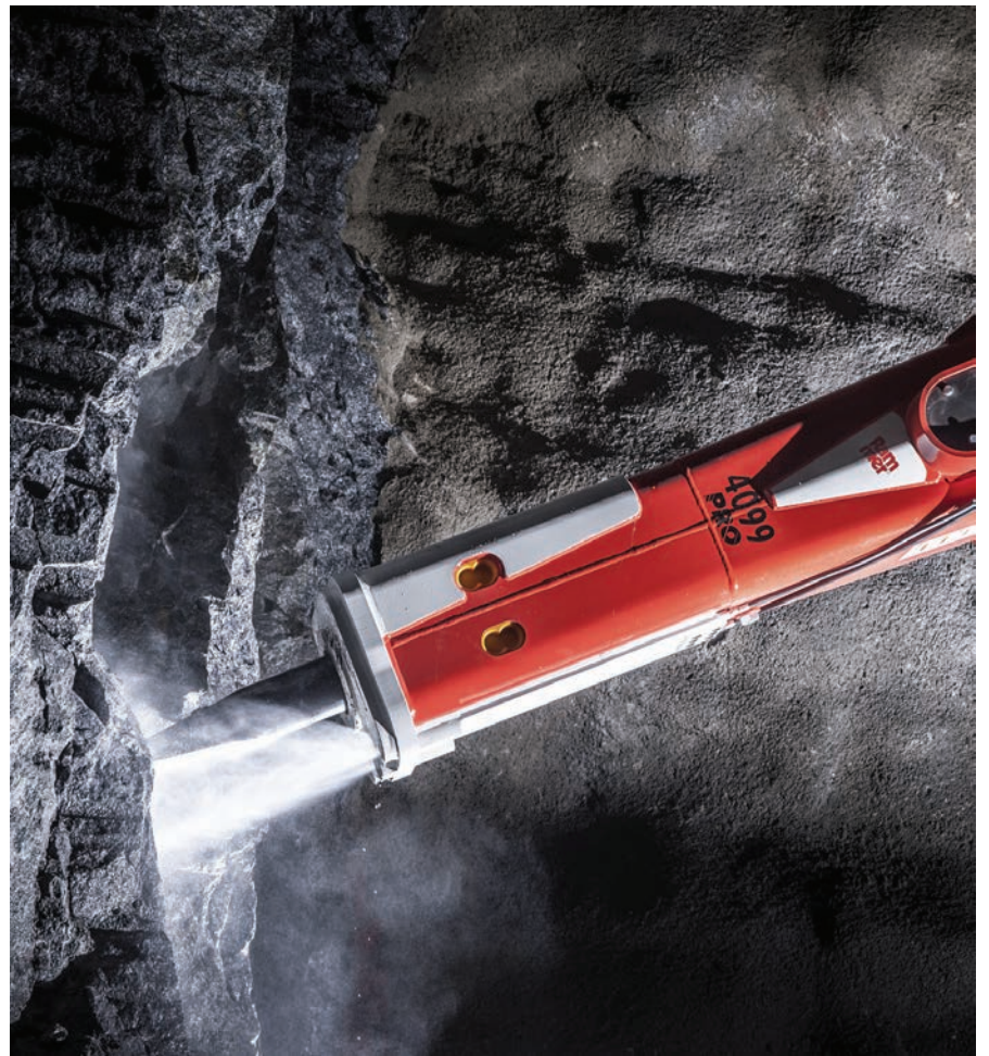
Rammer has developed a special water jet system which is designed to suppress airborne materials or dust during hammer operation.
