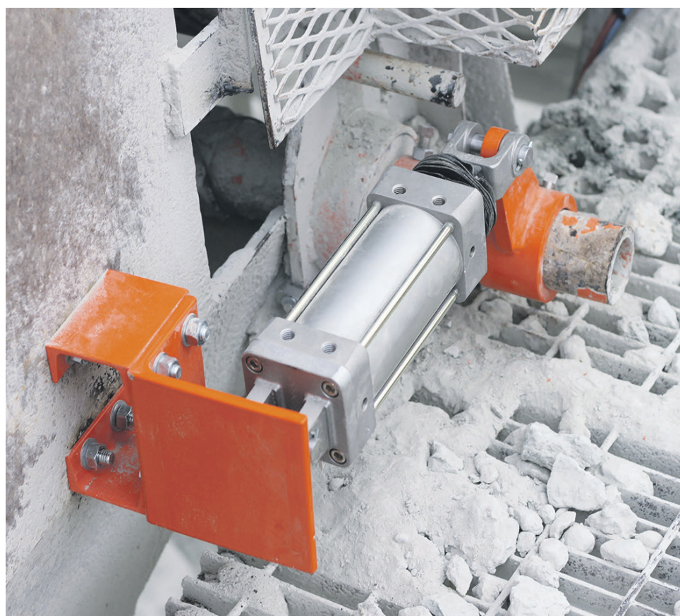
The Automated Blade System eliminates the need for manual blade tensioning.
