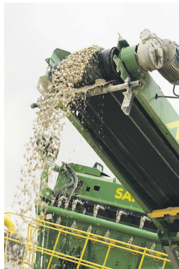
The plant processes limestone secondary crusher screenings to produce three spec concrete/asphalt aggregates and one spec concrete sand product.
