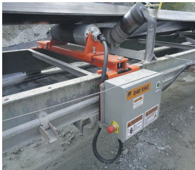
The Roll Gen System uses the movement of the belt to produce localized power.
