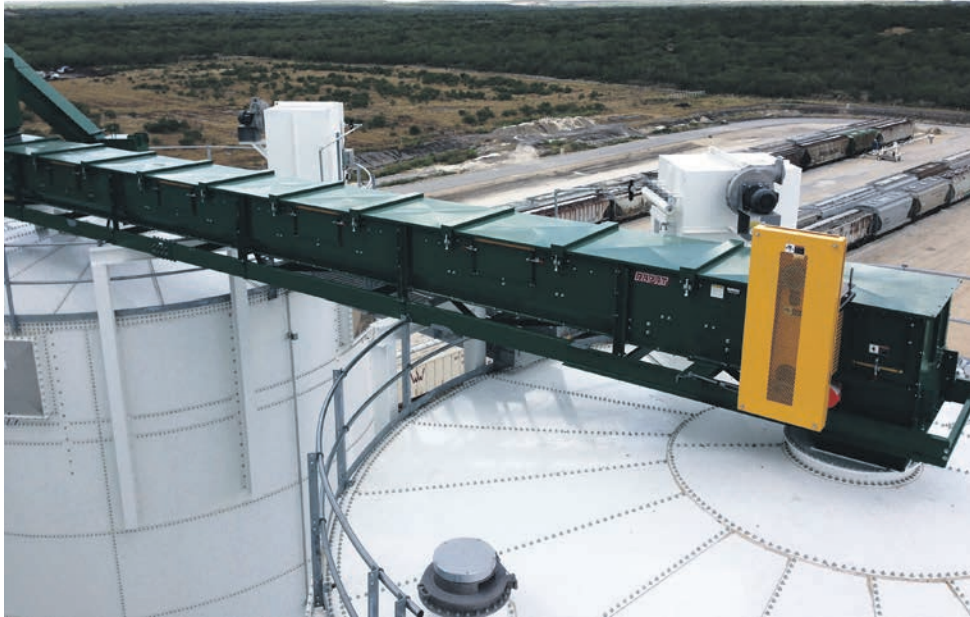
Rapat Corporation's complete line of enclosed conveyors helps eliminate dust emissions. Photos courtesy of Rapat Corp.
