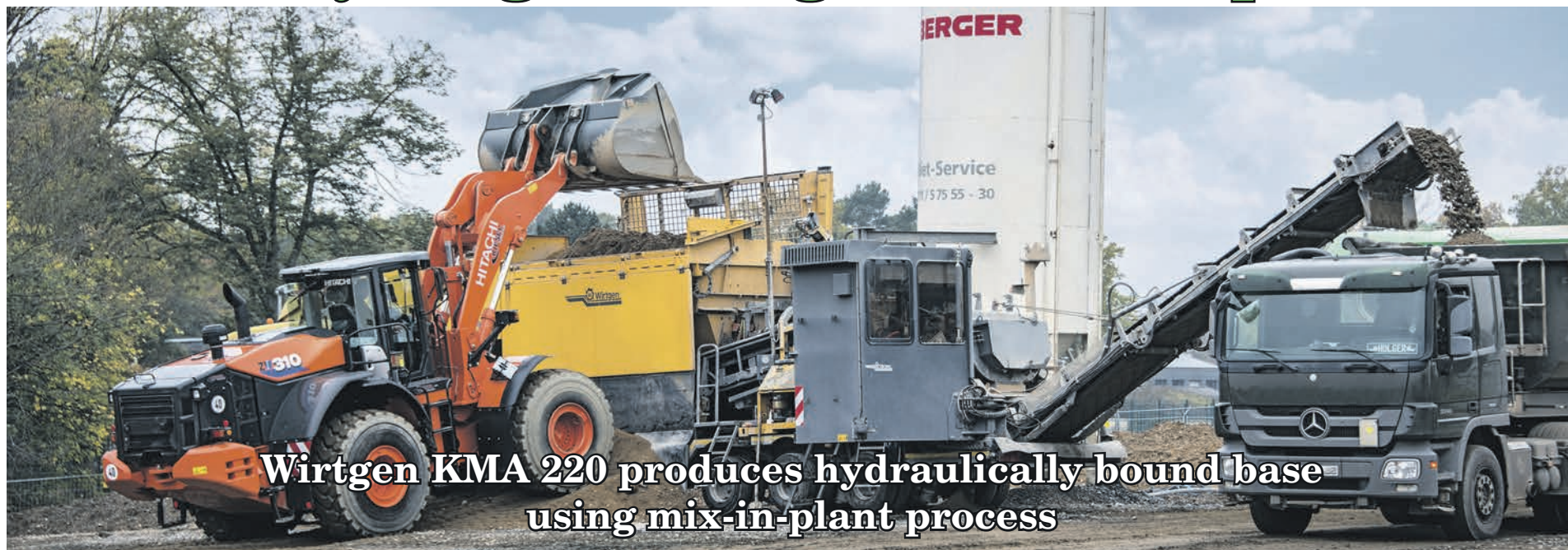
The mobile KMA 220 from Wirtgen can accommodate two different aggregate materials in the capacious twin-chamber proportioning hopper.
