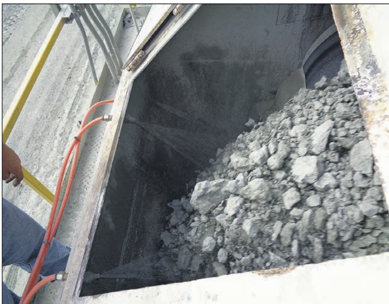
Left: To control fugitive emissions, the Martin Surfactant Dust System treats the cargo at the transfer point.
