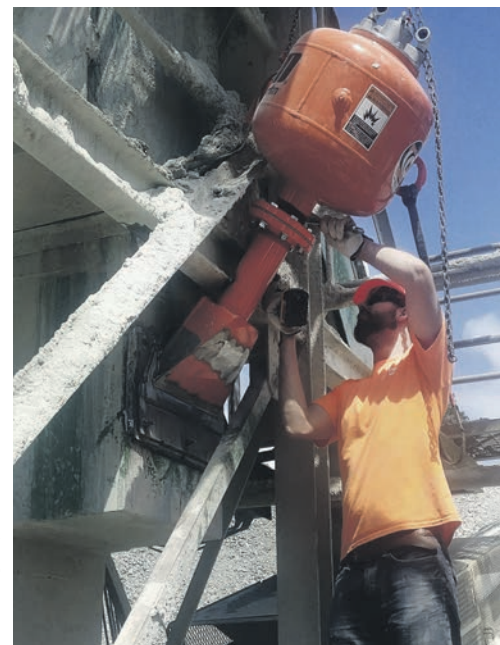
Right: The 70-L Hurricane Air Cannon features a fan jet nozzle for wide coverage.
