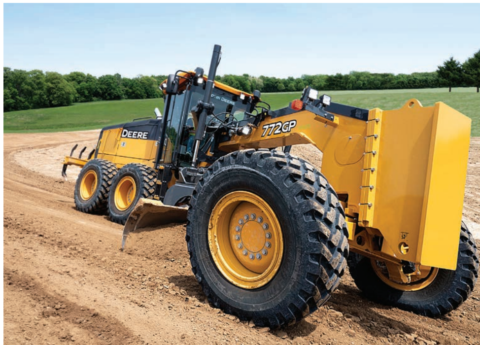
The system is fully incorporated into the machine's structures and software, delivering precise grading performance while eliminating vulnerable masts and cables.
