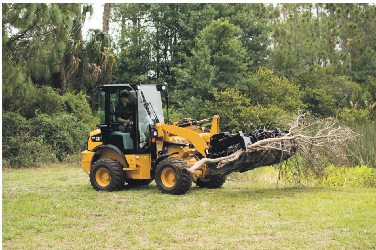
The differential locks can be engaged "on-the-fly," allowing the 903D to respond instantly to changing ground conditions.
