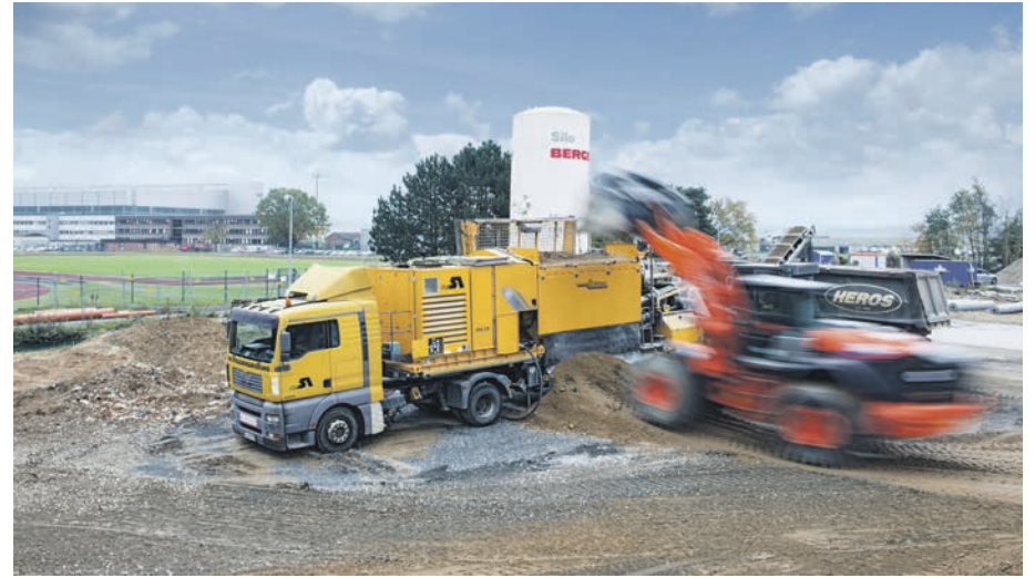
The KMA 220 from Wirtgen measures 14.71 m in length for transport, including the cabin. The transport width is only 2.50 m, though, because the cabin is folded in for transport.
