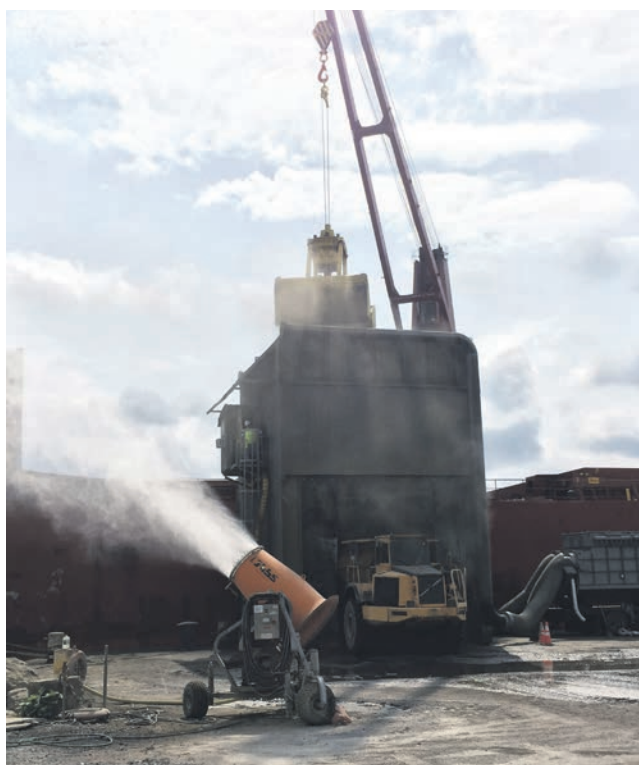
A clamshell shovel suspended from a crane slowly unloads the material into a tall portable hopper with a baghouse dust
