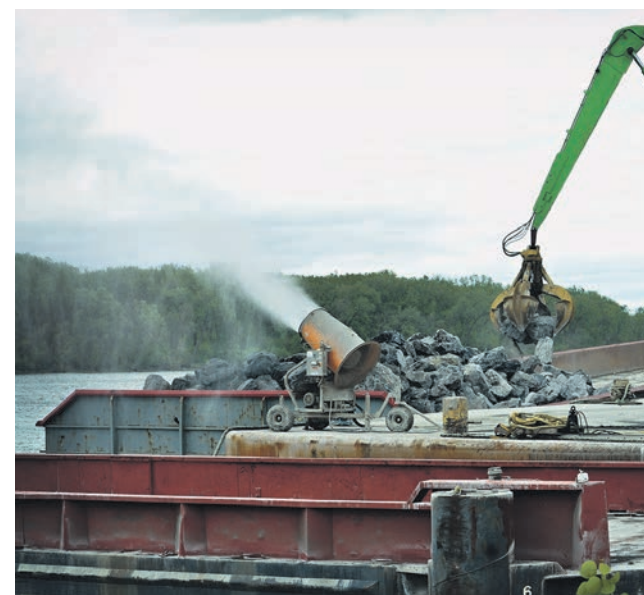
The cannons are easily positioned on the dock, taking up little room and covering a large area.
