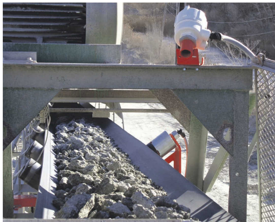
Powered by the Roll Gen, a sensor detects material on the belt and communicates with control systems.
