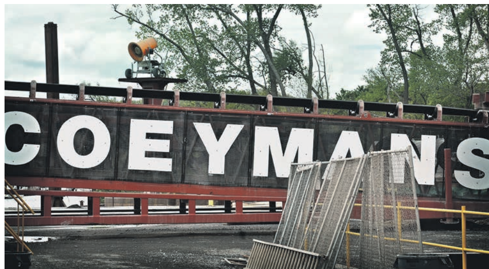
Mounted on a tower, the DB-60 suppresses dust over metal scrap recycling piles.
