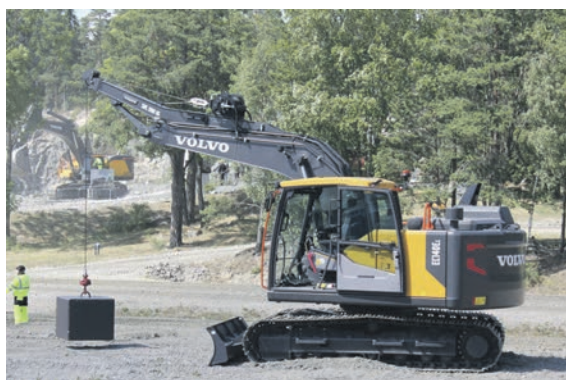
The pipelayer kit converts EC140D, EC140E and ECR145E excavators into a pipelayer for lowering pipes.
