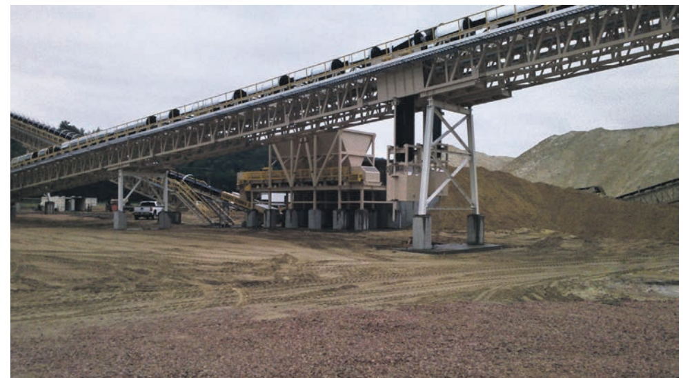
The Rapat Series ETR is a totally enclosed-frame conveyor with CEMA troughing idlers and a self-cleaning UHMW slide belt return.
