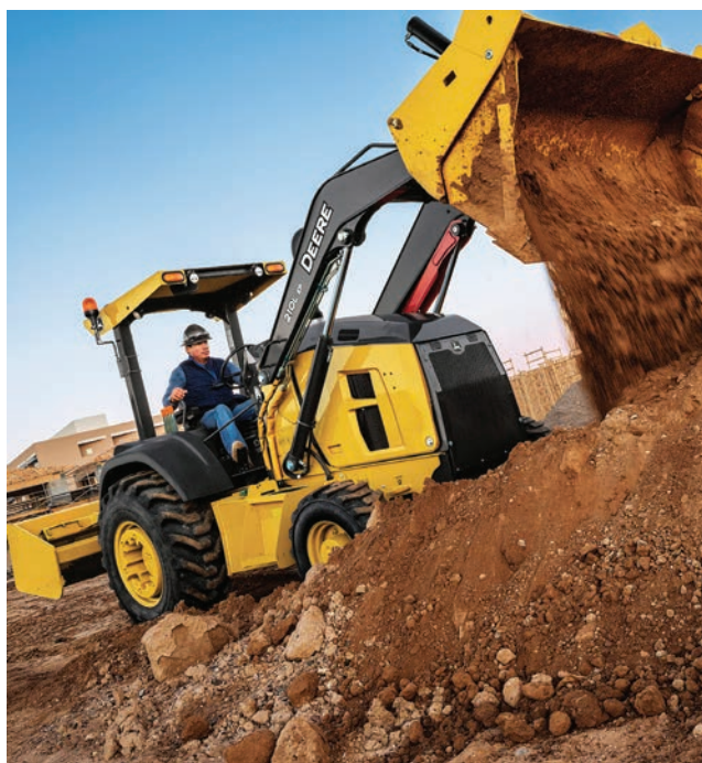
Loader lift times are 26 percent faster due to increased hydraulic pump flow and larger diameter hoses and tubes.
