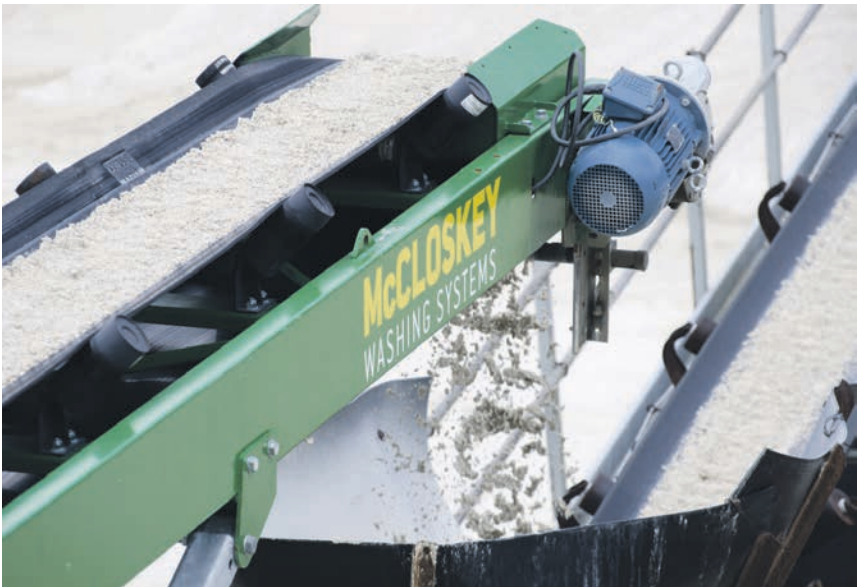
The sand plant also has the capability to blend all or some of the fine sand into the coarse sand to maximize the required grading.
