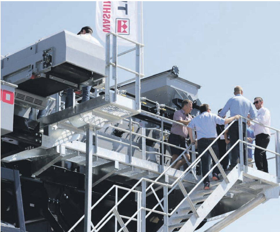
Above: AggWash 300's high performance solution brings together rinsing, screening, scrubbing and sand washing capabilities on a single plant.
