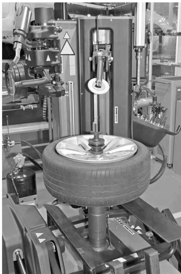
Tire balance is checked on a machine that will measure heavy spots. Technicians will apply weights to the tires to balance any inconsistencies in weight.
