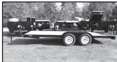
50'x16' GAC Angle Wood Deck Car Carrier, 4' Pull Out Ramps, Stake Pockets, 7,000# GVWR
