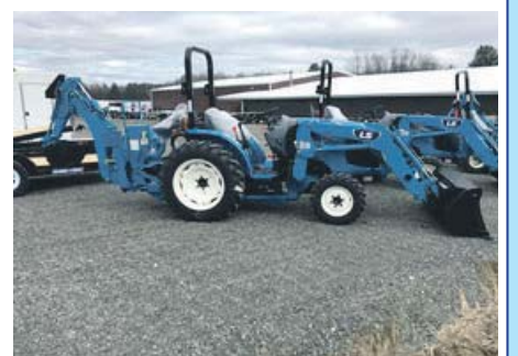
40 Horsepower Tractor, Gear Transmission with Front Loader and Rear Backhoe with 16" Bucket
