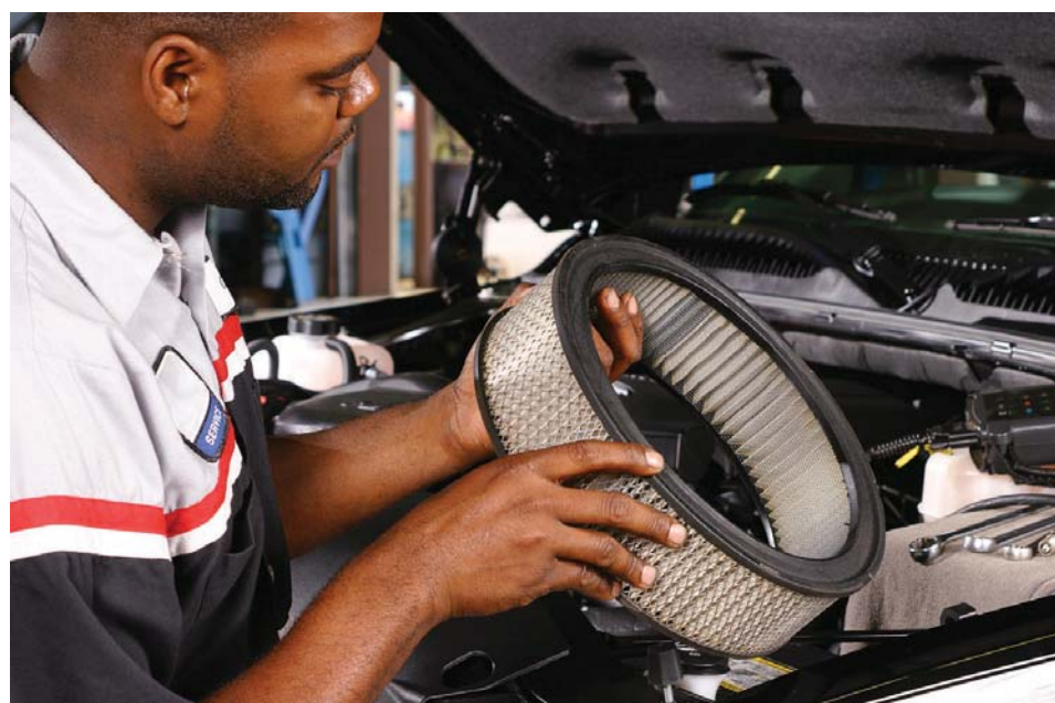
Air filters need to be changed regularly to maintain the right flow of air into the engine and to protect the engine from debris.
