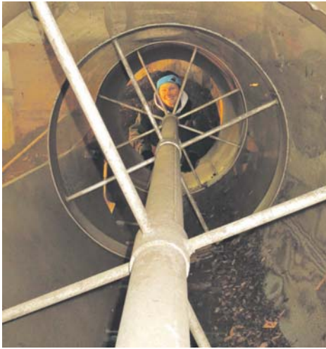
The Worm Queen uses a homemade rotary drum to screen the vermicompost into the final dried product
