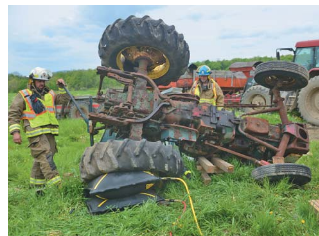
Air bags lift the tractor as blocks are used to hold it in place as it is lifted higher.
