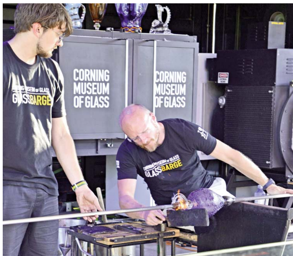
The beeswax used to reduce friction – not the soaked wood in his hand – briefly ignites as glassworker G. Brian Juk, assisted by Lukas Milanik, work on attaching a punty to the bowl they are making.
