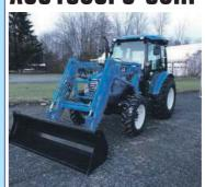
68 HP tractor with full cab, Power shuttle transmission and front end loader
