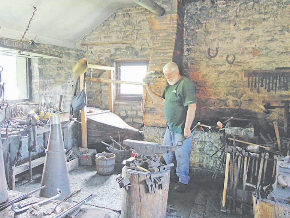
Blacksmith Steve Gurzler begins to create an anvil tool by using bellows to raise the temperature of the fire he has started.
