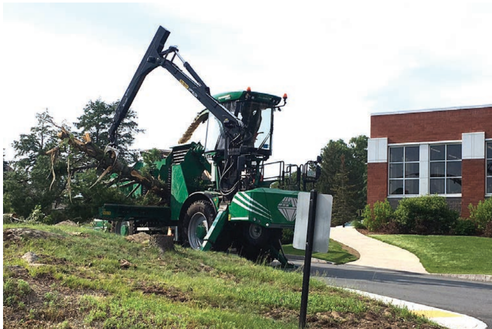
With its stabilizers down and the cab raised, the Diamant 2000 goes from being a mobile shredder to a stationary one with a clear view of the stack being ground and the truck being loaded.
