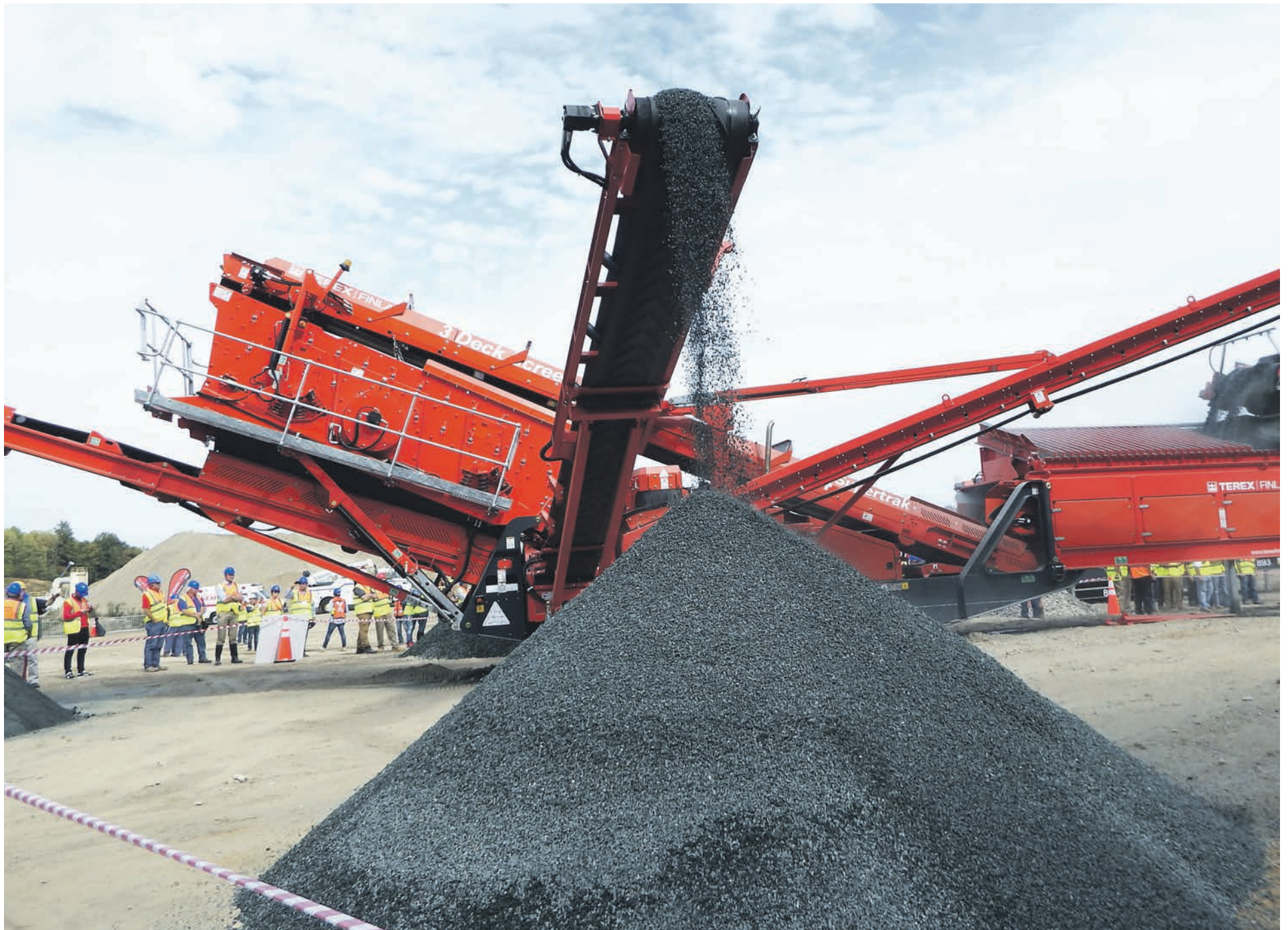
Once material had been crushed through the J-1170 and C-1550, a final screening through this 684 3-Deck inclined screen plant produces an additional four products.
