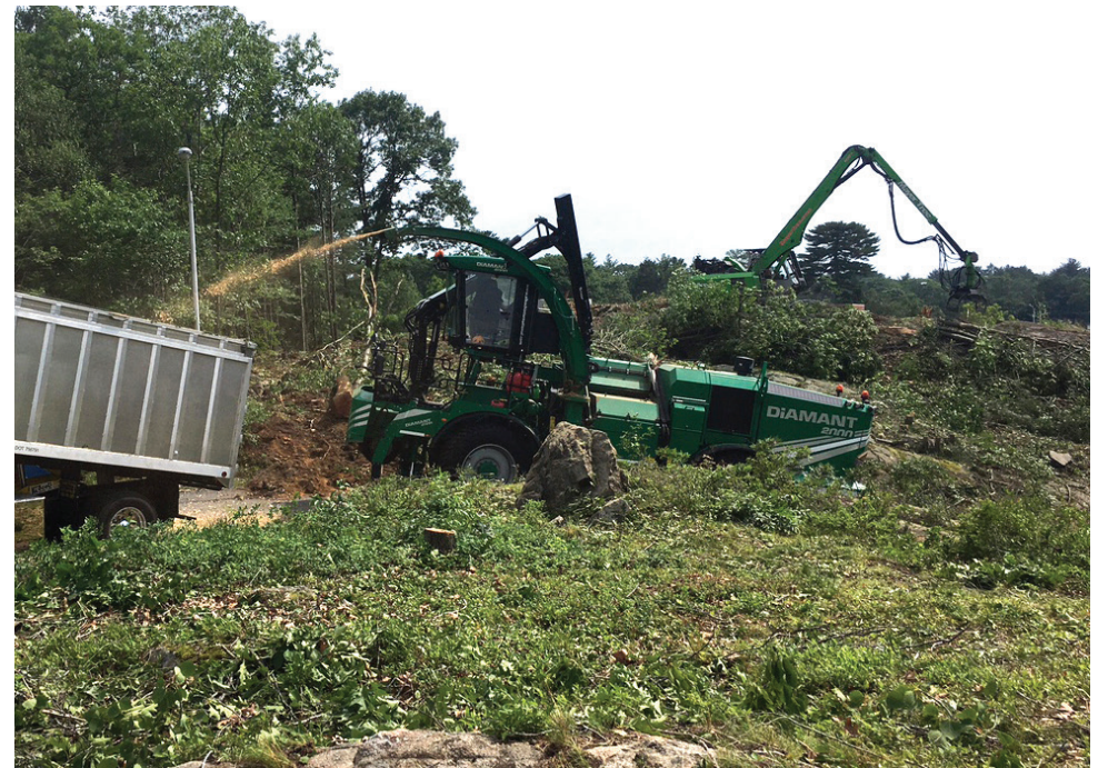
The Diamant 2000 grinds while the material handler cuts, piles and stacks it.
