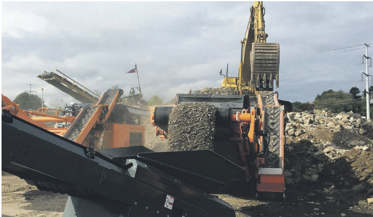
The Impactor R1000S equipped with its optional screening system crushes concrete on the RST18 stacker.
