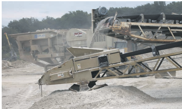
Showing the unusual arrangement of conveyors described in article. The Kafka conveyor (top) comes directly from the secondary, carrying 2"-minus rock to the small hopper on this separate screening conveyor on its way to the CedarRapids free-standing screen.
