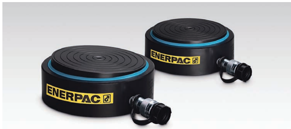
CUSP-Series has an integrated tilting function with 10 to 1,000-ton capacity, 0.26-0.69 inches stroke and maximum operating pressure of 10,150 psi.
