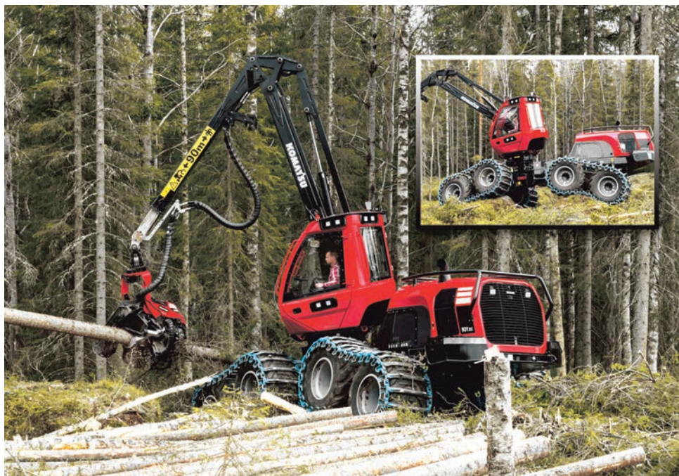
The new Komatsu 931XC is a Harvesting Powerhouse featuring a unique double Komatsu Comfort Bogie 8WD system designed to tackle steep, rough and soft terrain.
