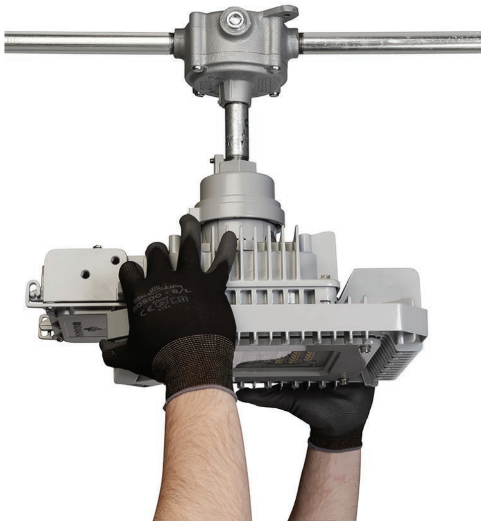
One electrician using standard tools is all that is required to pre-wire the mounting hood, line the arrows up, and lock the Baymaster into place.
