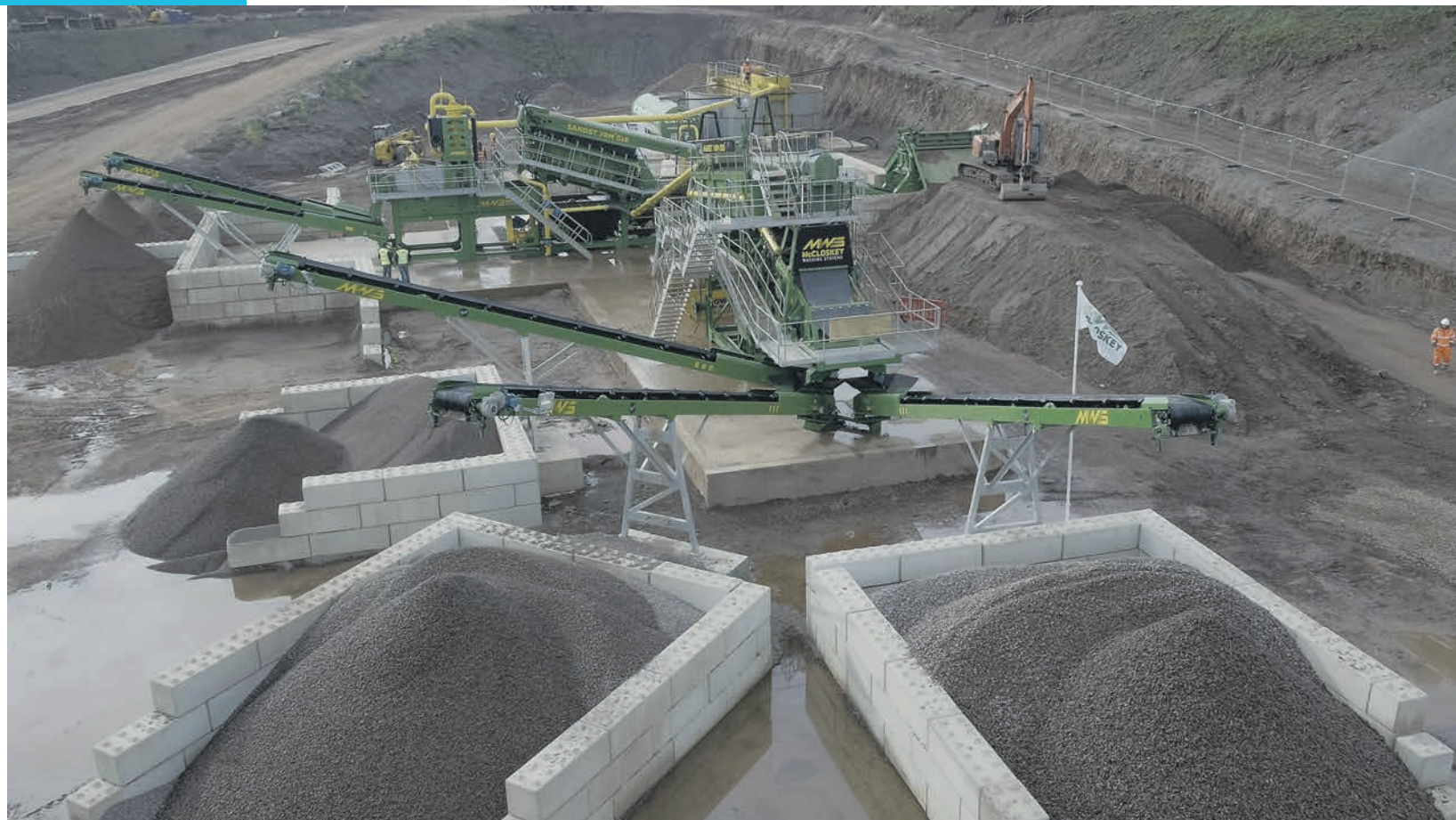
Together, they process quarry scalpings with a high clay content to produce three aggregates and two sand products.
