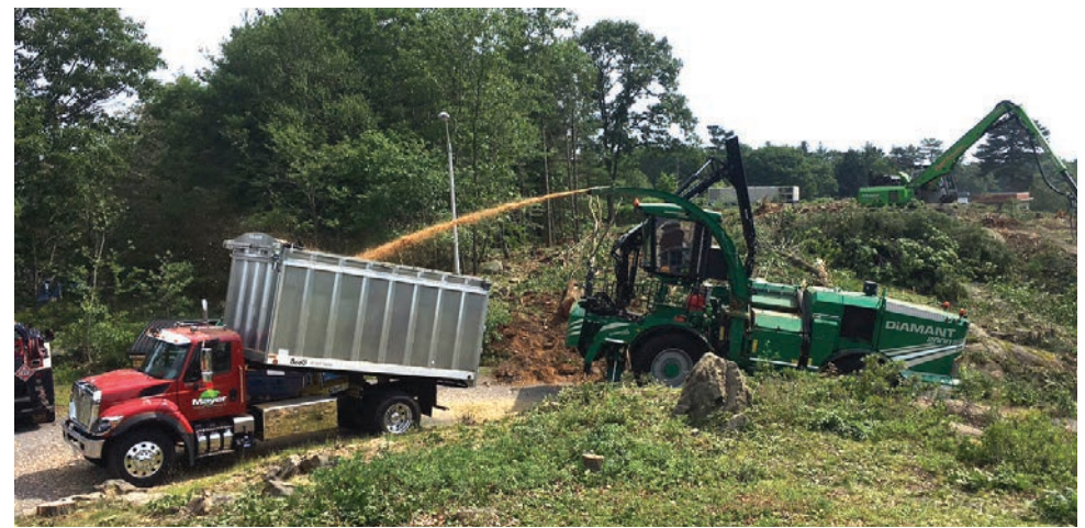
With its swivel seat and raised cab, the operator can use the crane while positioning the chute to load the truck.
