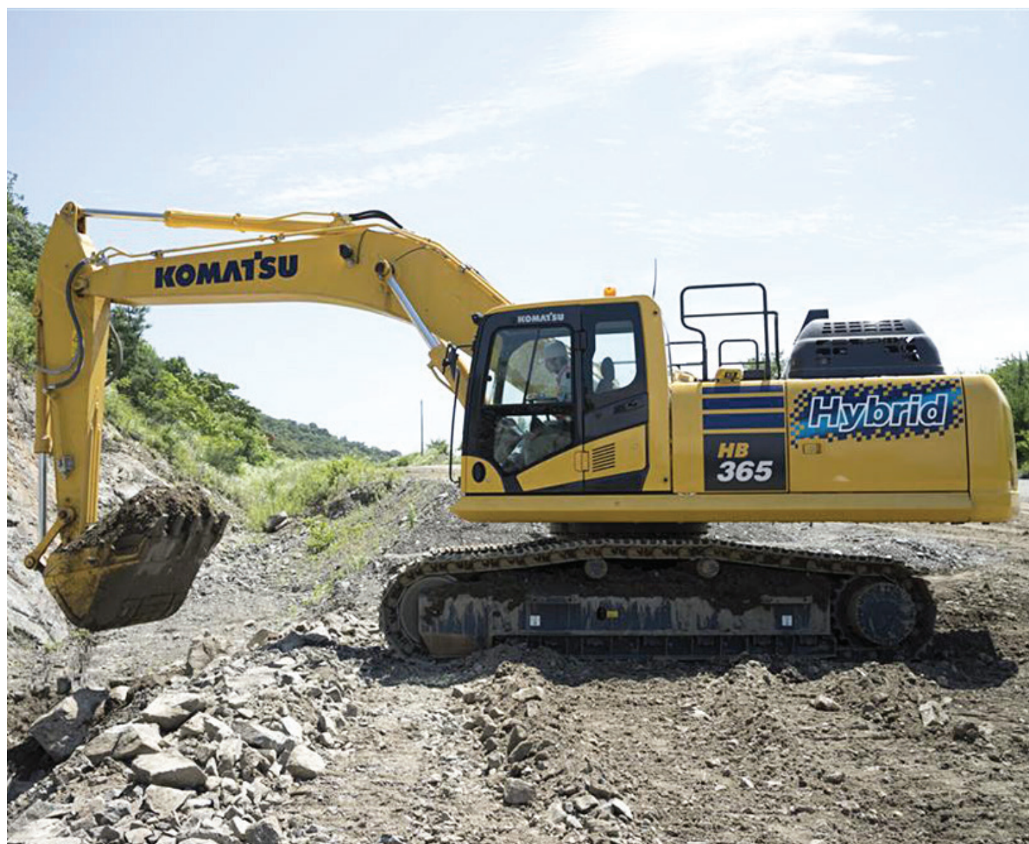
The revolutionary Komatsu Hybrid System uses swing energy regeneration and an ultra-capacitor that provides fast energy storage and instantaneous power transmission.
