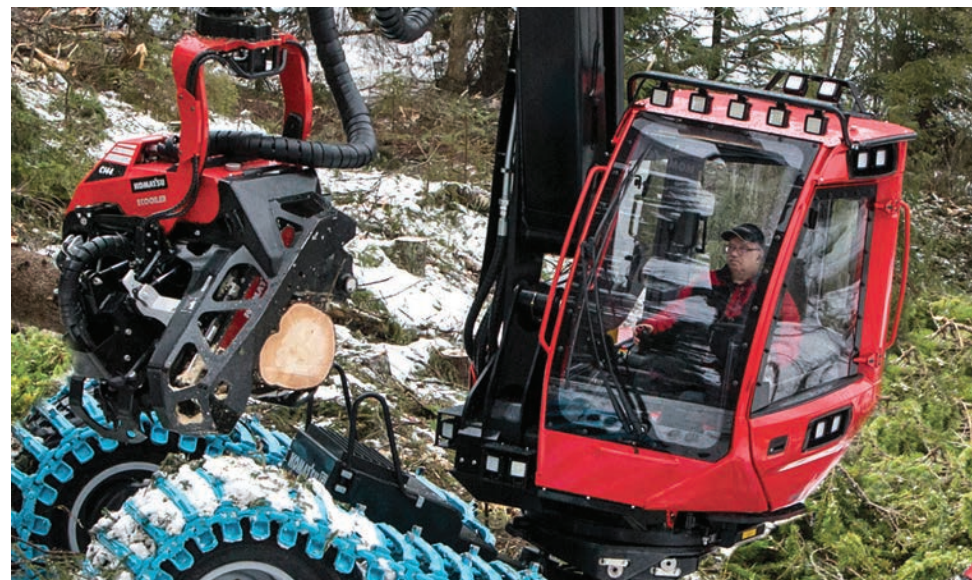
The modern 931XC cab features excellent upward/downward front line-of-sight visibility, 4-way cab/crane leveling and 360° cab/crane rotation.
