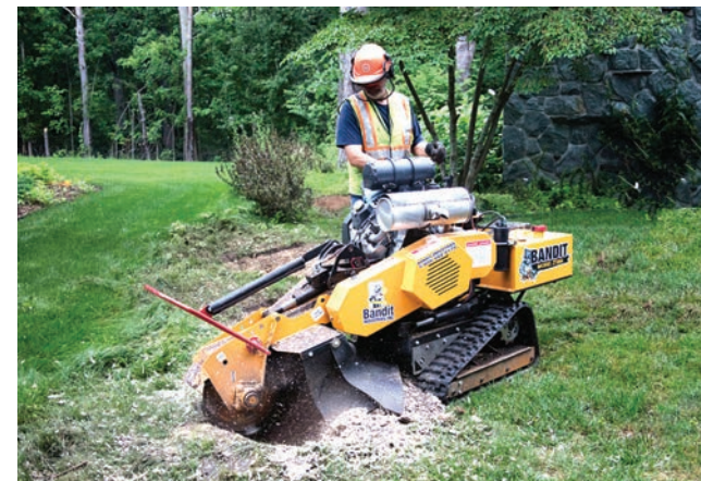
The Model ZT1844 is equipped with an 18-inch diameter Bandit cutter wheel featuring Green Teeth.
