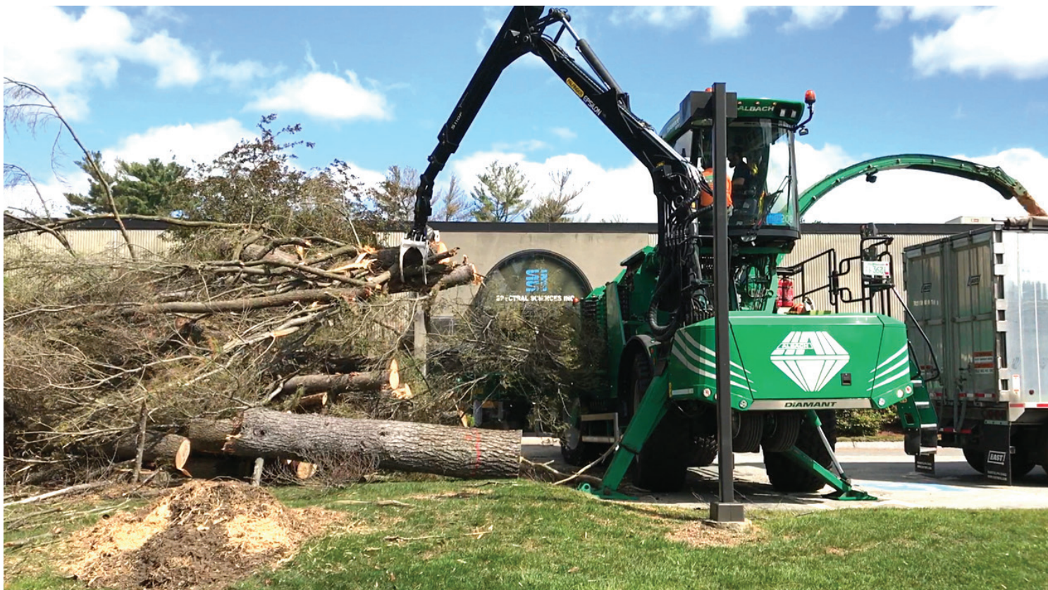
The Diamant 2000 loads on one side while the chute on the other side loads the trailer.
