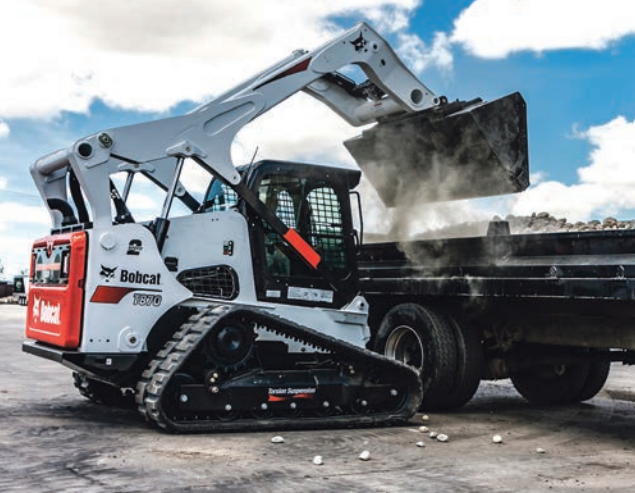
Bobcat lengthened the undercarriage's rubber tracks to increase surface area and ground contact.
