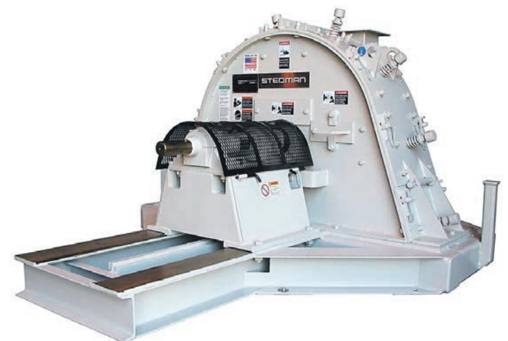
The flared housing design eliminates corners that trap material, reducing clogging and down time.
