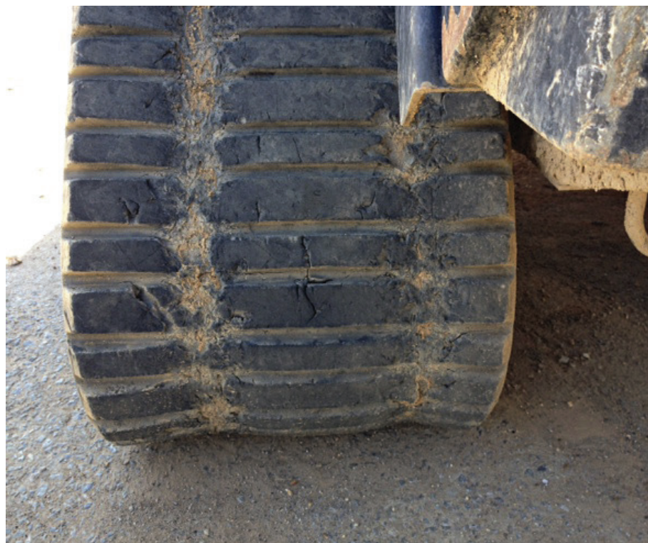
The average rubber track life is about 2,000 hours but can be as high as 5,000 hours with proper maintenance. Neglecting rubber track maintenance, however, can result in a wear life as low as 500 hours. The tread in this track is gone so it is at the end of its serviceable life.
