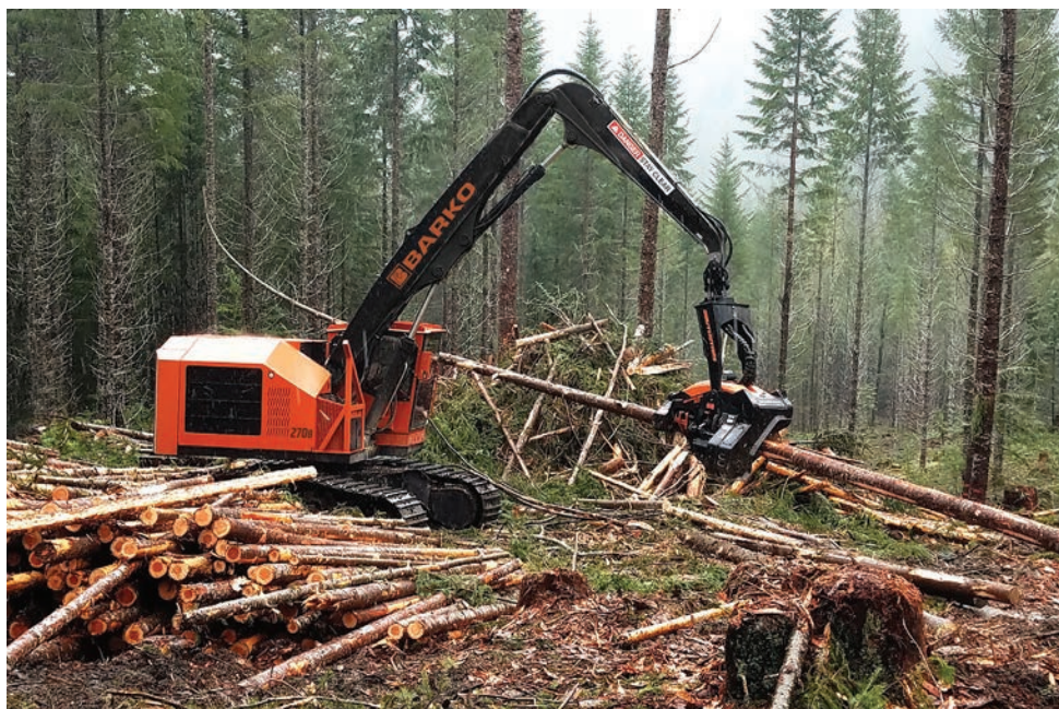
Offering exceptional horsepower, swing torque and tractive effort, the 270B features a dangle head boom configuration for picking, delimbing, cut-to-length harvesting, and stacking.
