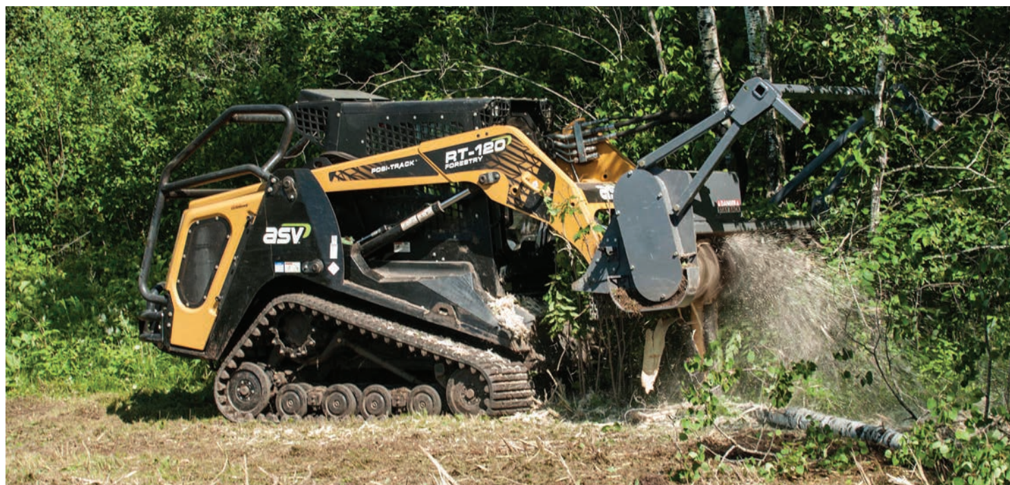
ASV Holdings Inc.'s RT-120 Forestry Posi-Track compact track loader delivers maximum size and power for workers in the forestry industry. The machine's durability, strength and innovative undercarriage make easy work of demanding tasks such as mulching, brush cutting and highway and utility work.
