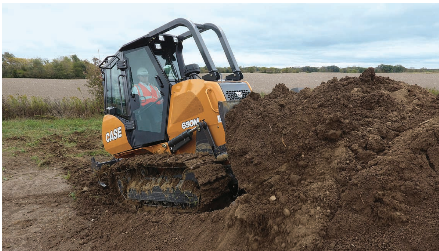
The new 650M also features an enhanced undercarriage with improved track frame, idler, sprockets, rollers and extended-life SALT HD tracks, as well as a reinforced mainframe.
