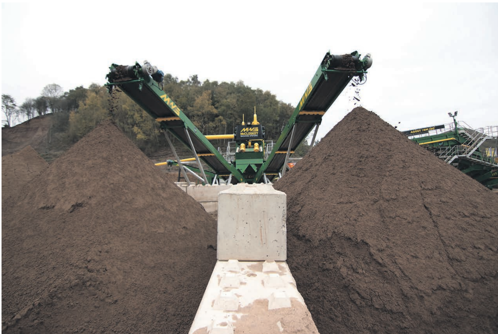
The modular wash plant SandStorm™ 516's unique features deliver exceptional results, producing 0-2 and 0-5mm grades of sand while producing plus 40mm rinsed stone.
