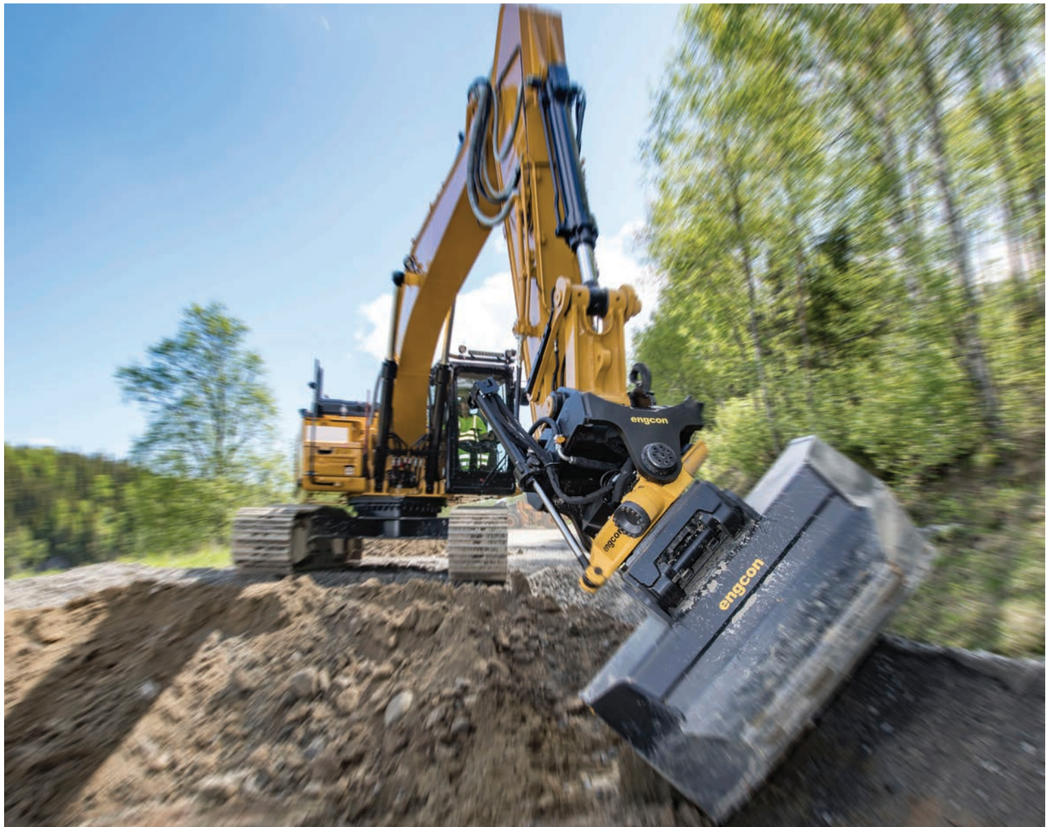
Engcon's new EC233 series tiltrotator has a break torque of 340 kNm (240,771 lbf-ft), making it the market's most powerful tiltrotator built for excavators up to 33 metric tons.
