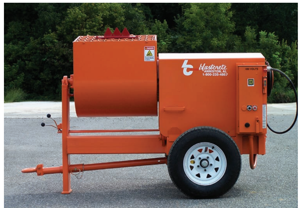
Blastcrete Equipment's refractory paddle mixer combines as much as 500 pounds of refractory castable, mortar or grout in less than two minutes.
