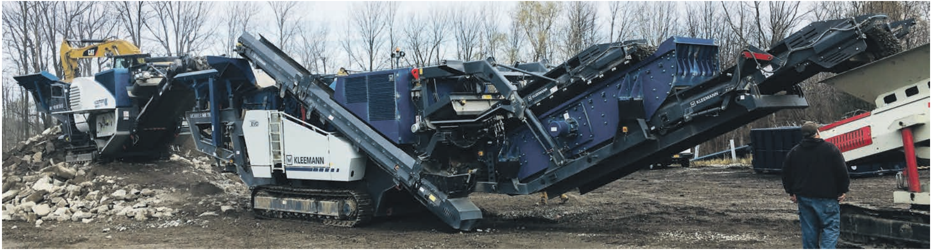
For the two-phase project, Osborne utilized Kleemann crushers to process the material in order to get it ready for their site.
