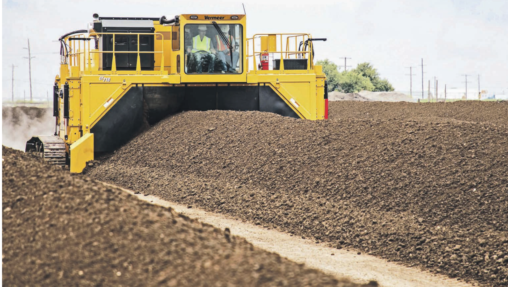
Vermeer compost equipment is designed to process up to 4,000 cubic yards (3058.2m 3 ) of compost per hour depending on the type and size of the turner.
