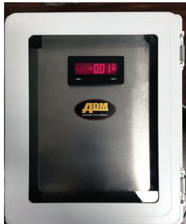
The digitized fuel meter linked to the control house provides an easier and safer way to measure fuel consumption.
