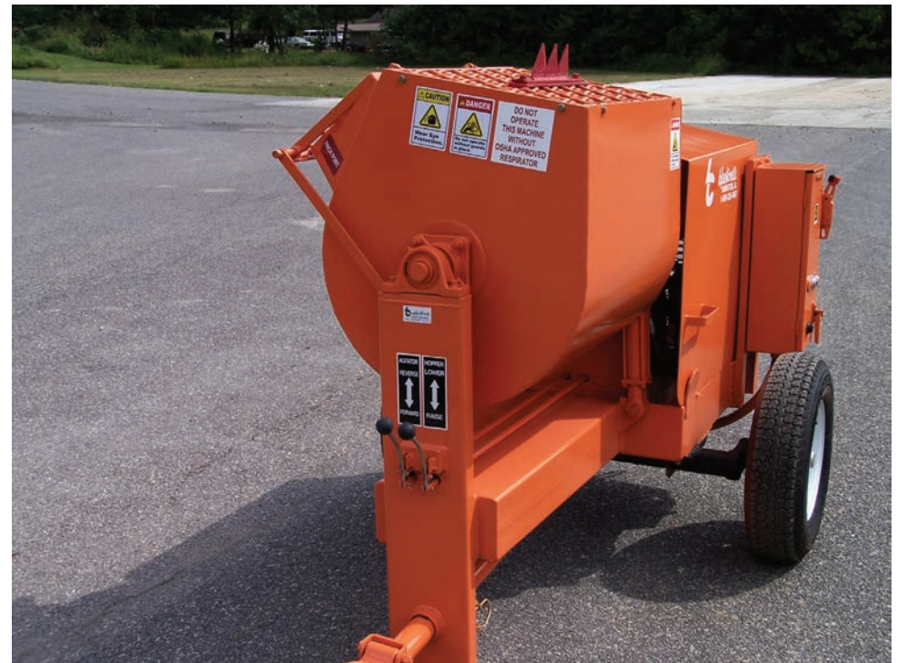
The refractory paddle mixer features hydraulic controls for forward, reverse and dumping.
