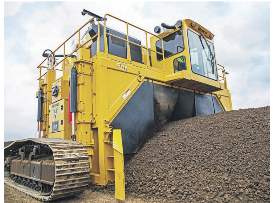
The new full track option is one of four drive systems available for Vermeer's CT718. Also offered are two wheel drive, four wheel drive and two wheel plus two short tracks drive system.
