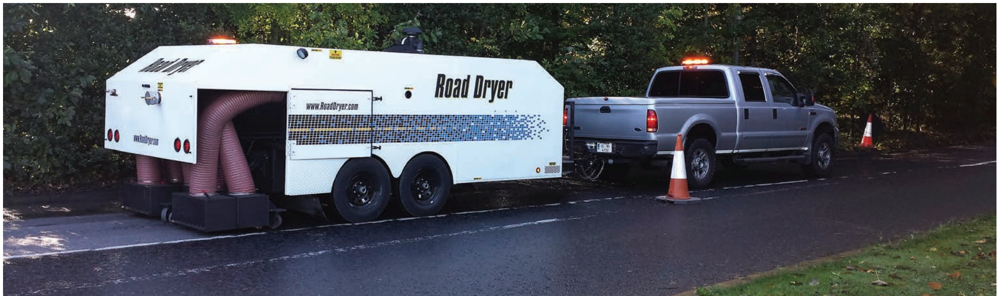
The Road Dryer swiftly and safely dries the pavement.
