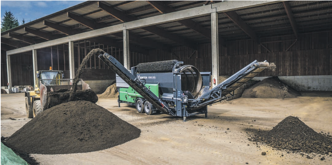
Left: Komptech's Nemus 3000: longer discharge belts and the ability to use screen drums from competitor machines are further benefits of this highly practical machine.
