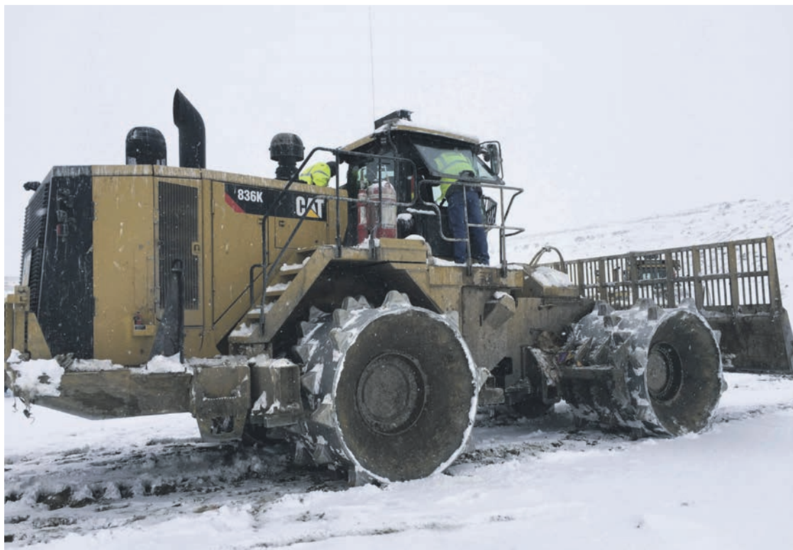
Trans-Jordan employs two Cat 836K landfill compactors equipped with JohnnyBall 3D onboard measuring systems to maintain a level top.
