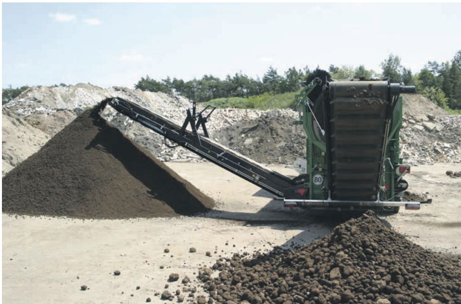
Komptech's new Nemus 3000 is a drum screener that has been designed for low maintenance and service friendliness.
