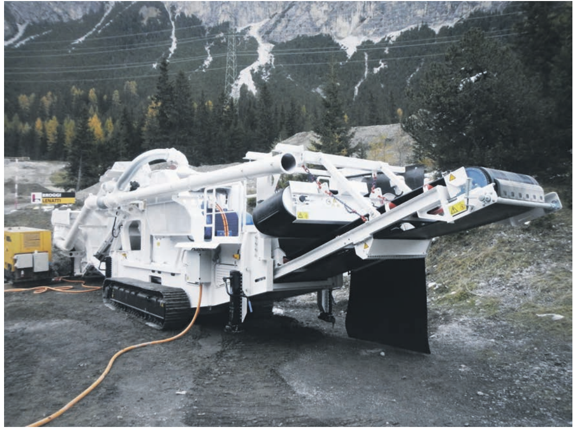
SBM's STE 100.65 TV PB mobile track-mounted jaw crusher has been tailored for the unique conditions experienced in tunnel construction.
