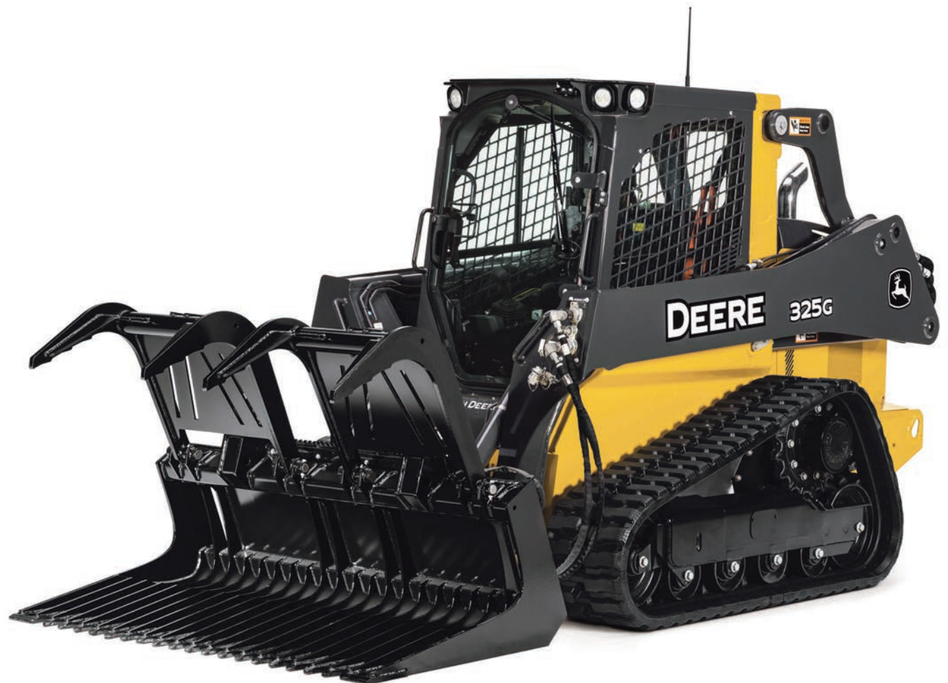
The rock grapple buckets are perfect for land clearing, job site cleanup and brush removal applications.
