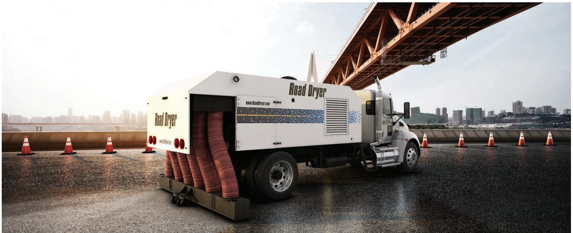
The unit blows heated air up to 300° F directly downward through multiple nozzles to dry the surface.
