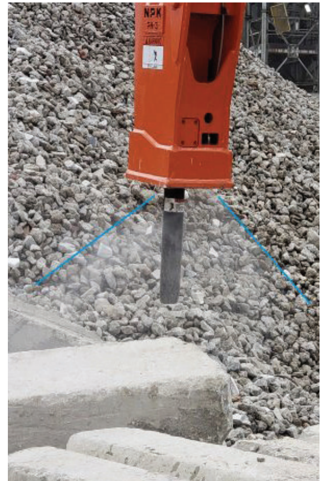
Located in the bracket of the hammer keeping it safe from flying debris, the nozzle is aimed where the tool makes contact with the breaking area.
