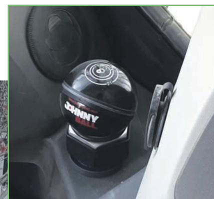
Right: All machines use JohnnyBall 3D onboard measuring systems, which are designed to provide operators with real-time level and slope.
