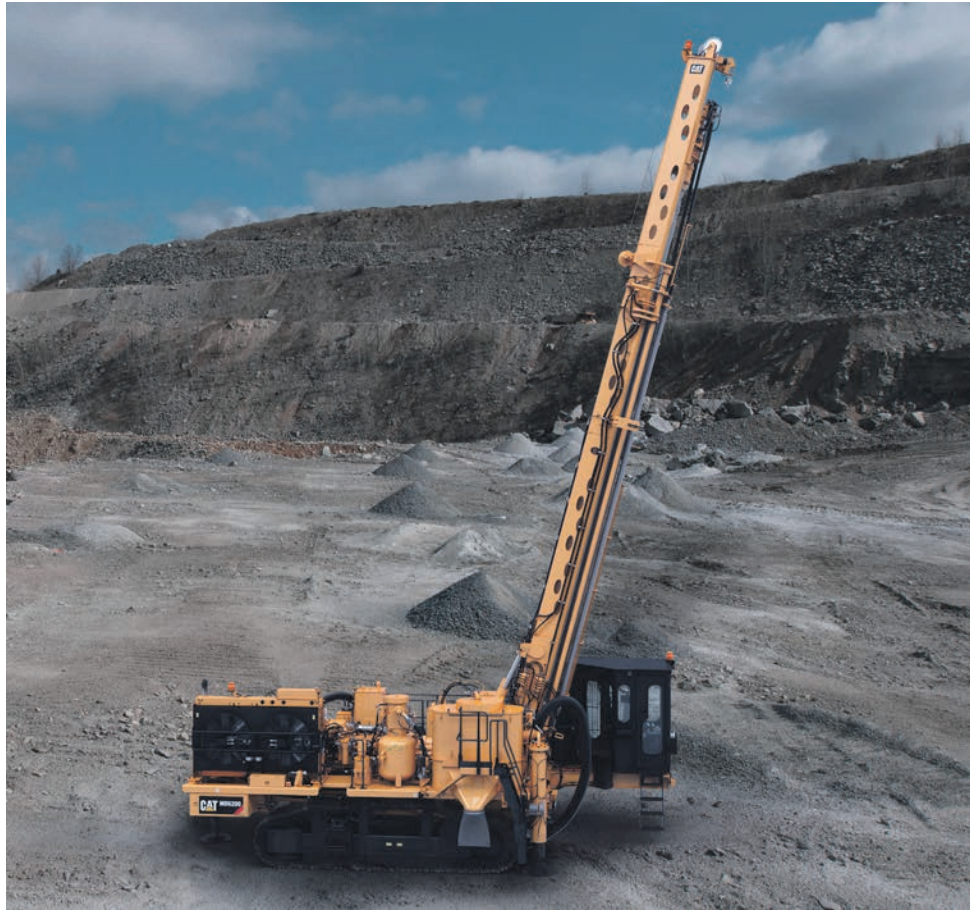
The operator can adjust the mast angle in increments of five degrees from the touchscreen in the cab — with no special setup required.
