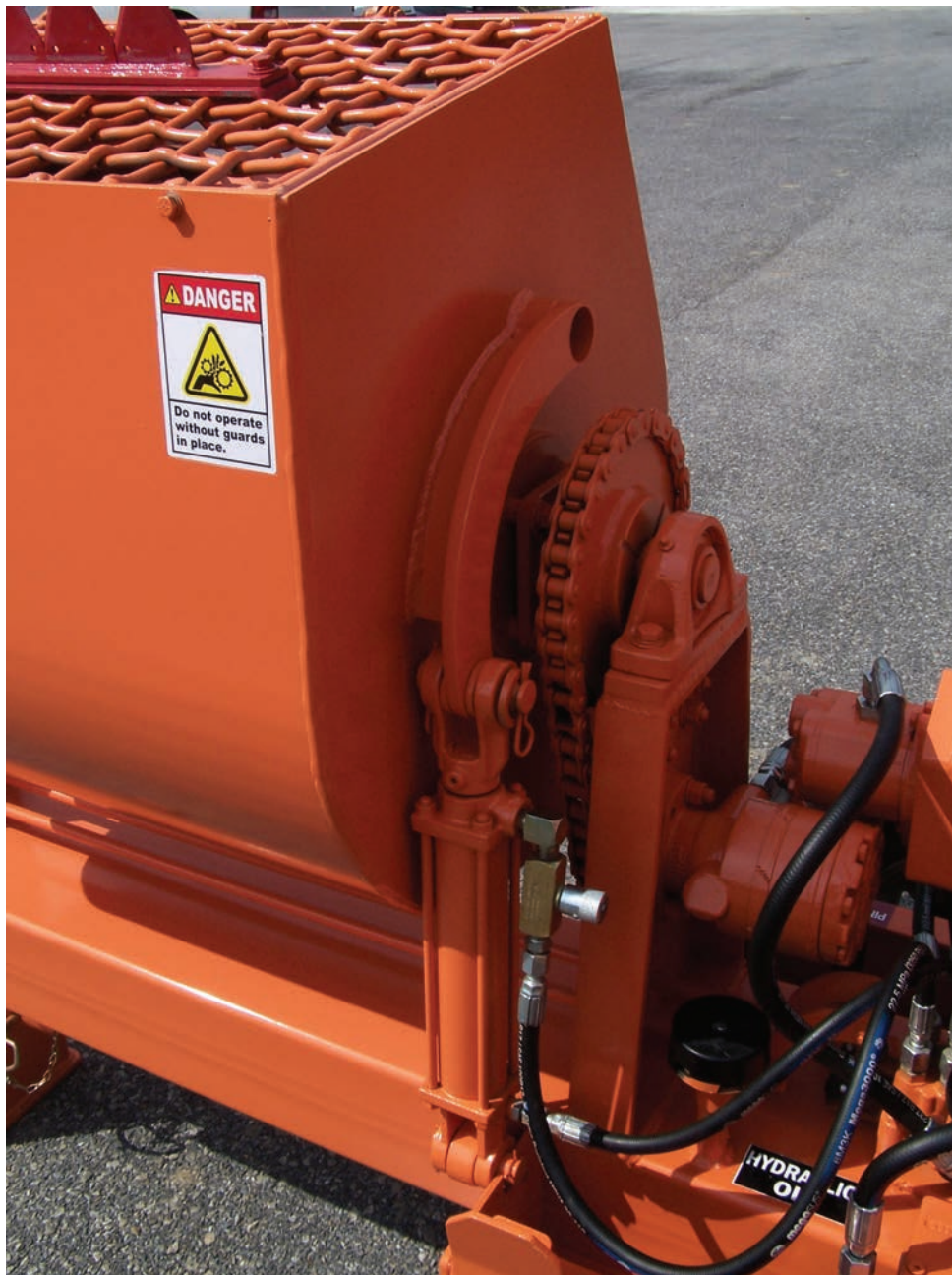
The refractory paddle mixer uses an oversized, heavy-duty, chain-and-sprocket drive system to provide years of reliable use.
