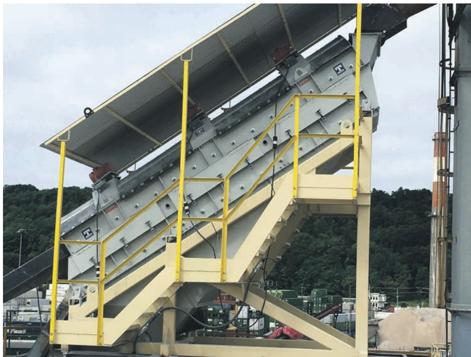
The package includes the heavy-duty welded bridge, A/C drives, controls and optional rubber dust covers for hot or cold applications.
