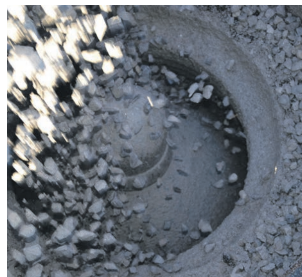
Schmidt recommended keeping the feed height into the crusher at a minimum and to be sure it is centered.
