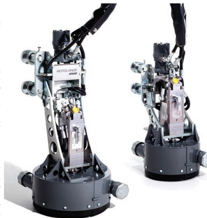
The powerful Rotolance tool, from Aquajet Systems AB, works in conjunction with the Aqua Cutter 710 hydrodemolition robot as well as the Aqua Spine and Aqua Frame to deliver water pressures in excess of 36,000 psi through a specially designed pattern of nozzles.
