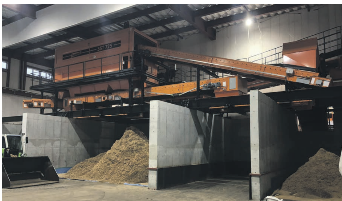
Here a DW 306 Ceron Type B pre shredder, AK 640 VE fine shredding system and SST 725 trommel screen have been combined to provide homogeneous, high quality and metal free material to be used for thermic recycling purposes.
