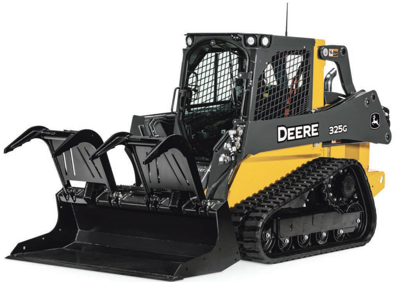
The scrap grapple buckets are ideal for applications where grappling power is needed to handle material.
