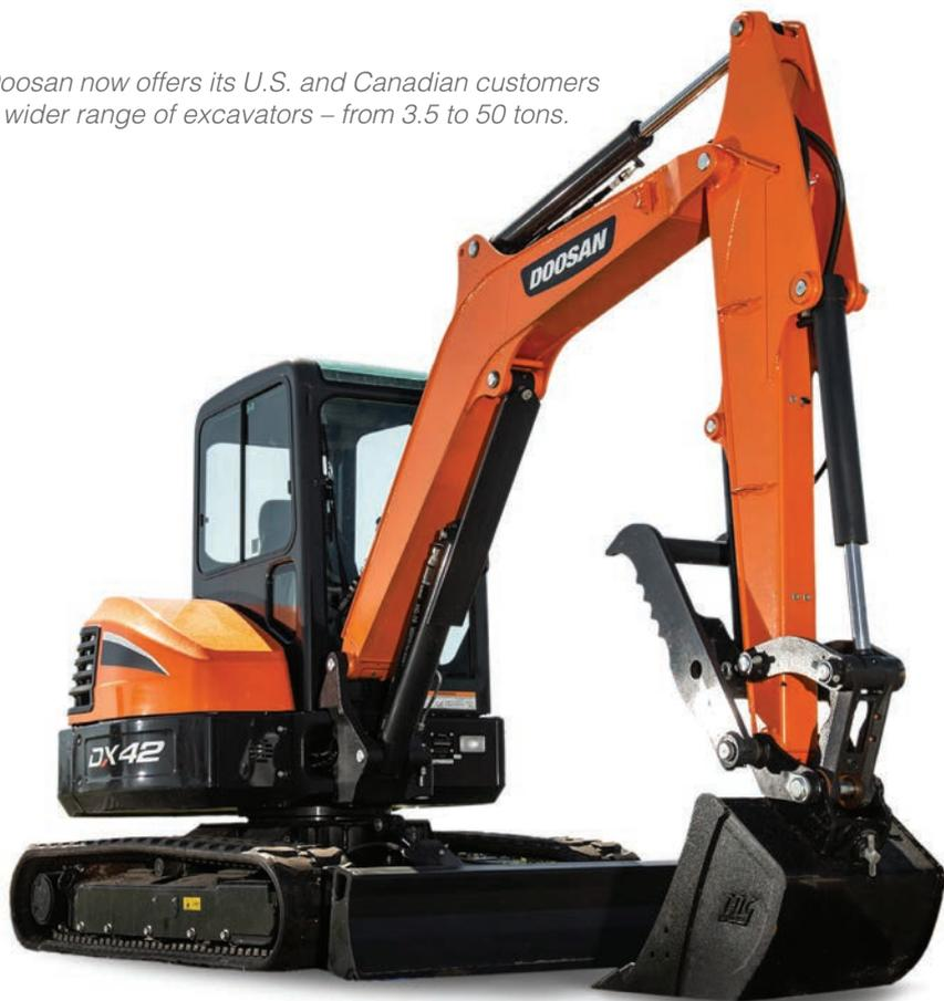
Operators have access to 17 to 20 gallons/minute of auxiliary hydraulic flow, depending on the model, to provide power to other attachments, such as augers, breakers and plate compactors.
