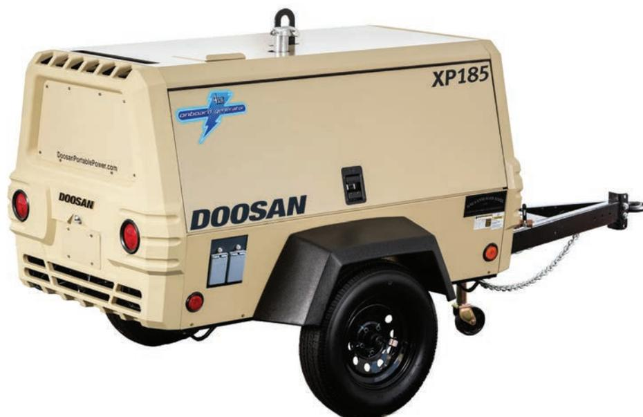
This high-pressure model produces 185 cfm and 125 psi.
