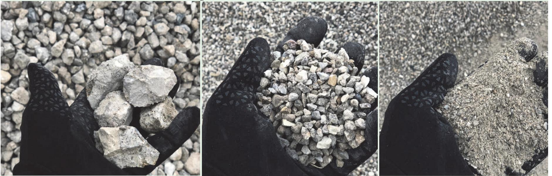
Clean aggregate is produced at site from material that would have traditionally been seen as waste: CA1/CA16 and FA6.
