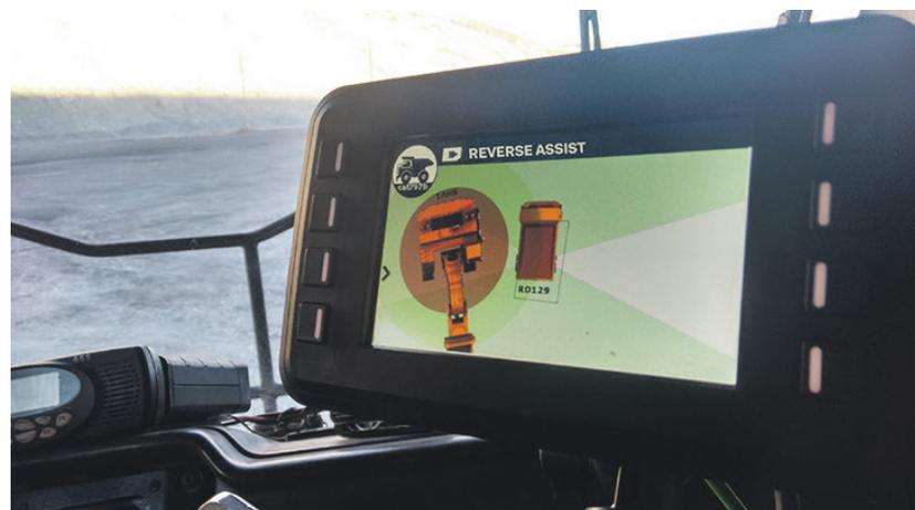
Reverse Assist ensures operators position right the first time, without the need for shovel-bucket support.
