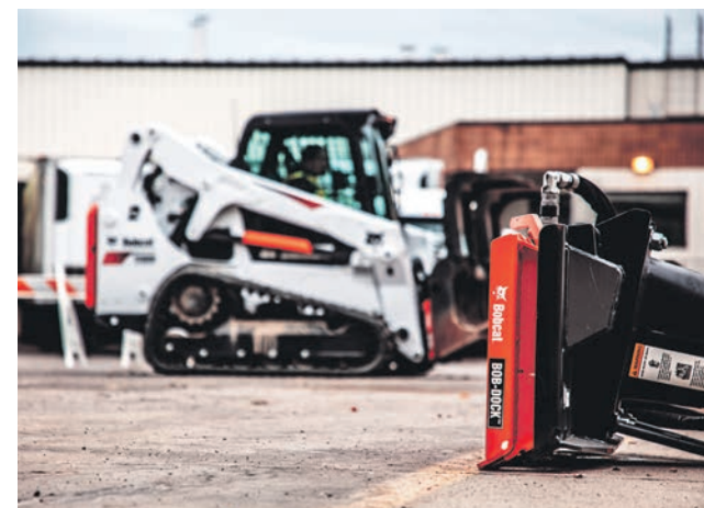
To connect an attachment to a compact loader equipped with the Bob-Dock system, an operator lines up the loader with the attachment's Bob-Dock adapter plate.
