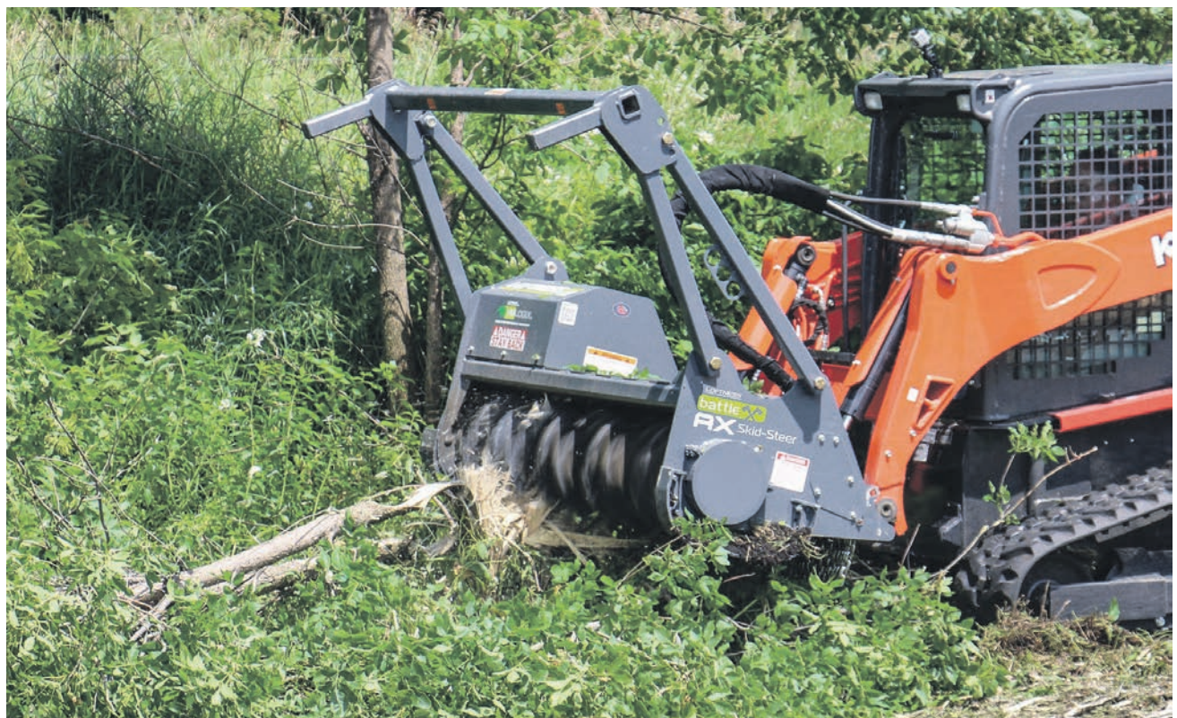
A fixed-displacement gear motor operates at a constant RPM that provides an optimal balance between speed and torque. Photo courtesy of Loftness
