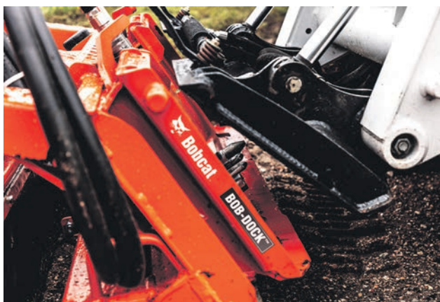
The system prevents many common operator errors, like failing to disconnect hydraulic hoses before backing away from an attachment.
