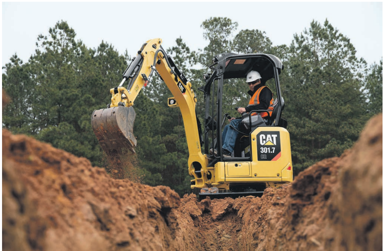
Dig depths are 7 ft, 8 in or 7 ft, 9 in depending on the model, and an available long stick increases depth to 8 ft, 4 in or 8 ft, 5 in.
