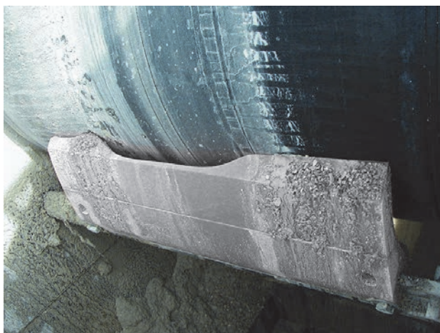
As the center of the blade wears unevenly, the outer edges create a "smiley face" or "mooning" effect.
