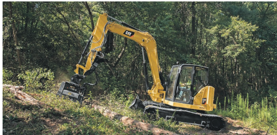
For added versatility, the standard auxiliary hydraulic system (complete with quick-disconnect lines) provides one-way, two-way and continuous flow.
