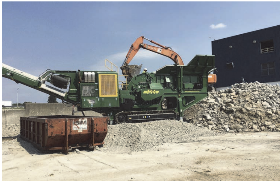
An over band magnetic separator removes rebar and other metal contaminants prior to the crushed concrete being fed into the scalper-screen.
