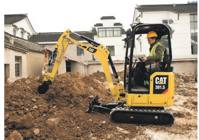
Rubber track undercarriages are standard, with steel tracks available for all models.
