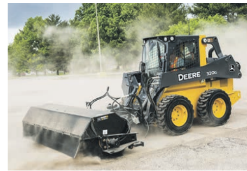
The 32-inch diameter brush features standard 50/50 poly-wire segments, a well-suited combination for dirt and debris cleanup on hard surfaces.
