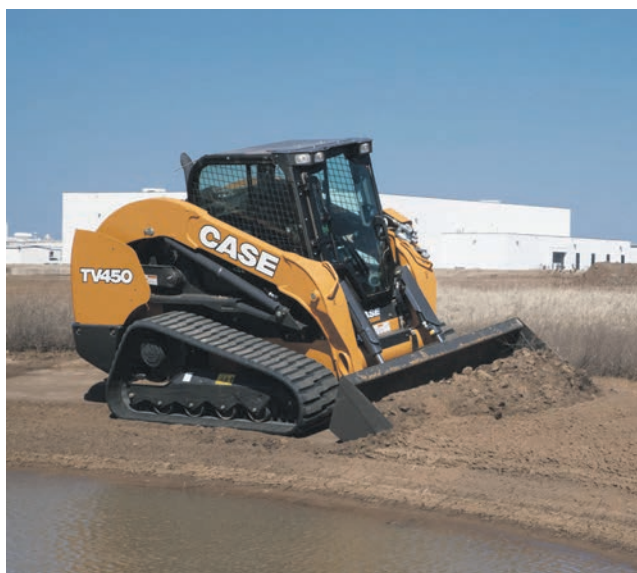
The newest and largest CASE CTL ever built features an industry leading 9,188 pounds of breakout force.
