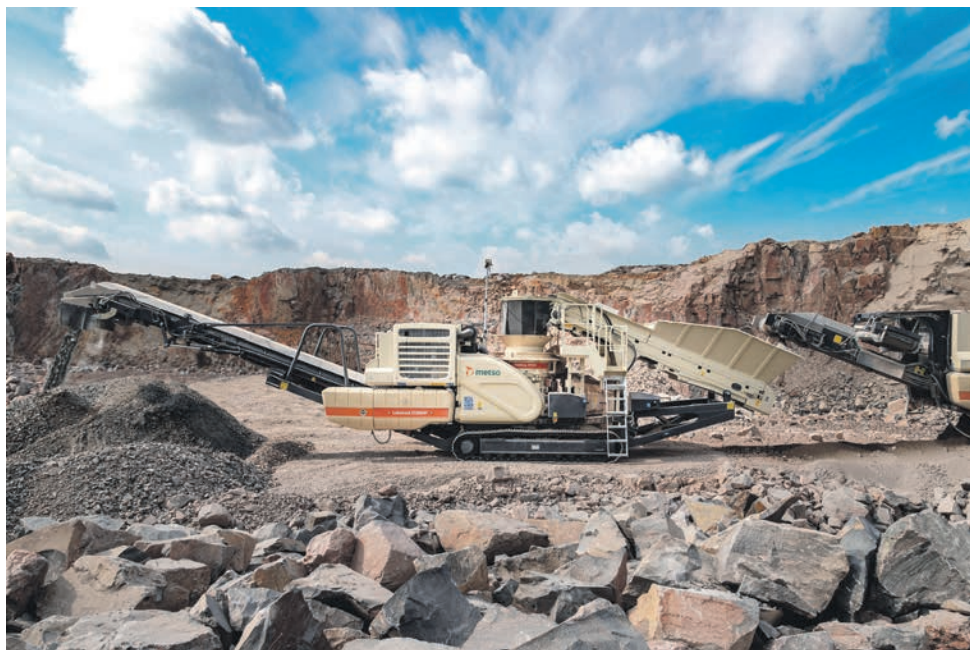
Thanks to its direct V-belt drive from the gearbox, the renewed Lokotrack LT200HP delivers fuel consumption savings of at least 15 percent compared to hydraulically driven cone crushers.
