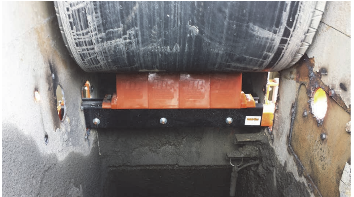
Sixteen additional secondary belt cleaners were attached behind the header, equipped with tungsten tipped blades.
