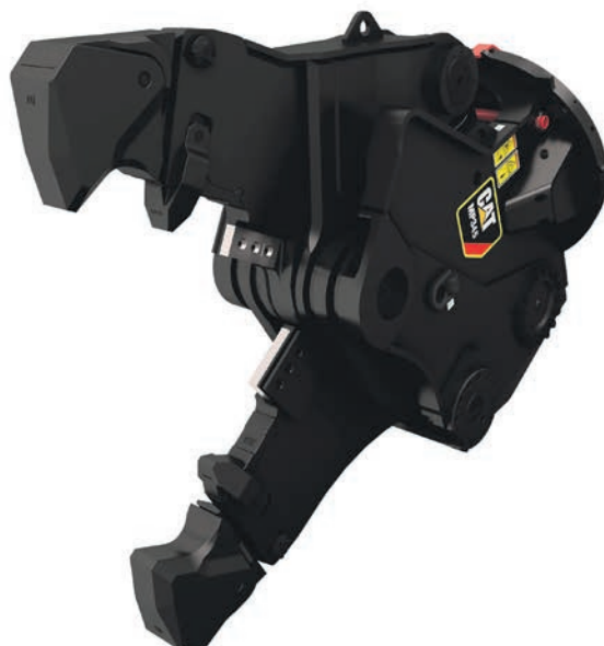
The MP345 with concrete cutter can cut I-beams (17.7 in/450 mm) and H-beams (11.0 in/280 mm).
