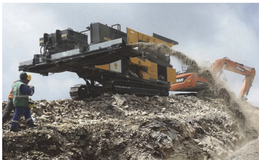
Left: Due to their small size and low weight, many compact crushers are capable of getting to even the most difficult parts of a site.
