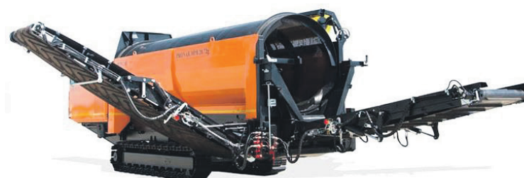
The Model 7.24 GT is a track-mounted or towable trommel screen that has some of the highest throughput in the industry.
