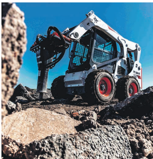
The Bob-Tach system secures the attachment while the Bob-Dock system automatically connects the hydraulics.
