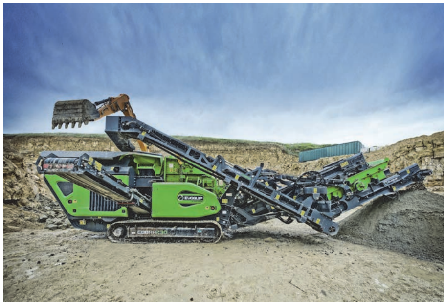
Some compact impact crushers are now equipped with material recirculation equipment.
