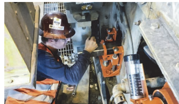
Martin Engineering replaced existing primary cleaners at 16 discharge points, fitting them with low-adhesion urethane blades.
