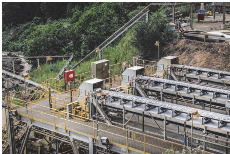
The original conveyor belt cleaners could not manage the overburden, resulting in carryback that caused equipment failures and downtime.
