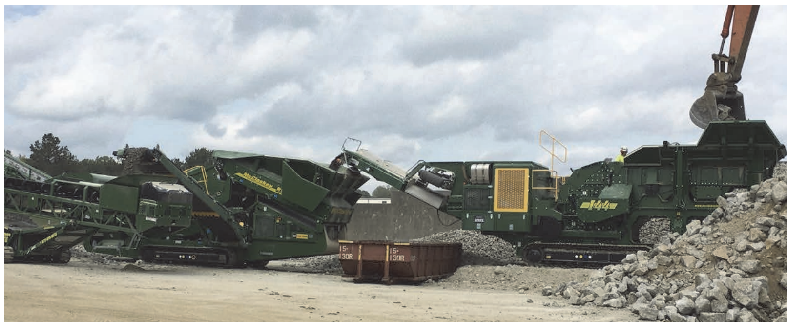
An excavator loads the impact crusher prior to feeding the scalper-screen for further processing.
