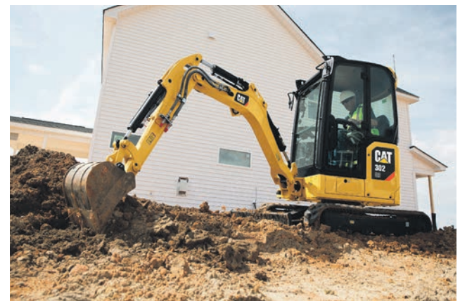
The new Next Generation mini excavators use an efficient, fuel saving, load-sensing hydraulic system with an electronically controlled variable displacement piston pump.
