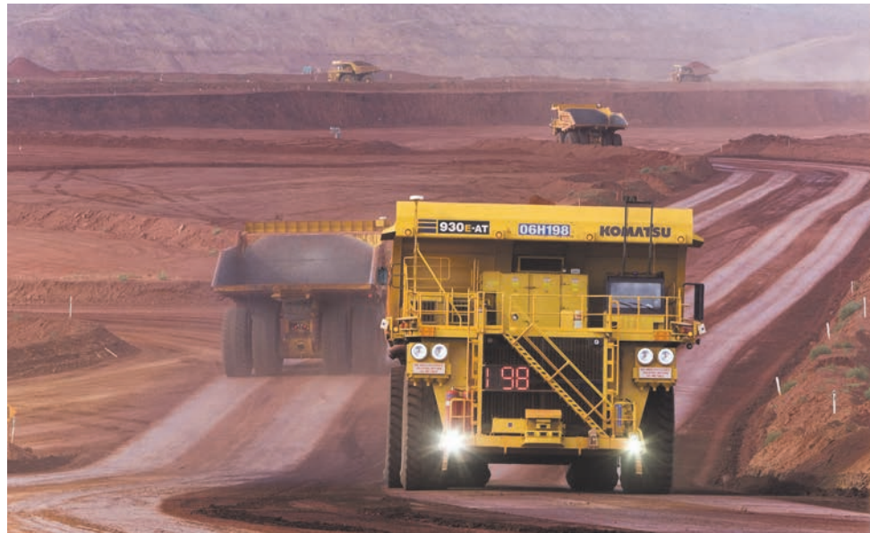
Komatsu's FrontRunner AHS allows unmanned operation of ultra-class mining trucks and is critical to the mining industry.
