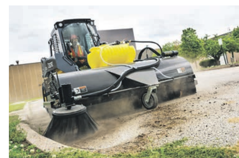
An optional 130-gallon roof-mounted water tank kit is available for applications that require dust suppression.
