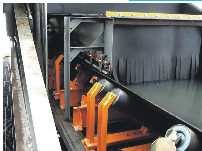
An effective transfer point requires the belt's line of travel to be stabilized and supported.
