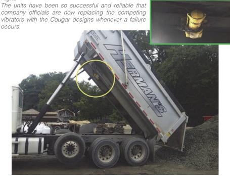
Placed on the upper spine of the truck bed's support frame, the compact unit requires minimal space on Herman's trucks.
