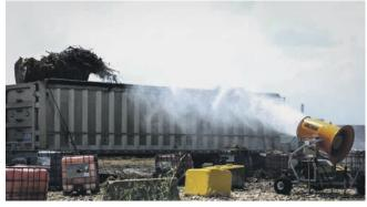
Gavlick's crew positioned the unit to cover the area where yard waste is loaded into trucks for transport to one of the company's composting facilities.
