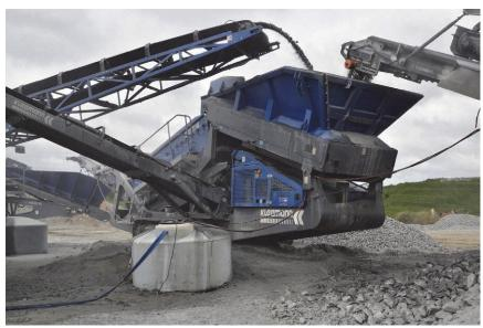
Jaw (right conveyor) and cone crusher (left) send aggregate to the Kleemann Mobiscreen MS 15 Z for further classification.
