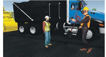
Module scenarios at the paving train help the user to identify and negotiate blind spots, safely navigate around and between equipment and improve communication with workers.
