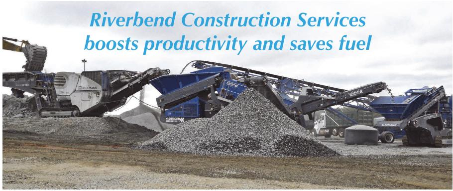
Kleemann Mobicat MC 110 Zi EVO primary jaw crusher, Mobiscreen MS 15 Z screen, and Mobicone MCO 9i EVO secondary cone crusher work together in Interlinked mode.
