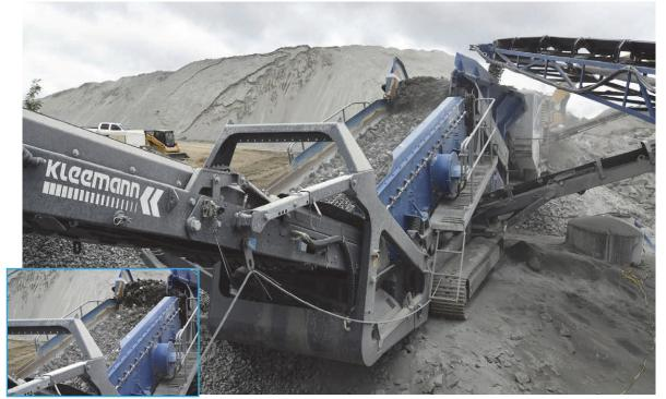
The Kleemann Mobiscreen operates in closed circuit with both the jaw and cone.
