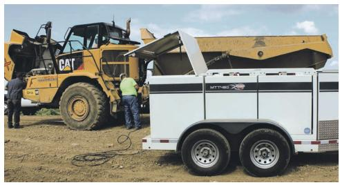
The MTT updates are highlighted by a new electric manifold that automatically shuts off tank valves after fueling to ensure legal transportation and provide protection. Photos courtesy of Thunder Creek
