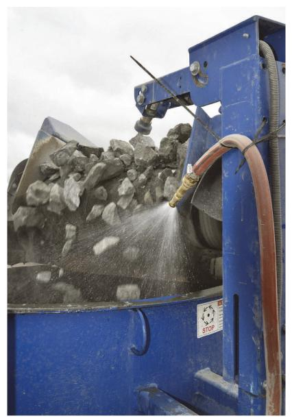
The feed to the cone crusher is subject to the crusher's dust suppression system.
