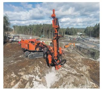
The non-cabin Ranger DXR drill rigs flourish on unstable benches and deep cuts typical to applications such as road and railroad construction.
