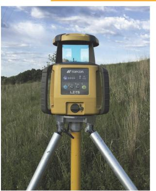
According to Topcon, the product is the world's first GPS-based millimeter accurate control for pavers.
