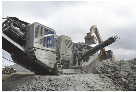
Instead of a grizzly, the new Mobicat primary jaw crusher utilizes an independent prescreen that boosts productivity while reducing wear and tear on system from abrasive fines
