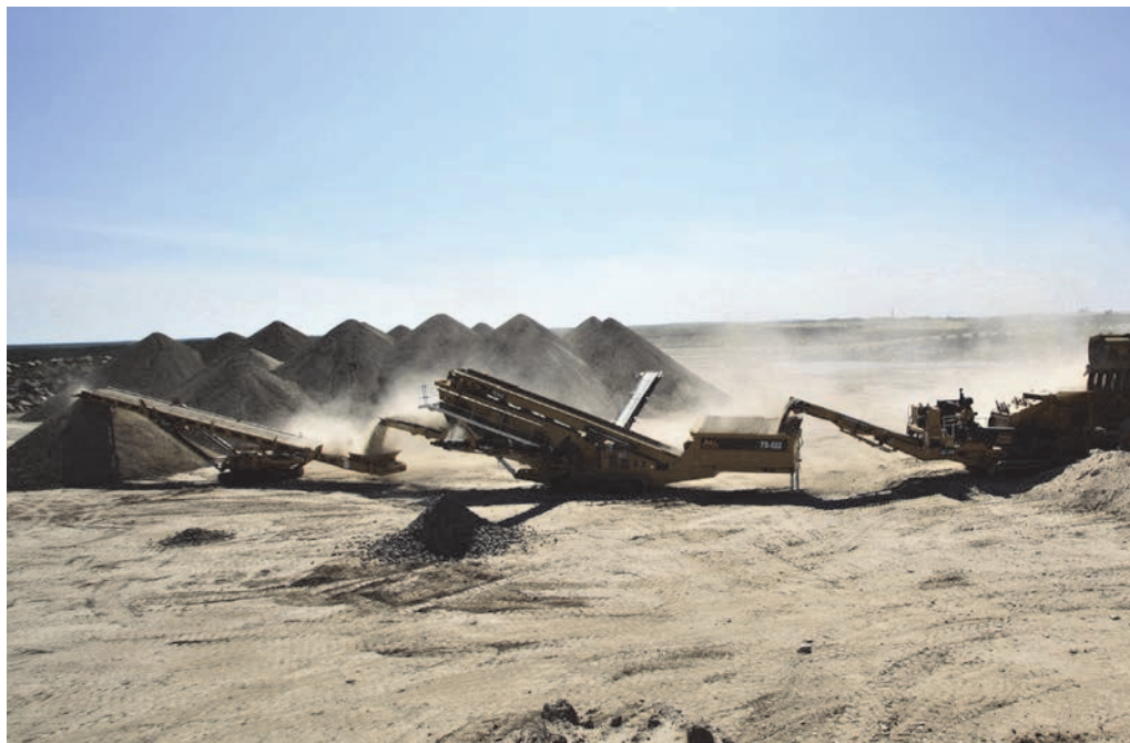
A screening and crushing train using a tracked conveyor as part of the processing unit.
