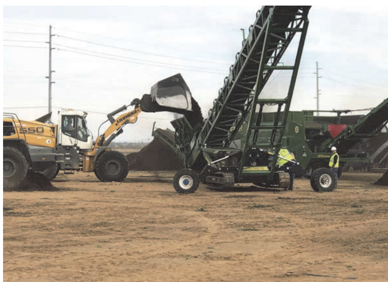
McCloskey's all-terrain stackers combine the benefits of onsite track mobility with the high productivity of a radial conveyor.
