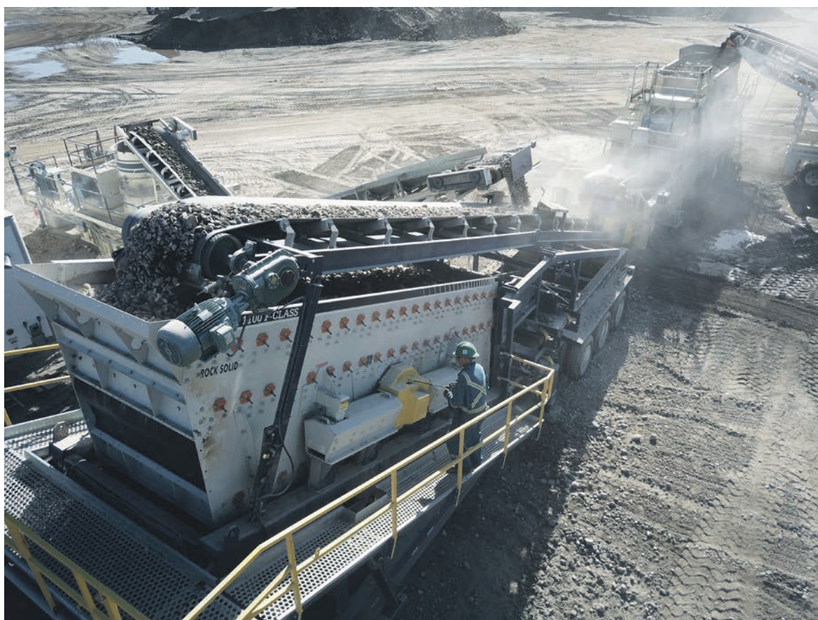
The system reduces water consumption by as much as 75 percent over traditional washing systems, such as log washers and other aggregates washing systems.
