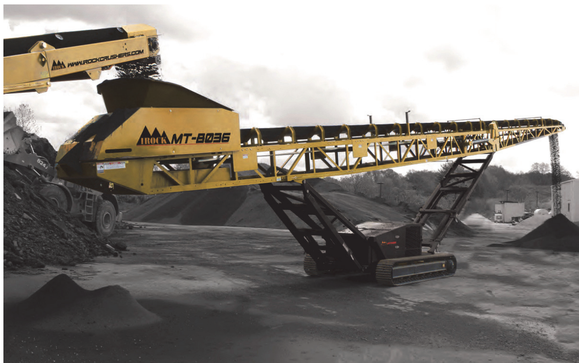
The IROCK MT-8036 possesses heavy duty tracks making the series ideal for demanding terrain or challenging weather conditions.
