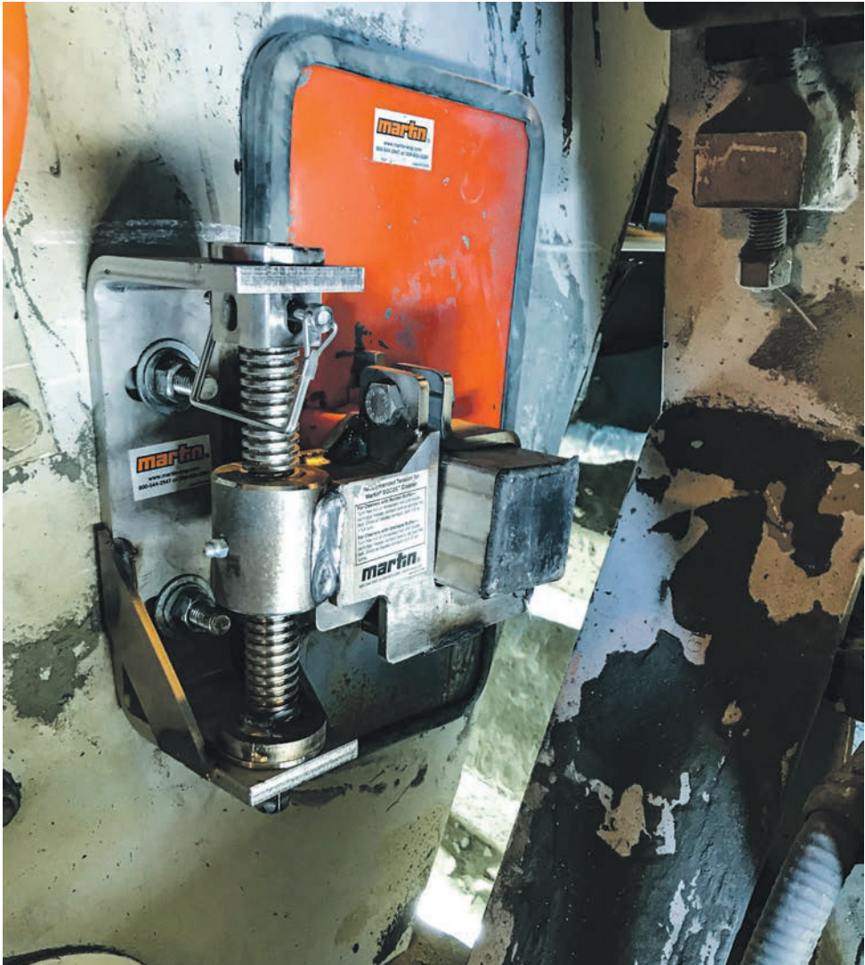
The CS2 typically requires just one re-tensioning during its lifespan, helping to reduce cost of ownership.
