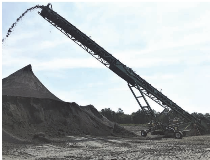
Designed for use in any terrain, the stackers, ranging from 60' to 150', are easily moved site to site.
