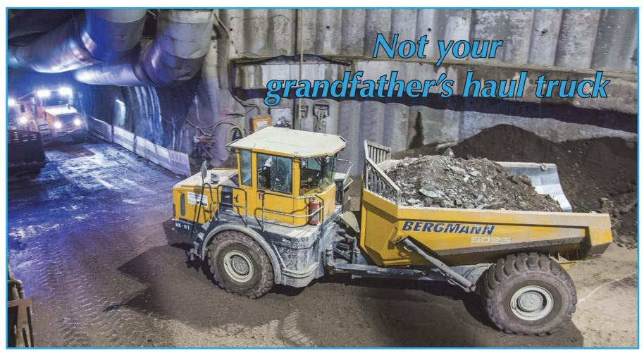
With an empty weight of only 19.25 tons, this articulated 25-ton two-axle vehicle can reach speeds of up to 40 km/h.
