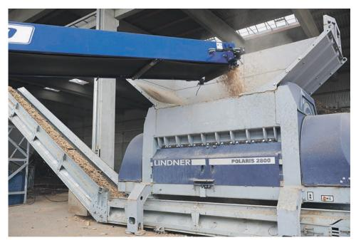
The Lindner Polaris 2800 shredder is designed for continuous operation.
