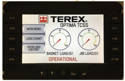
The initial screen on Terex's Load Alert indicates the system is operational.
