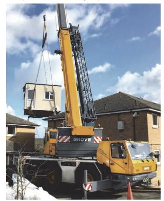
GMK3060L features highly compact dimensions in the three axle segment, enabling it to access tight job sites, maneuver easily around city centers and even work indoors.
