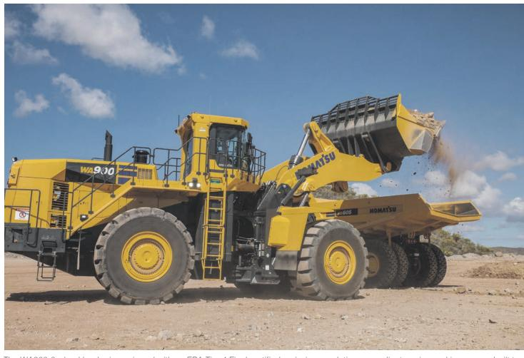
The WA900-8 wheel loader is equipped with an EPA Tier 4 Final certified emission regulations-compliant engine and is purpose-built to load 70- to 150-ton haul trucks.
