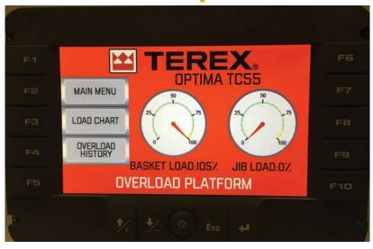
If an overload is detected, the Load Alert screen turns red, displays "overload" and a dial read-out shows the percentage of overload for either the platform or the jib or both.
