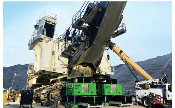
In addition to the JS-500 Jack-up system, Elko also used Enerpac's EVO synchronous lift system under the car body to make small adjustments to the alignment of the center pin going through the center of the machine as they lifted the upper revolving deck.
