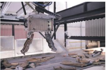
The ZenRobotics ZRR2 Al operates 20 hours/day with total system production of 150,000 tons/year, increasing diversion of recyclables by 20%.
