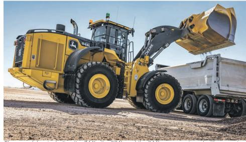
Three models – including the 744L, the 824L and the 844L – are equipped with a roomier cab, new electrohydraulic (EH) controls and an improved HVAC system.
