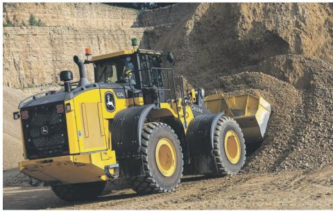
All units boast improvements in fuel efficiency, with the 824L specifically being equipped with a 9.0-L engine.
