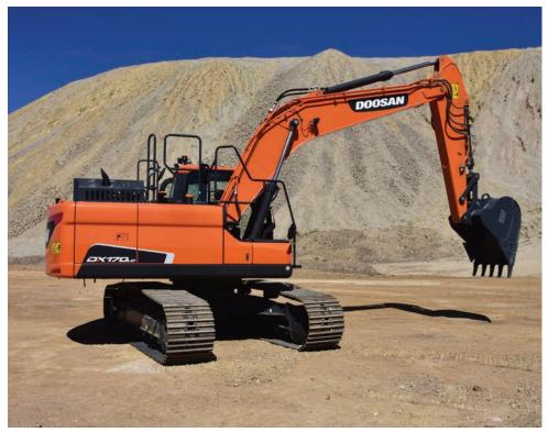
The Doosan DX170LC-5 complies with Tier 4 emission standards with modified diesel engine and aftertreatment technologies.
