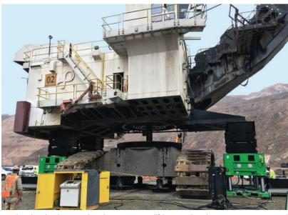
Alignment is checked very closely to ensure lifting under the correct parts and that no damage will take place.
