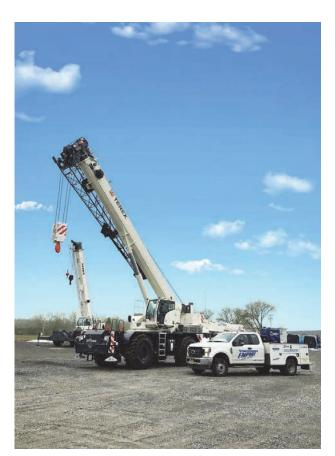
The RT 100 rough terrain crane offers a five section, fully hydraulic boom that extends up to 154 ft (47m).
