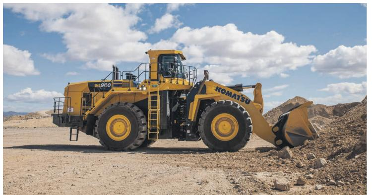
A variable traction control system and modulation clutch system provide optimal tractive effort for various ground conditions.
