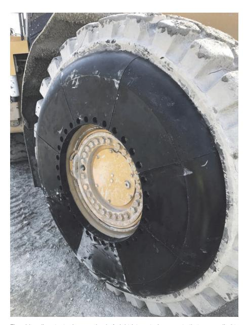
The sidewall protector is comprised of eight integrated segments that are applied to the wheel.
