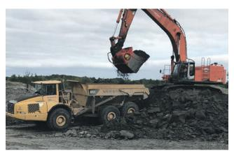
The company purchased the mine-duty M-Series screener-crusher attachment from ALLU to use with its Hitachi 650 excavator in order to crush mined clay down to 4 inch-minus and simultaneously load haul trucks.
