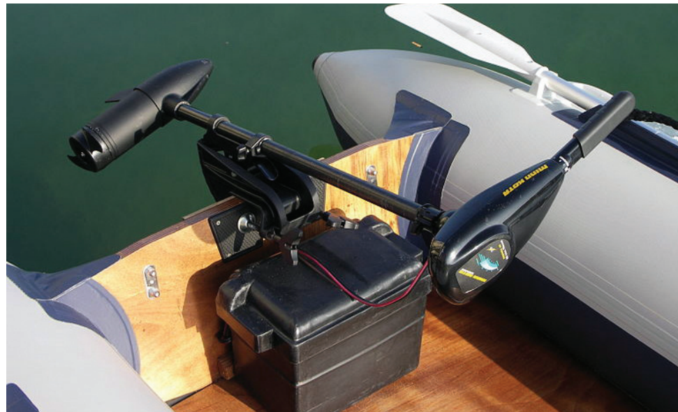
A 12Volt, 30 pound thrust Minn Kota Endura 30 electric trolling outboard motor mounted on a eight foot inflatable.
