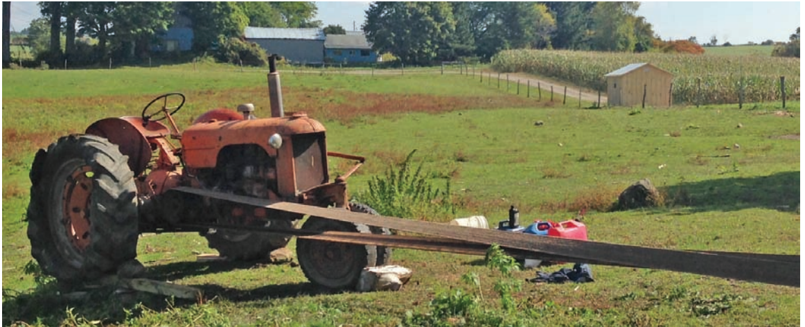
A Case tractor was utilized to power the belt that turned the motor on the machine that blew the corn into the silo.
